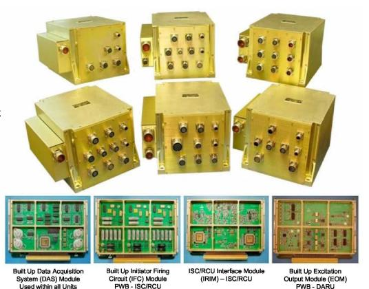
Avionics Box Mock-up LRU 1<sup>st</sup> Generation Engineering Boards
