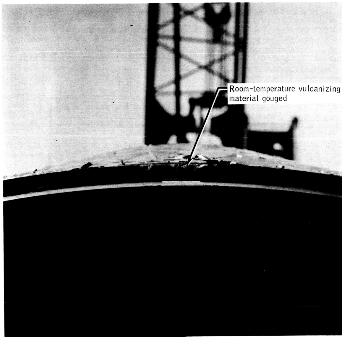
Figure 12.- Forward heat shield damage.
