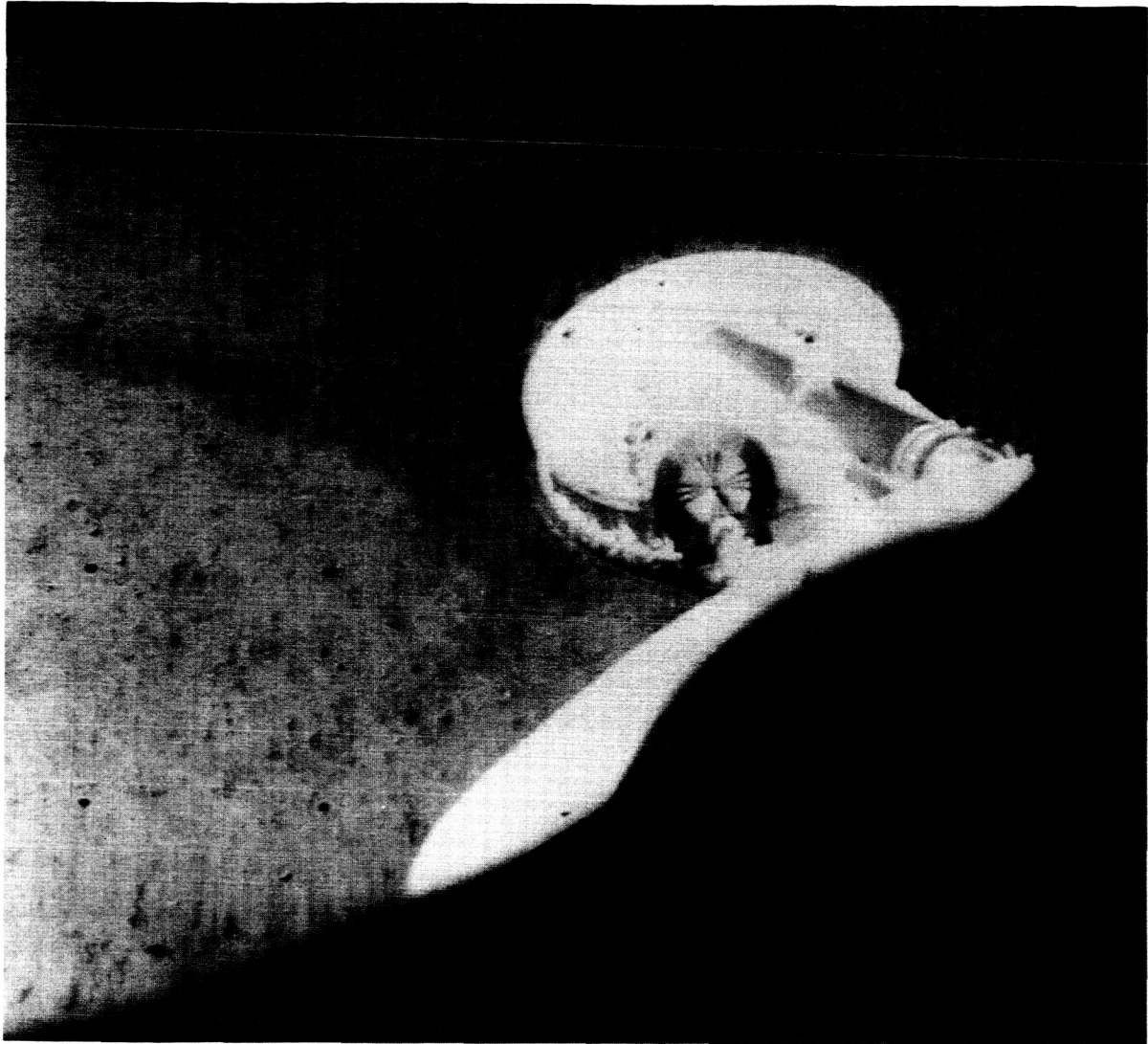
FIGURE 12. — Wide-angle photograph of footpad 2. Note the displaced material that covers the lunar surface beyond the footpad, and the ray extending to the left from the footpad.
