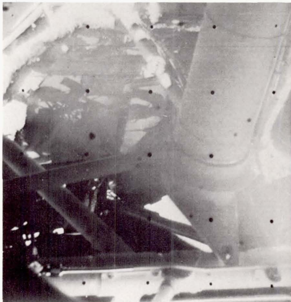
FIGURE 5-23. — Wide-angle view of the auxiliary mirrors on Surveyor III. The shadowed areas under crushable block 3 and the vernier engines are visible in this frame (Day 117, 11:17:45 GMT).
