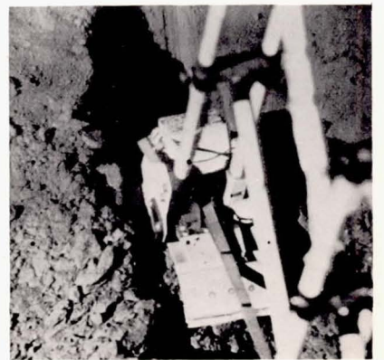
Cover Photo: Narrow-angle photo taken by Surveyor III on the Moon showing fine details of surface sampler digging a trench in the lunar surface. Photo was taken at 17:00:31 GMT, May 1, 1967.
