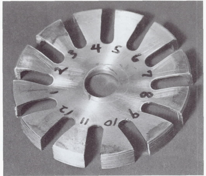
Fig. 2. Selected diaphragm Configuration B. Shown after the testing described in Sec. II
