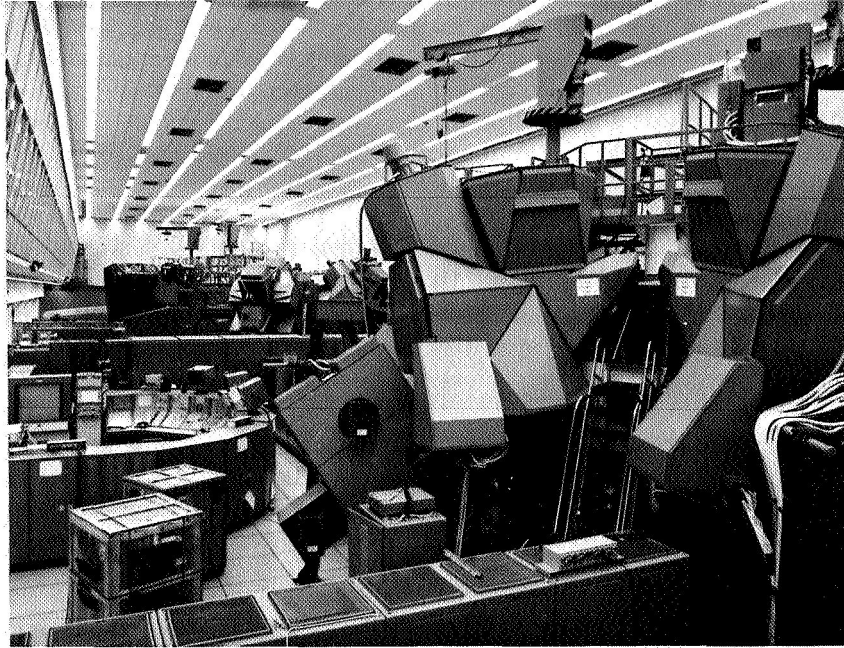
Figure 1-15. Apollo simulator room, KSC. Foreground: Apollo Mission Simulator No. 2; center: Lunar Module Mission Simulator No. 2.
