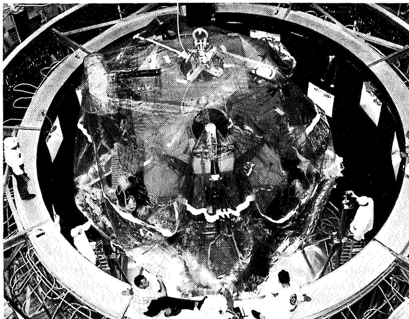
Figure 1-4. LTA-8 being put in space simulation chamber for manned thermovacuum tests.
