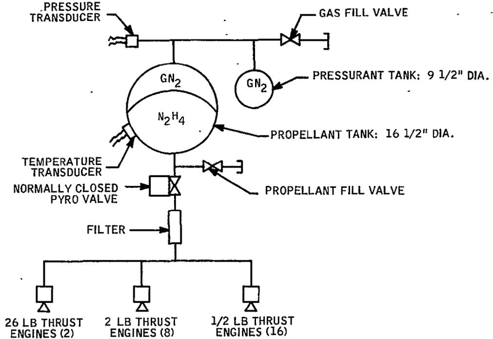
Figure 9.5-5. Propulsion Subsystem Schematic
