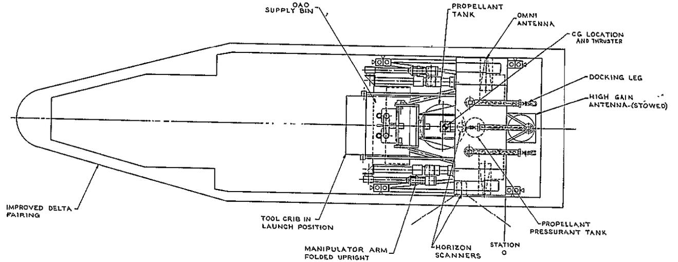
Figure 9.1-6. OAO Repair Configuration
