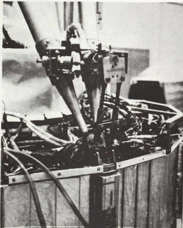
Figure 4-16. Cable Cutter on Paddle Release Mechanism
