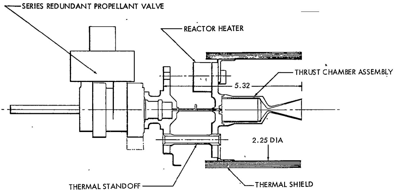
Figure 9.5-3. 1/2-lb Monopropellant Hydrazine Rocket Engine Assembly for Attitude Control and Maneuvering
