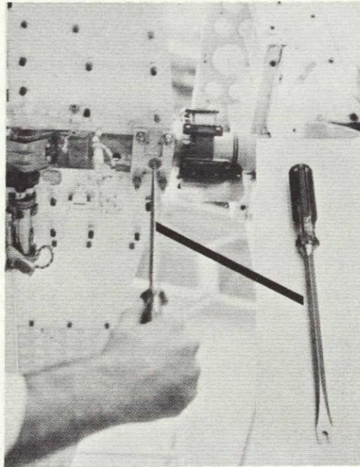
b. Removing Locking Plug-Bottom
