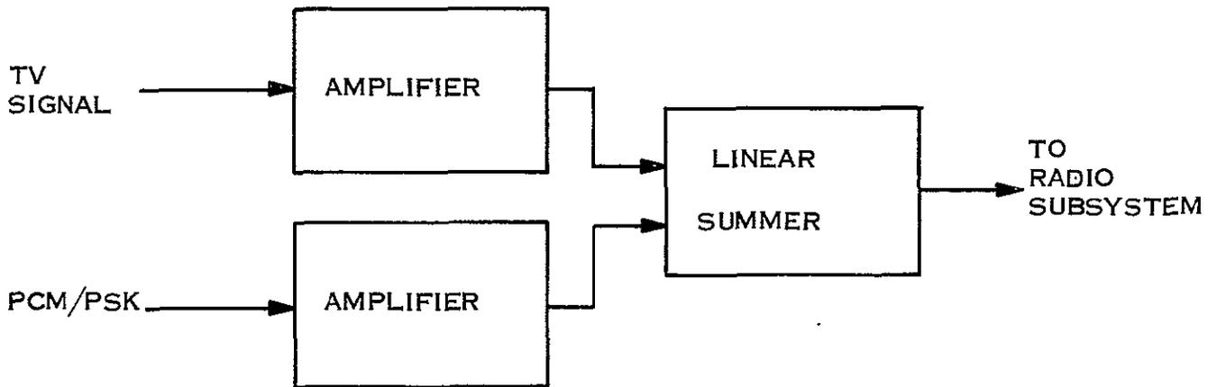
Figure 9.4-9. Baseband Multiplexer Block Diagram
