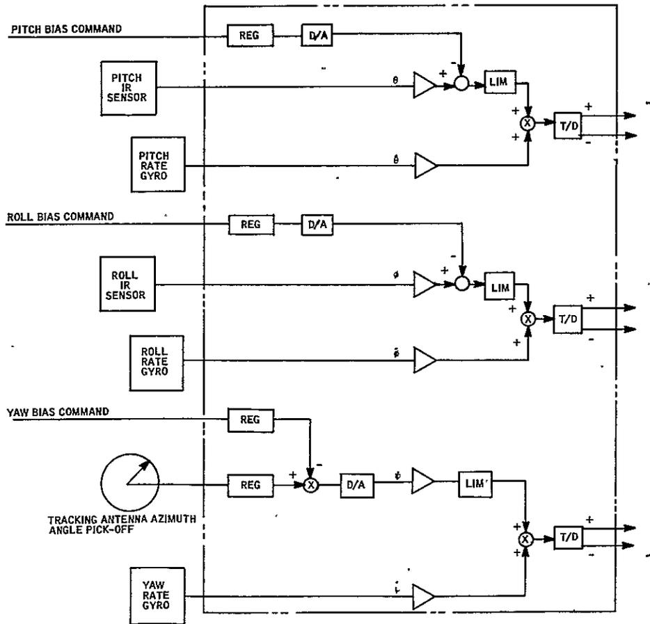
Figure 9.6-4. Attitude Control Reference Subsystem - Fine Sensing Mode
