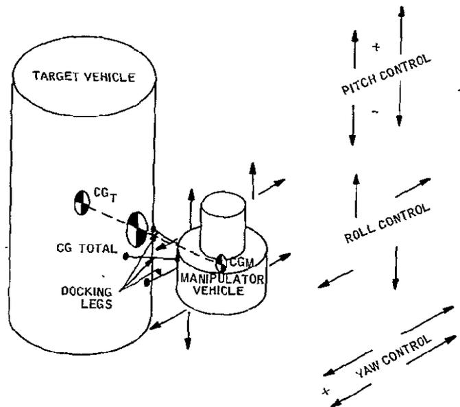
Figure 9.6-2. Thruster Operation for Attitude Control With Offset CG
