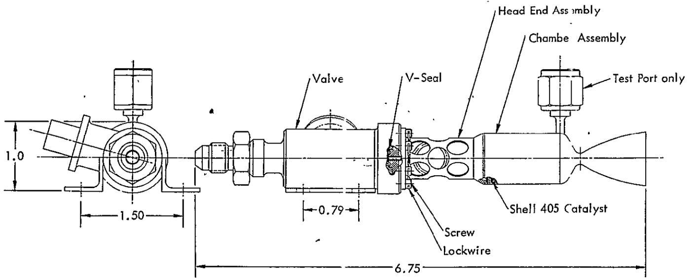
Figure 9.5-2. 2-lb Monopropellant Hydrazine Rocket Engine Assembly for Attitude Control and Maneuvering
