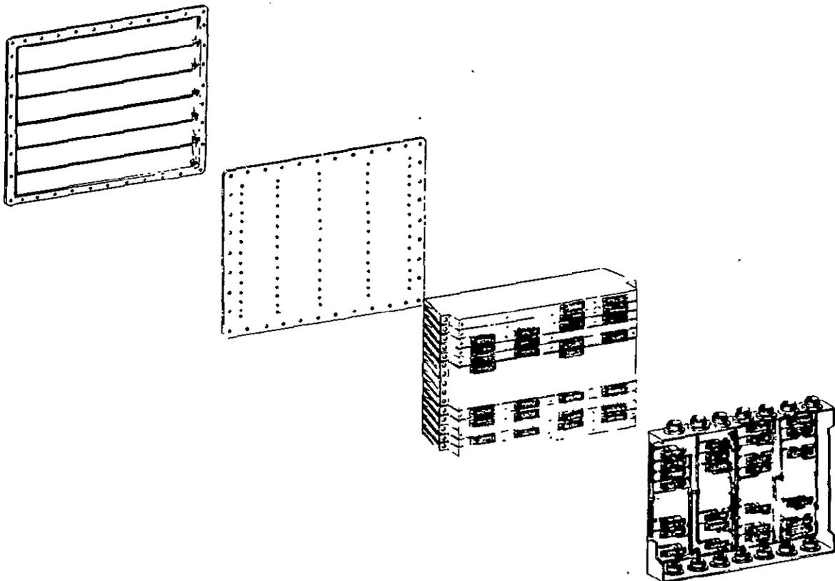
Figure B-10. Electronic Equipment Assembly (Exploded View)
