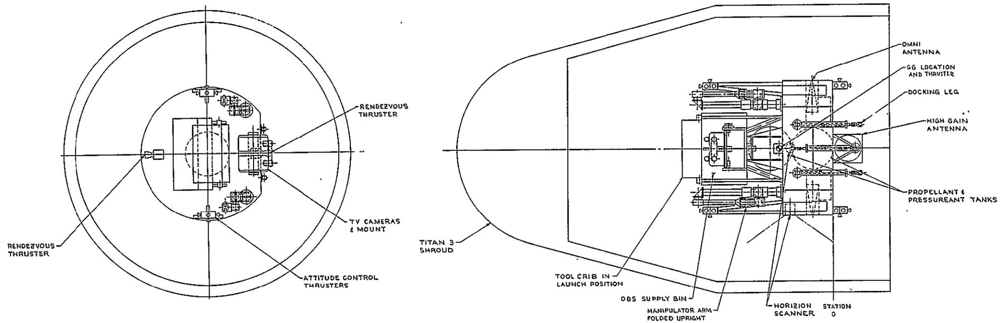
Figure 9.1-7. DBS Repair Configuration
