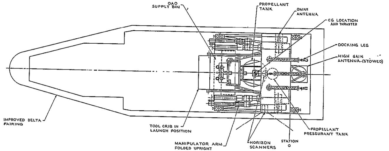
Figure 9.1-6. OAO Repair Configuration
