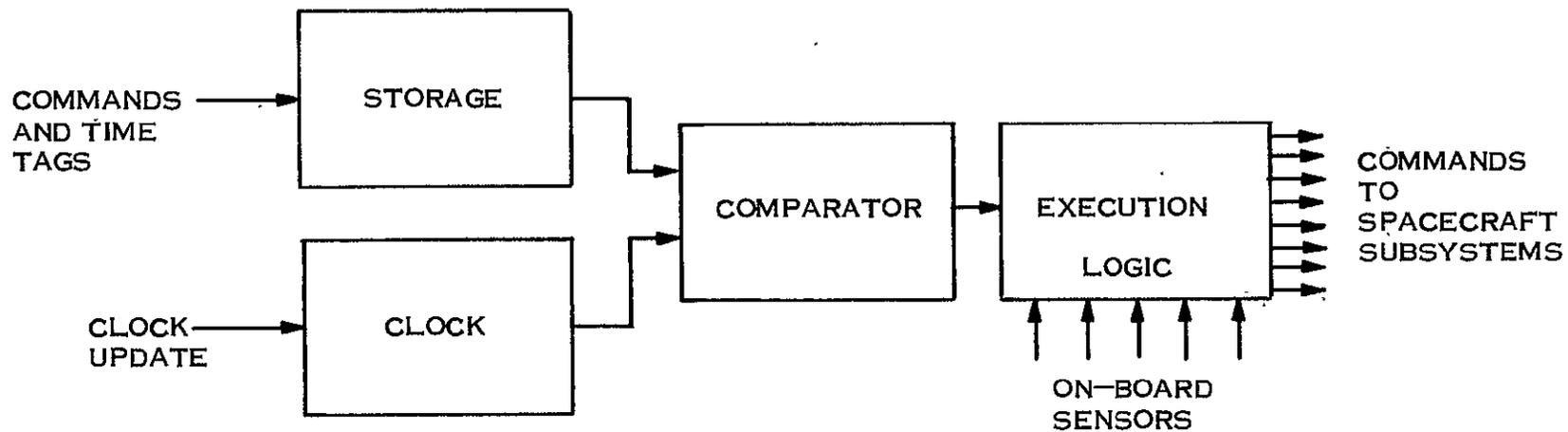
Figure 9.4-7. Command Programmer and Sequencer Block Diagram
