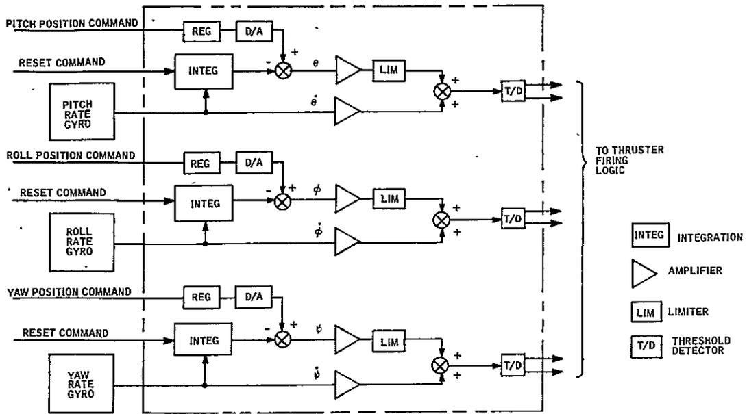
Figure 9.6-3. Attitude Control Reference Subsystem - Inertial Mode
