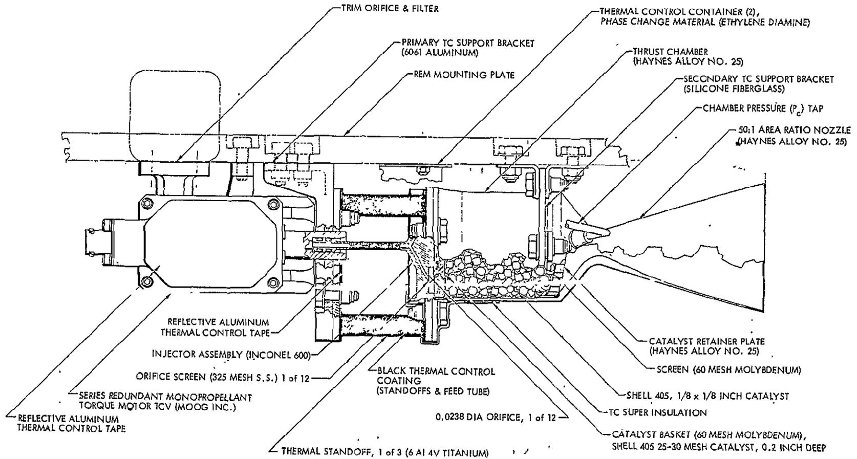
Figure 9.5-1. 26-lb Monopropellant Hydrazine Rocket Engine Assembly for Rendezvous
