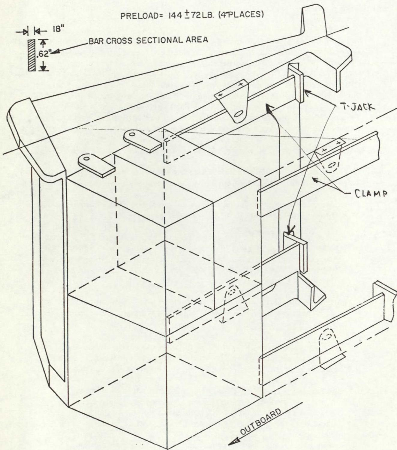
Figure 4-4. Module Preload Arrangement
