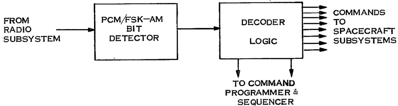
Figure 9.4-6. Satellite Command Decoder Block Diagram
