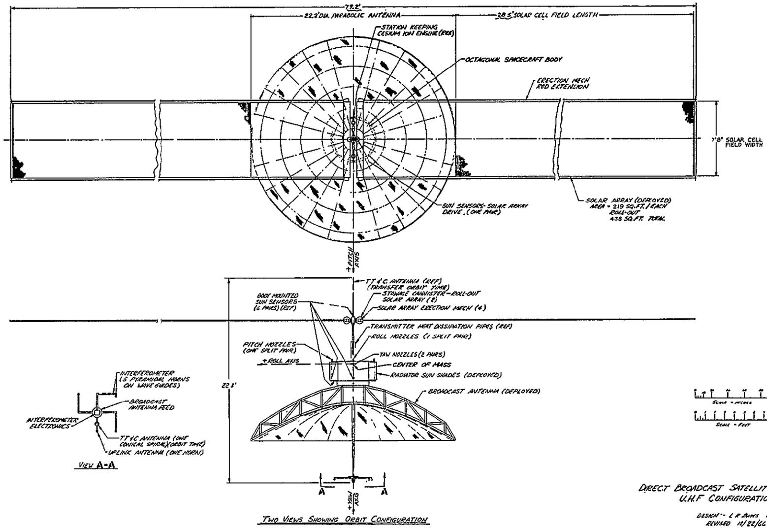
Figure B-7. Direct Broadcast Satellite - Voice Broadcast Mission UHF Configuration
