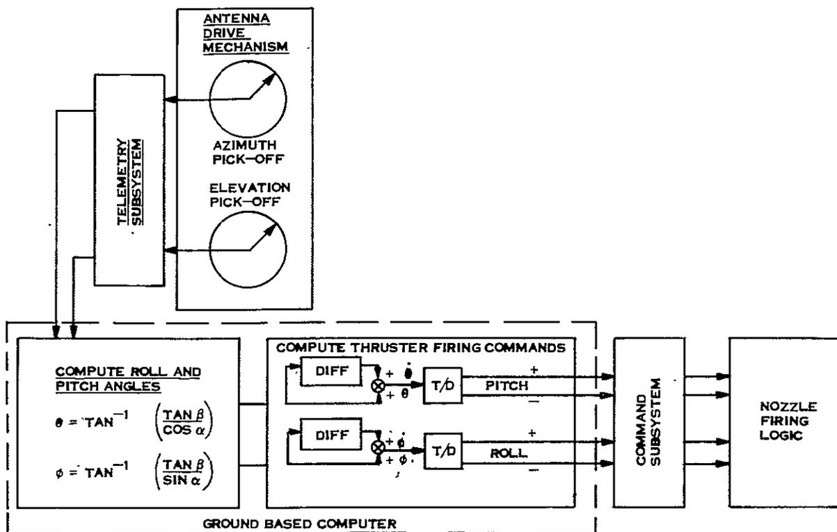
Figure 9.6-5. Attitude Control Subsystem in Coarse Antenna Pointing Mode
