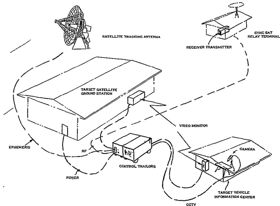
Figure 9.9-2. Ground Station Interfaces
