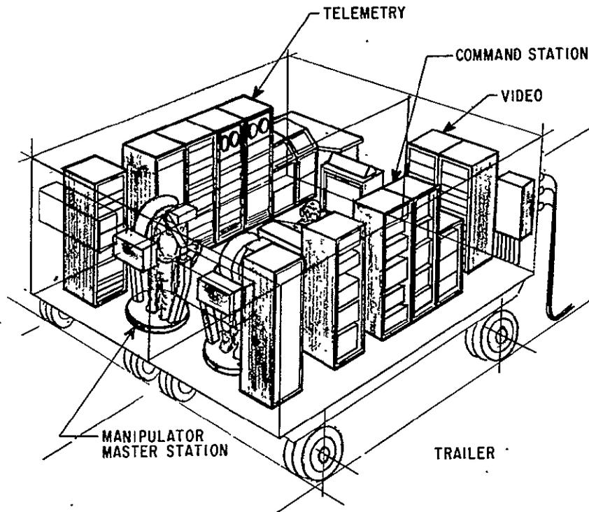
Figure 9.9-1. Ground Station Trailer Design
