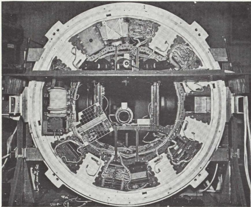
Figure B-16. Nimbus A Component Locations in Sensory Ring - Bottom View
