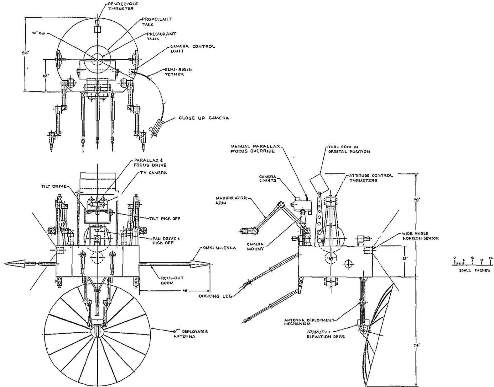
Figure 9.1-3. Basic Manipulator Spacecraft Orbital Configuration
