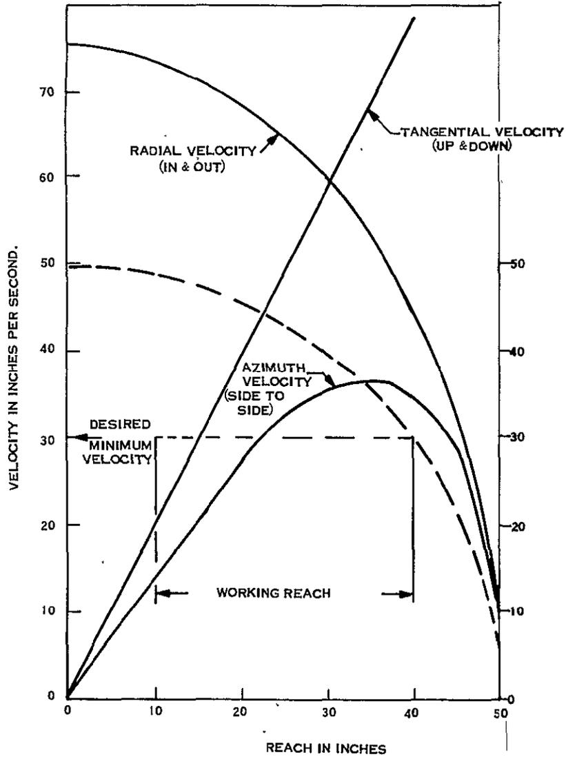
Figure 9.3-4. Velocity Capability versus Reach
