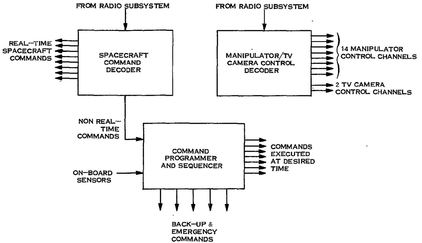
Figure 9. 4-4. Command Subsystem Block Diagram
