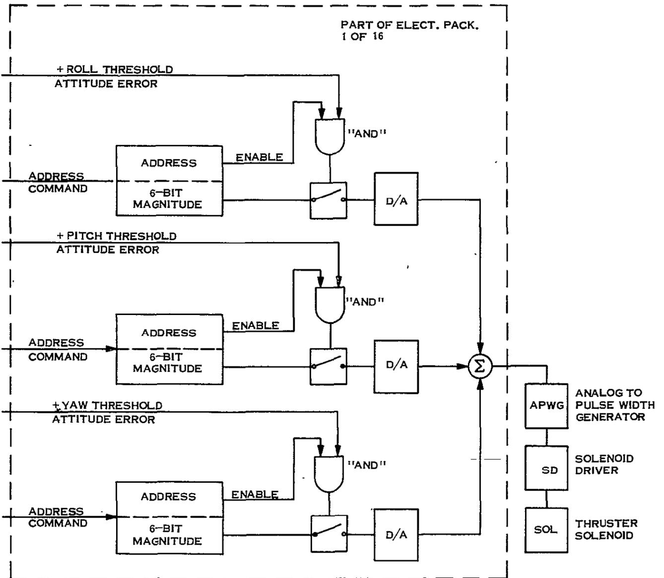
Figure 9.6-6. Thruster Firing Logic for One Thruster Solenoid
