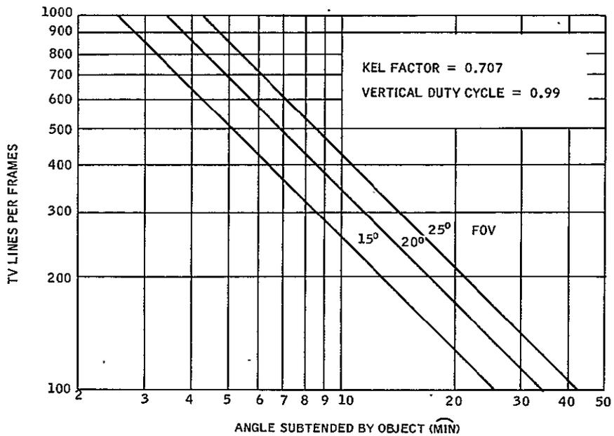
Figure 9.2-3. TVL per Frame versus Angular Resolution
