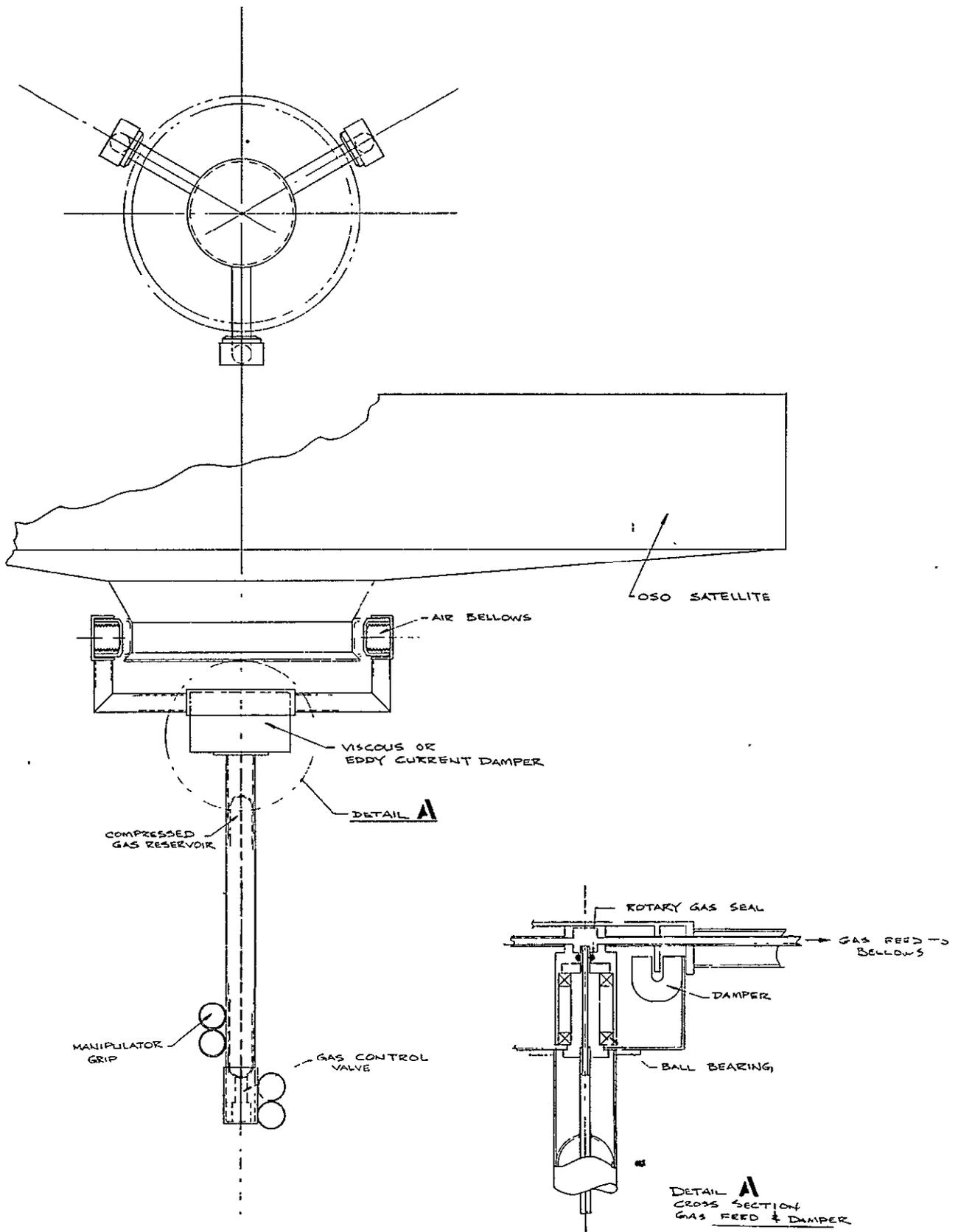
Figure 3-30. OSO-D Fixture Nonrotating Air Bellows Attachment Head
