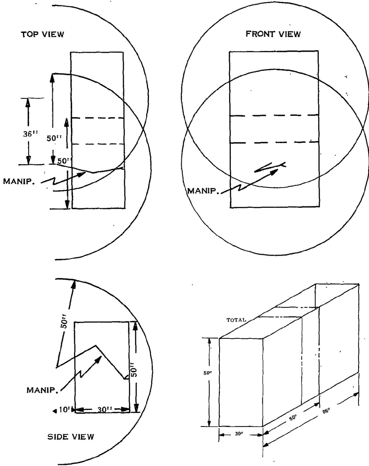
Figure 9.3-3. Total Working Volume for Two Manipulators
