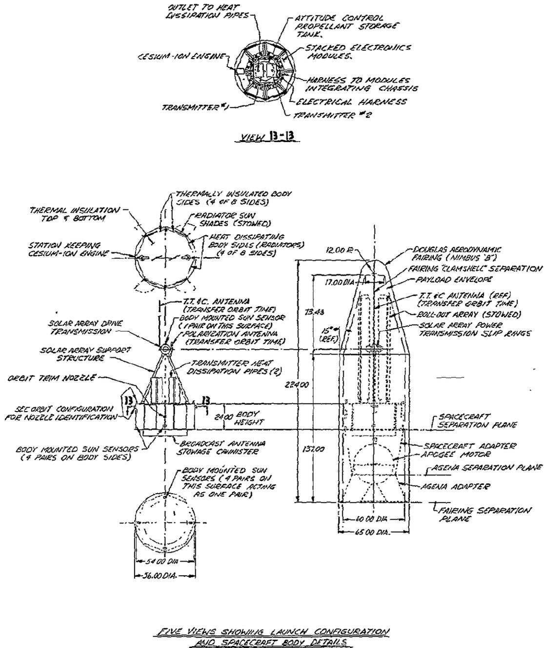
Figure B-6. Launch Configuration of the DBS Satellite
