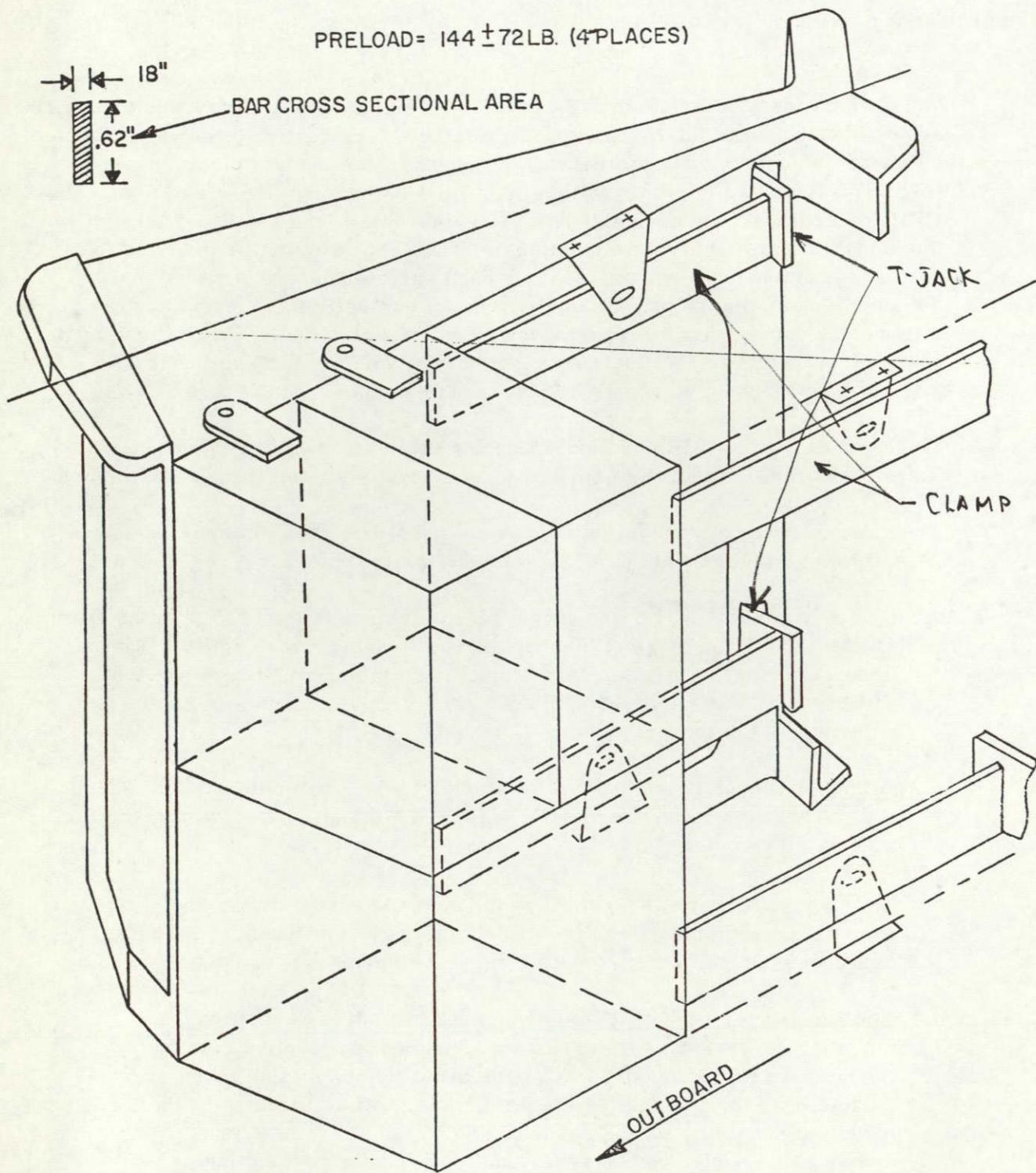
Figure 4-4. Module Preload Arrangement
