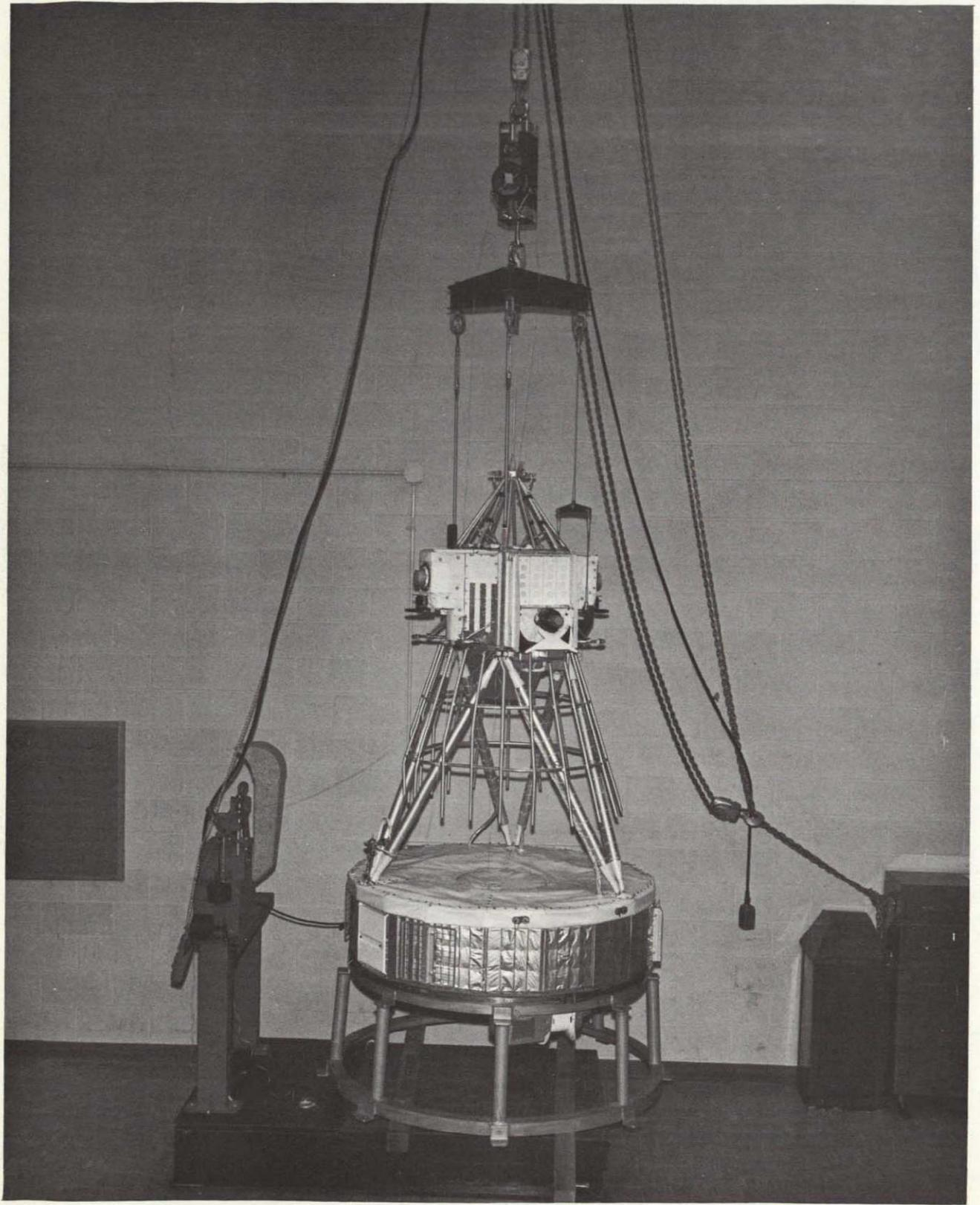
Figure 4-9. Thermal Blanket Attachment
