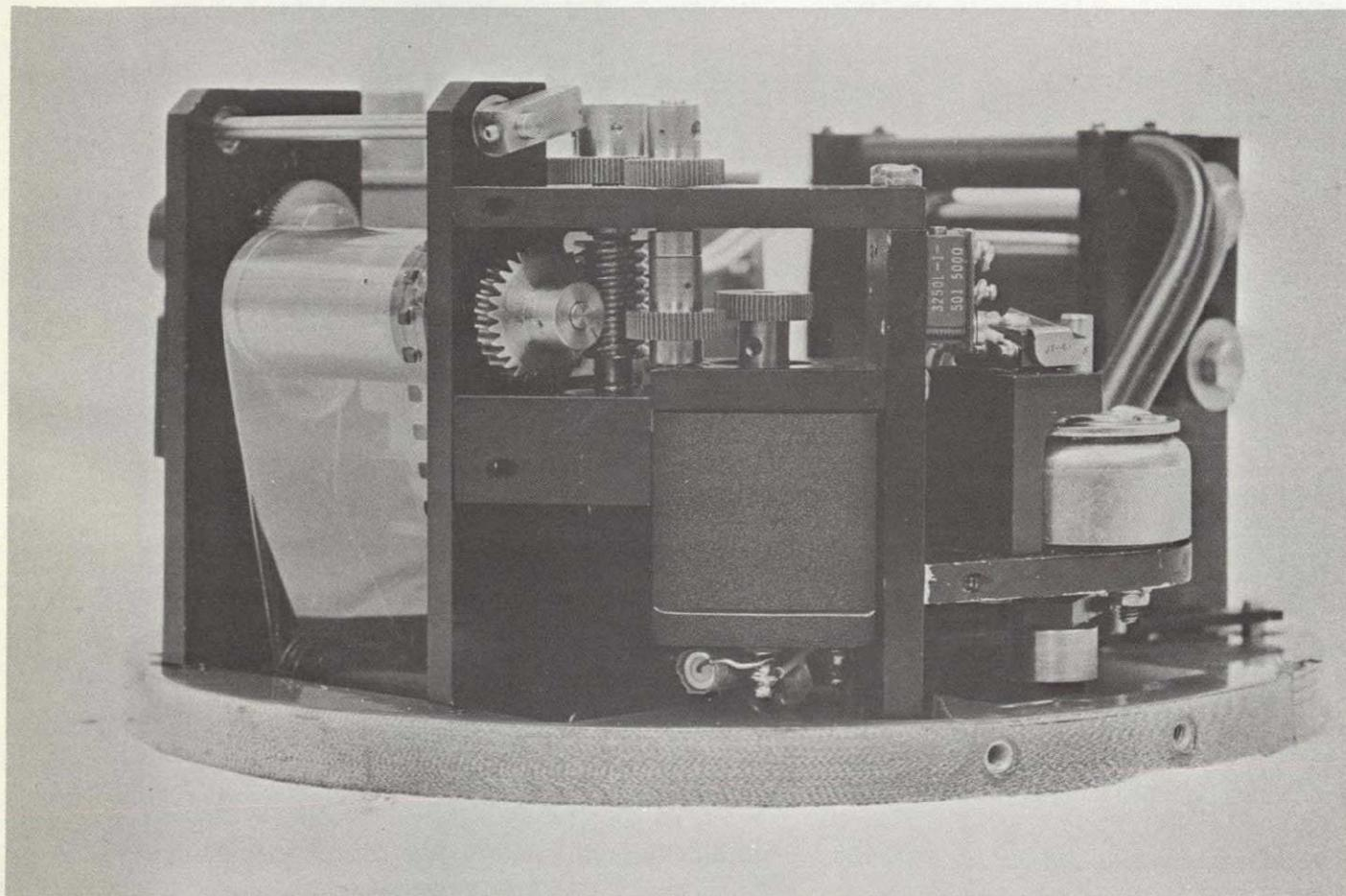
Figure 9.2-5. Automatic Light Control Shutter Assembly
