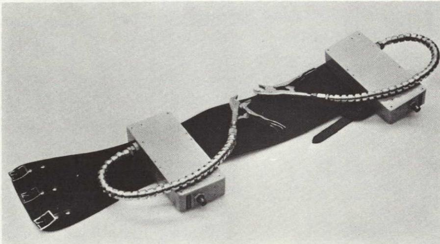
Figure 3-21. Rigidizeable Tether Concept
