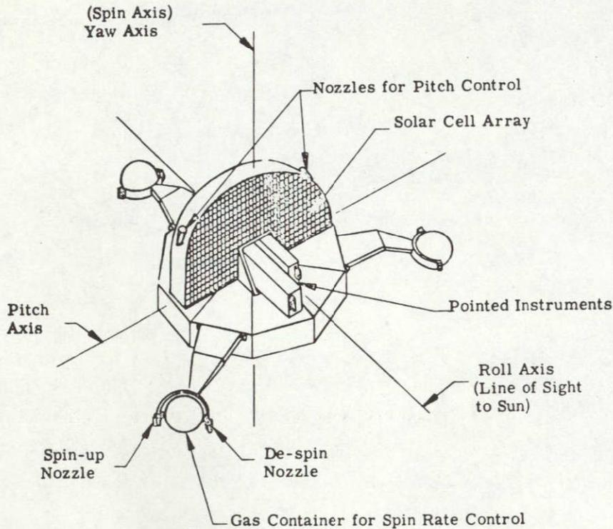
Figure B-5. Orbiting Solar Observatory Physical Characteristics
