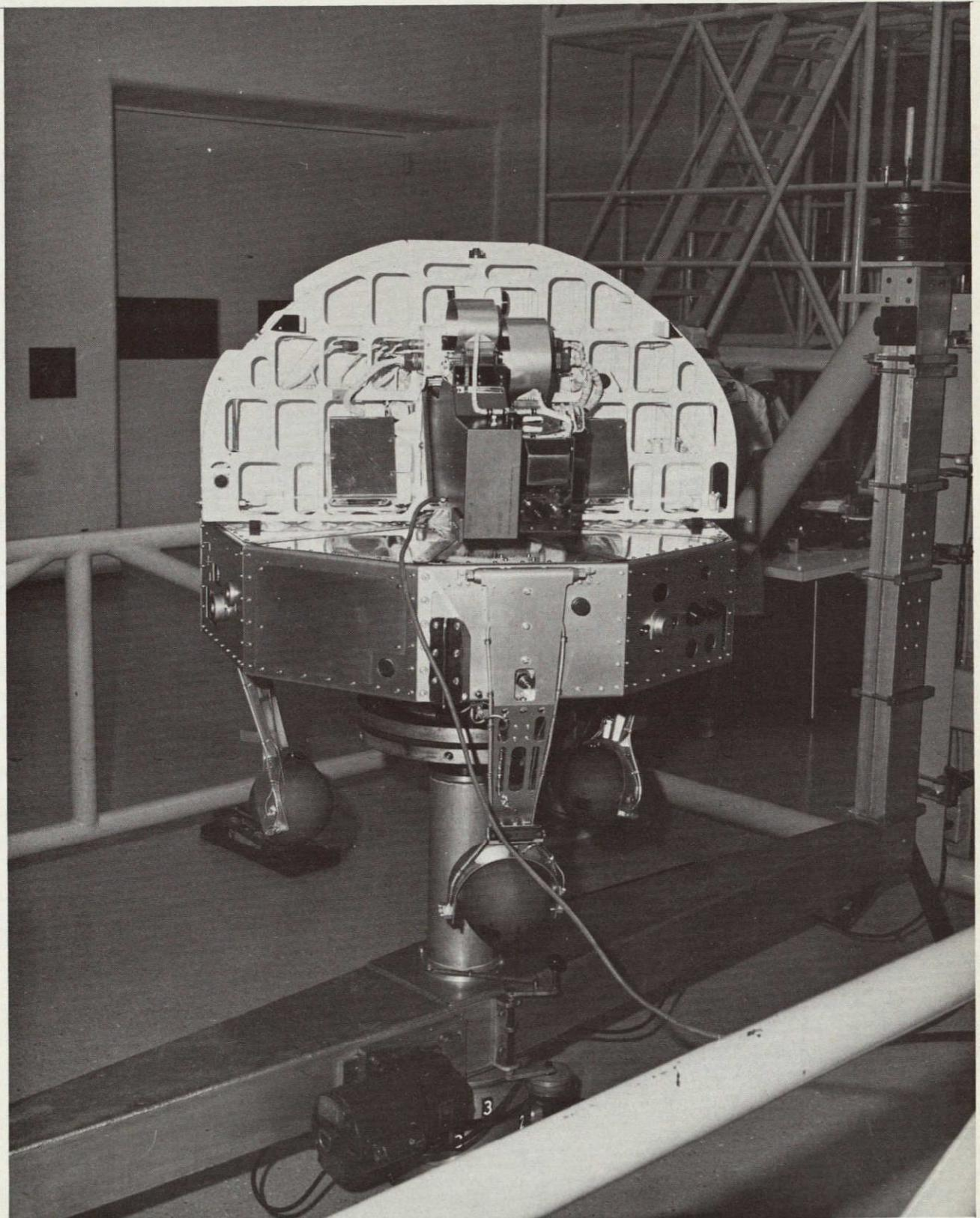
Figure 3-34. OSO-D Showing Compartment Cover Screws and Gas Charge Fitting
