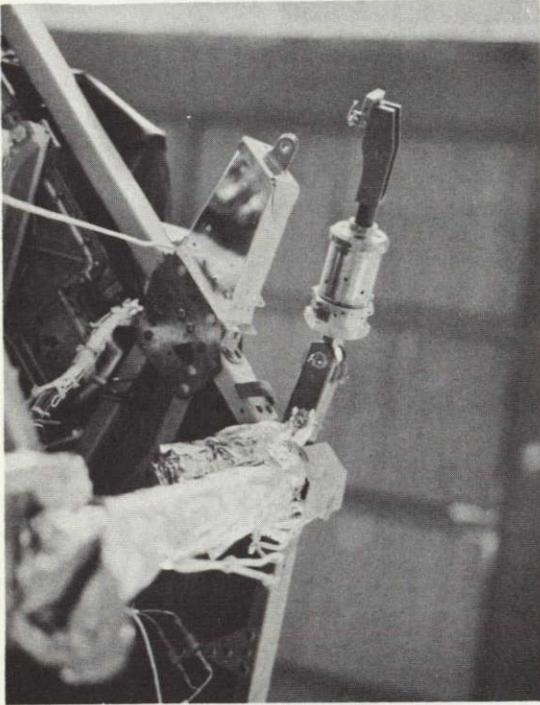
Figure 3 22. Upper Main Paddle Pivot and Damper
