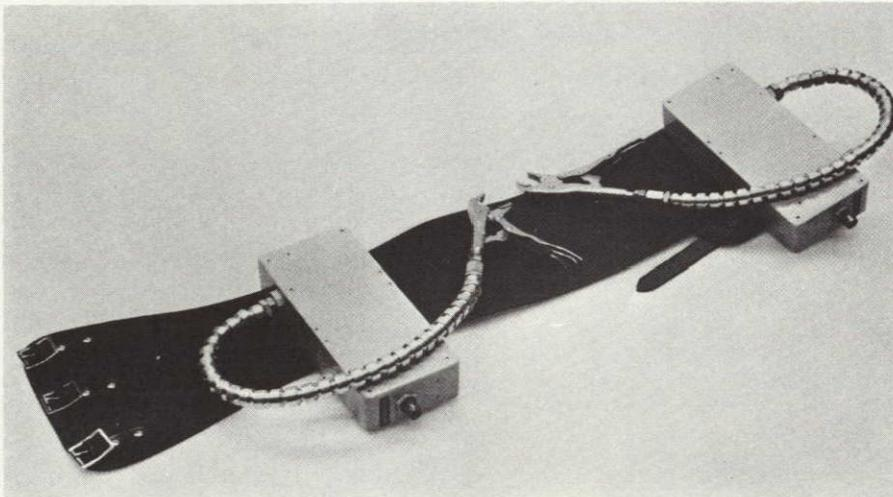
Figure 3-21. Rigidizeable Tether Concept
