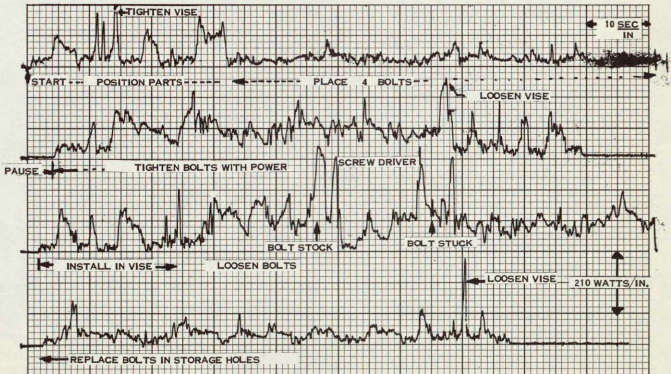
Figure 9.3-8. Power Profile, Assembly and Breakdown of Solenoid Valve
