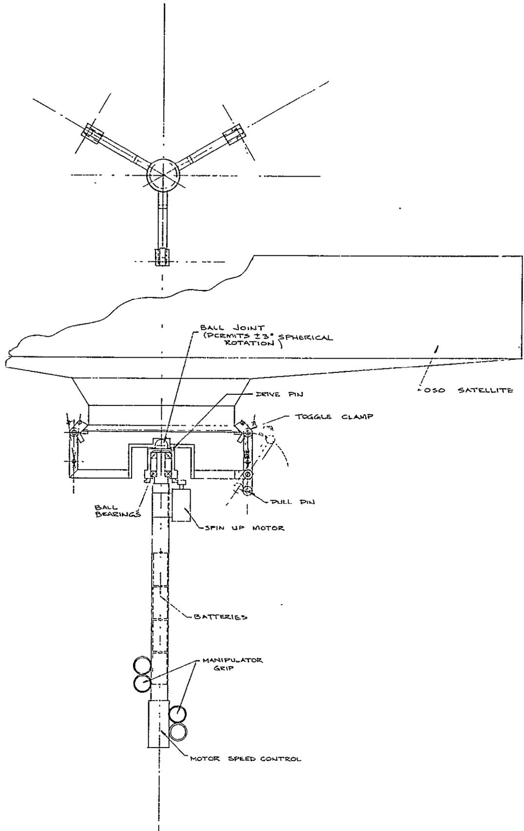
Figure 3-28. OSO-D Despin Fixture Rotating Attachment Head
