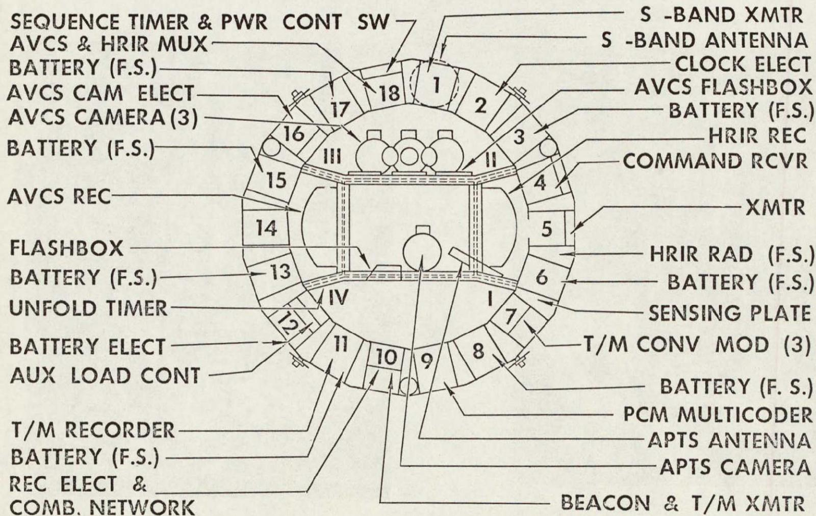
Figure B-15. Nimbus A Component Locations in Sensory Ring - Top View
