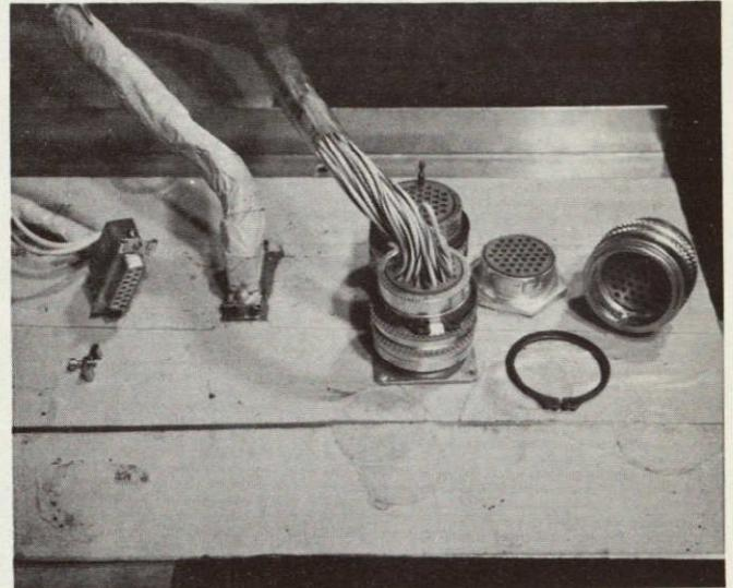
Figure 5-4. Cannon (Left) and Deutsch Electrical Connectors
