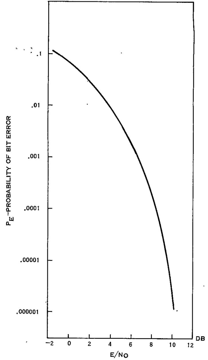
Figure 9.4-14.  $P_e$  versus  $E/N_0$  for PCM/PSK
