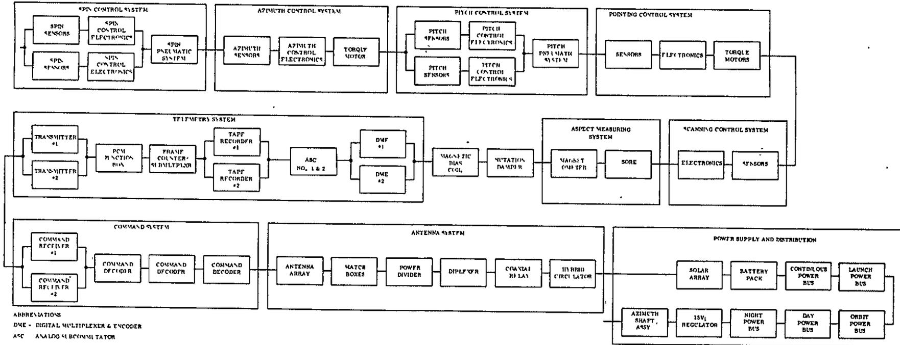
Figure 3-27. OSO-D Reliability Block Diagram
