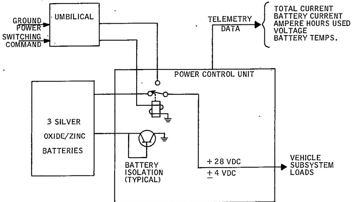
Figure 9.8-1. Electric Power Subsystem Block Diagram
