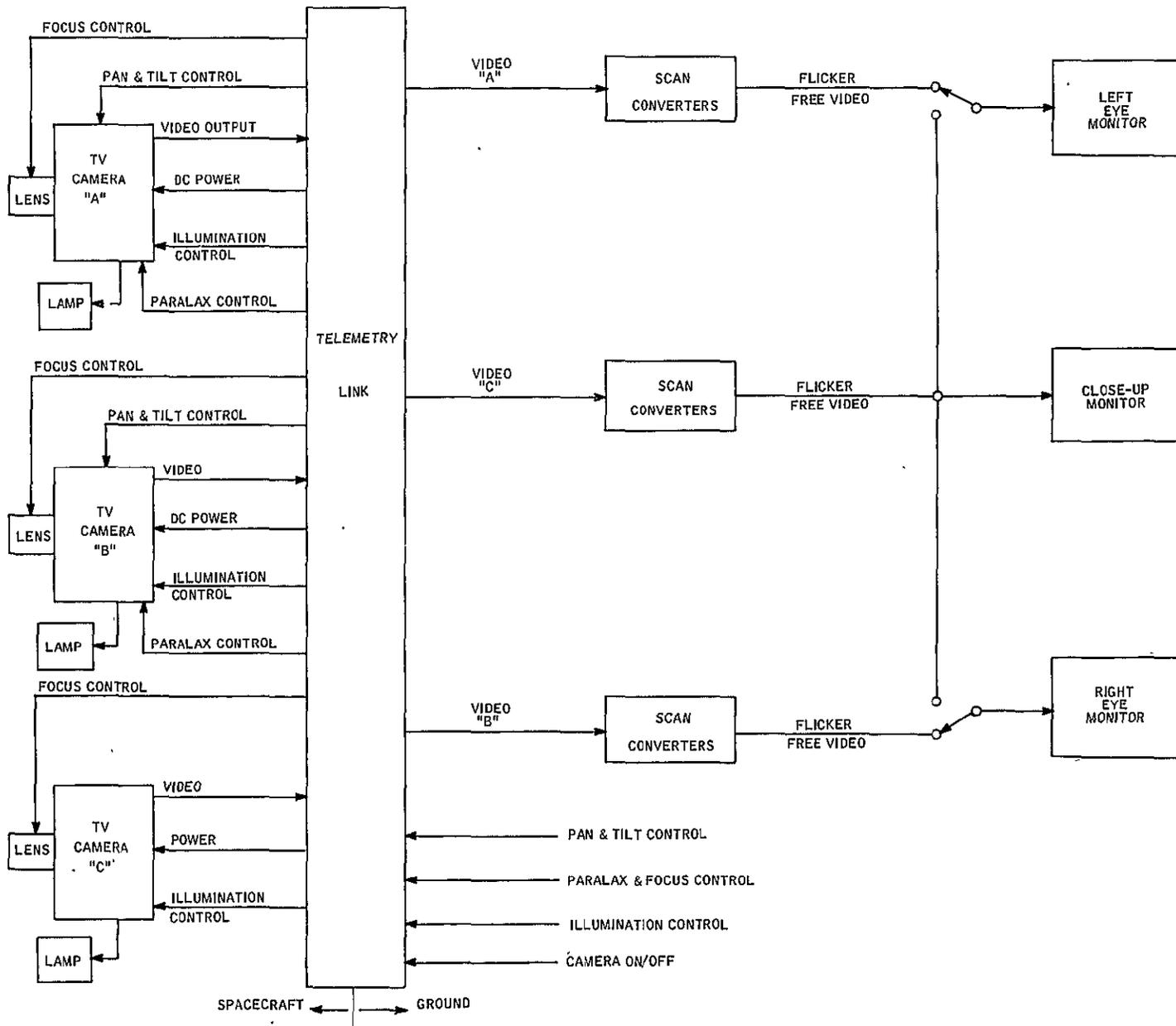
Figure 9.2-1. Video and Illumination Subsystem Schematic
