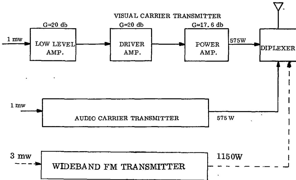
Figure B-8. UHF Transmitter Block Diagram
