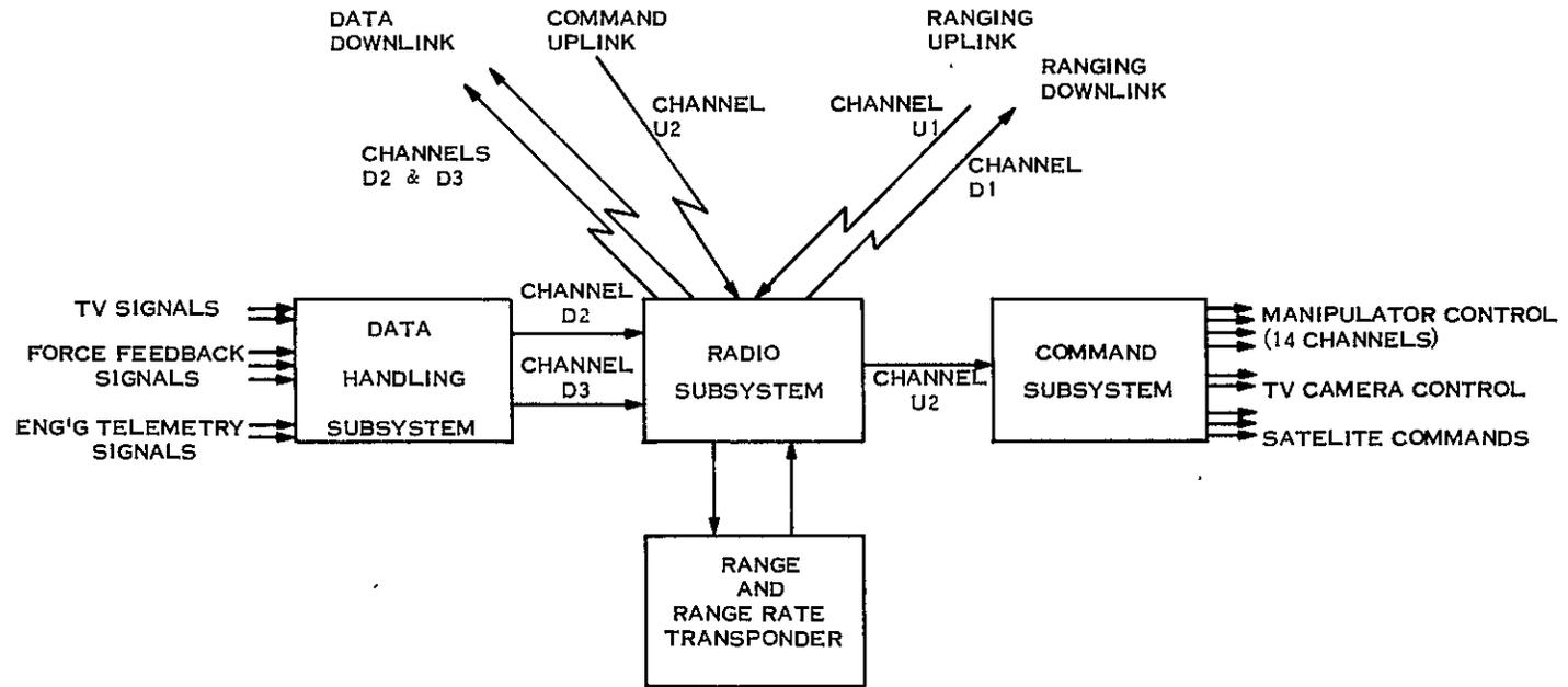
Figure 9.4-1. Communication Subsystem Functional Flow
