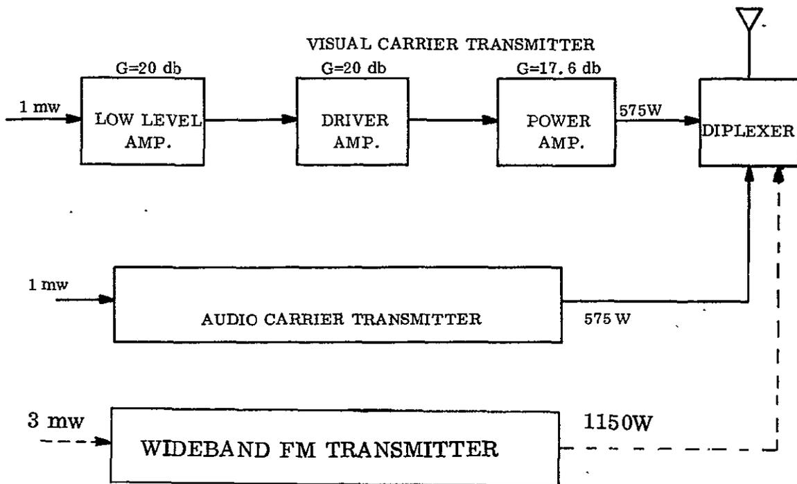
Figure B-8. UHF Transmitter Block Diagram
