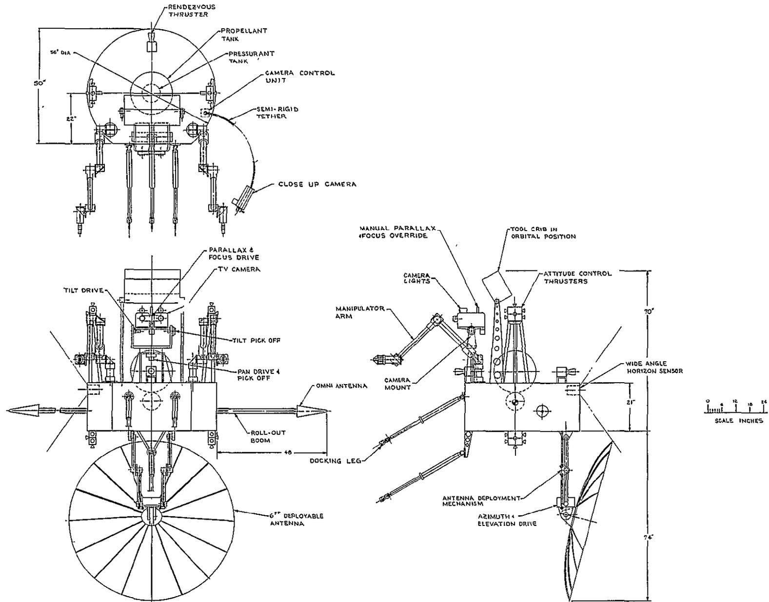
Figure 9.1-3. Basic Manipulator Spacecraft Orbital Configuration
