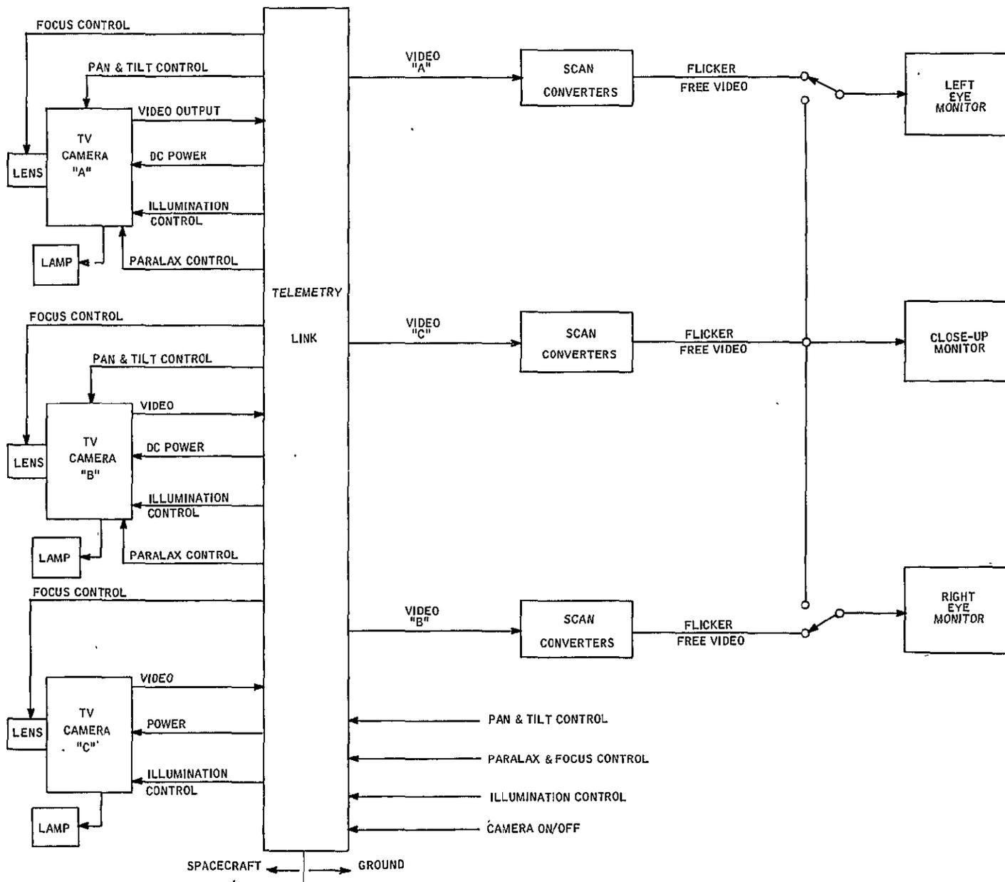
Figure 9.2-1. Video and Illumination Subsystem Schematic
