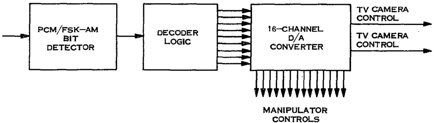
Figure 9. 4-5. Manipulator/TV Camera Control Decoder Block Diagram
