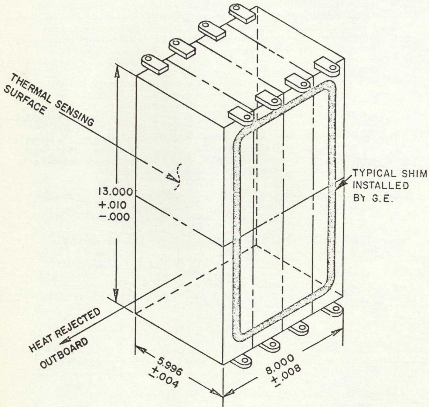
Figure 4-8. Nimbus Module Shimming
