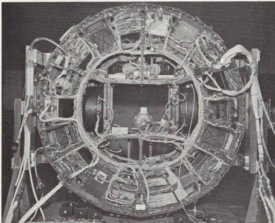
Figure B-17. Nimbus A Component Locations in Sensory Ring - Top View
