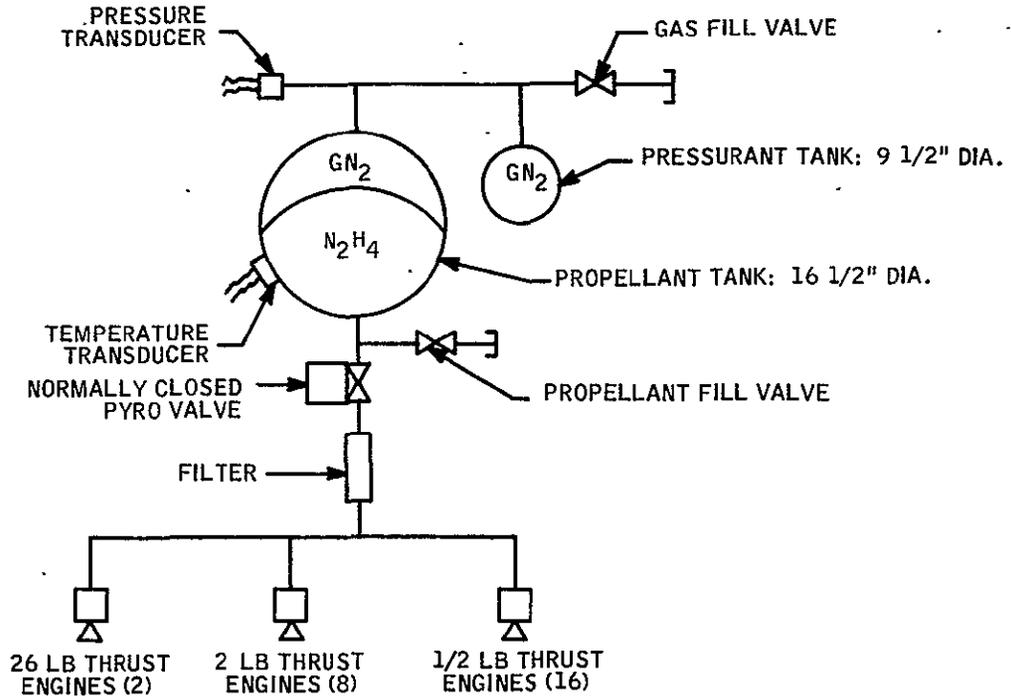
Figure 9.5-5. Propulsion Subsystem Schematic
