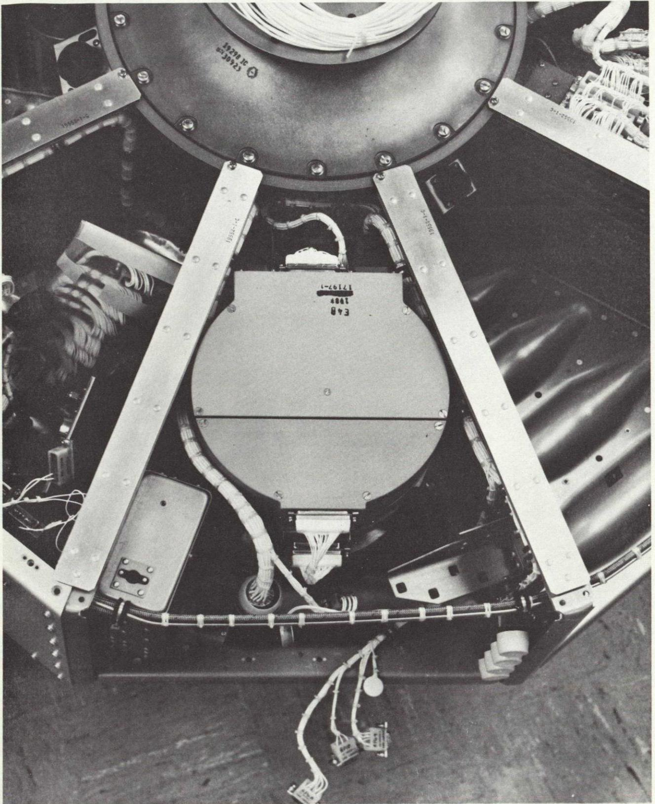
Figure 3-33. Tape Recorders in Compartment No. 8
