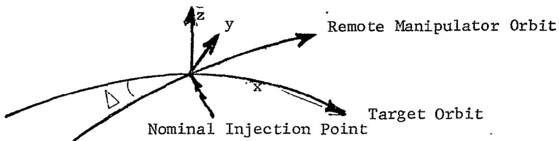
The velocity of the vehicle at injection is approximately 24440 ft/sec; this translates into the following dispersions:
