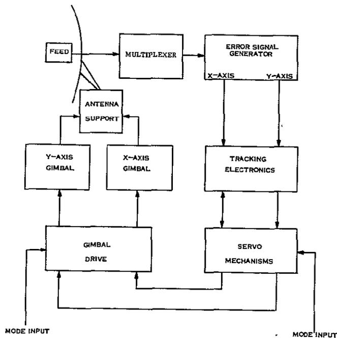
Figure 9.4-3. High-gain Antenna Tracking System
