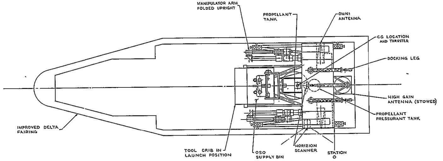
Figure 9.1-5. OSO Repair Configuration
