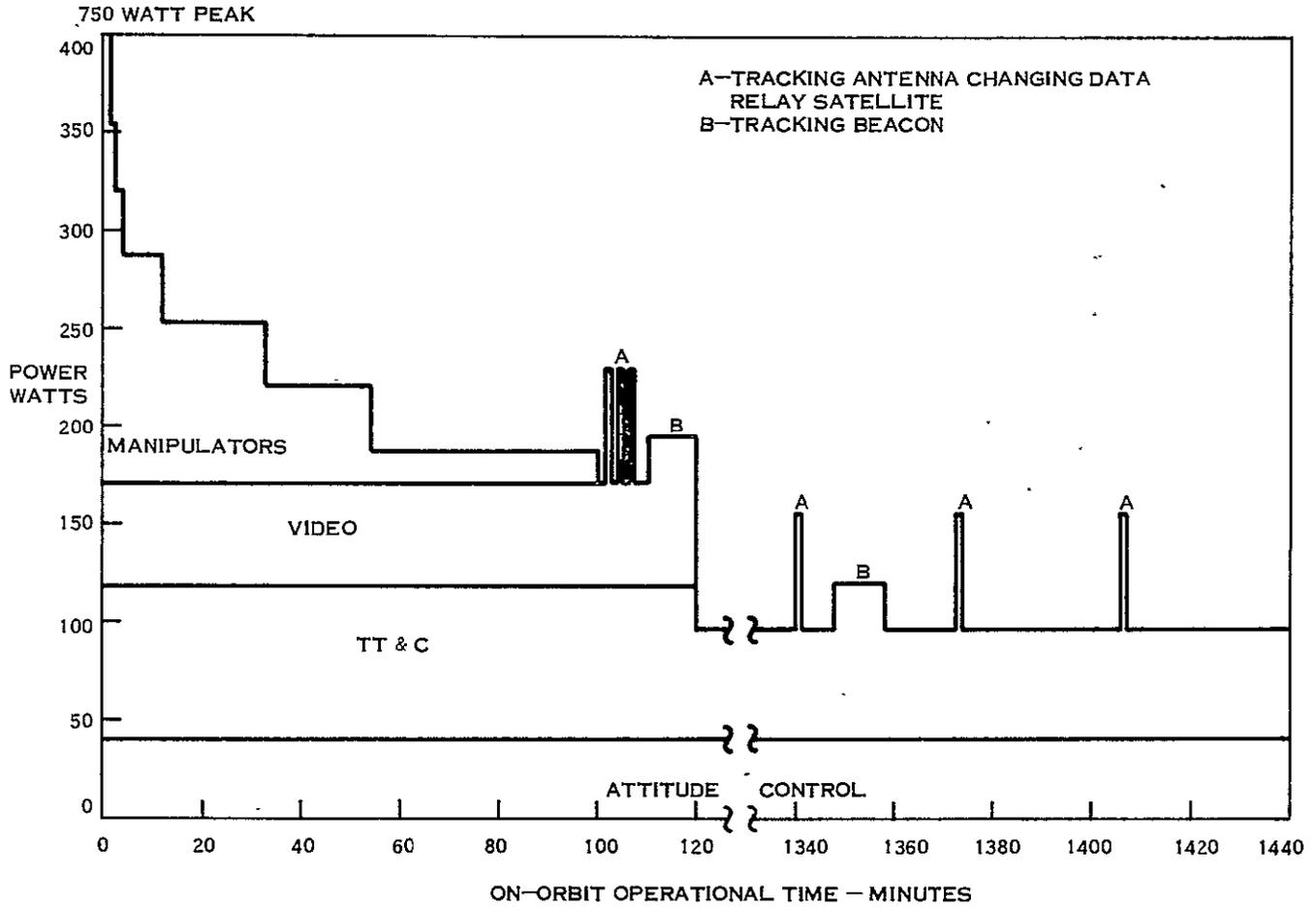
Figure 9.8-2. Manipulator Spacecraft Power Profile
