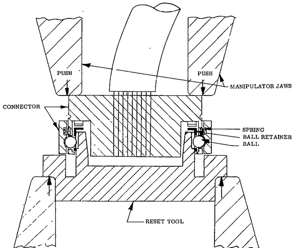
Figure 6-3. OA0 A1 Deutsch Connector Reset Device
