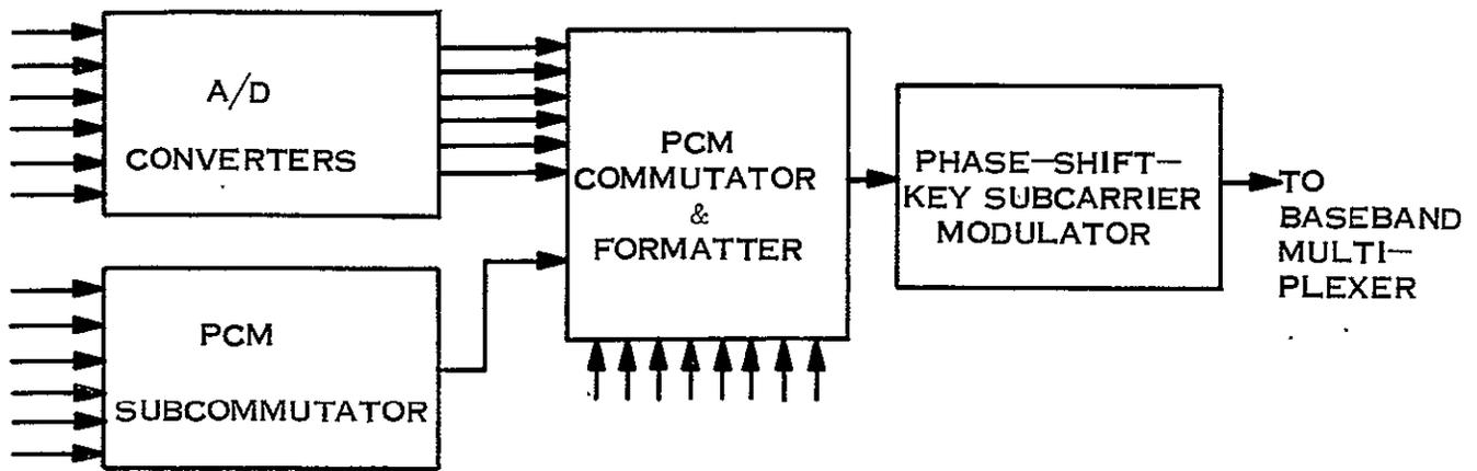
Figure 9.4-10. PCM Multicoder Block Diagram
