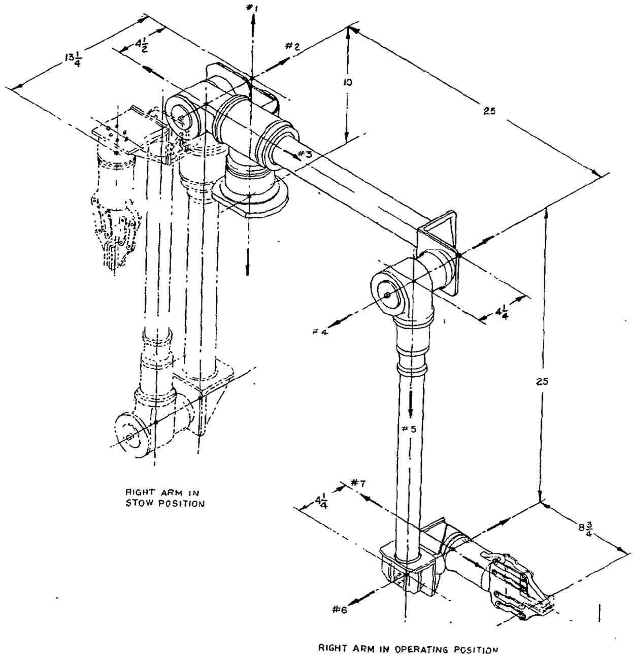
Figure 9.3-1. Isometric of Slave Manipulator
