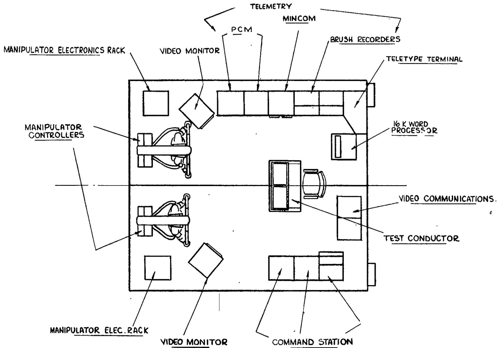
Figure 9.9-3. Ground Station Layout Plan View
