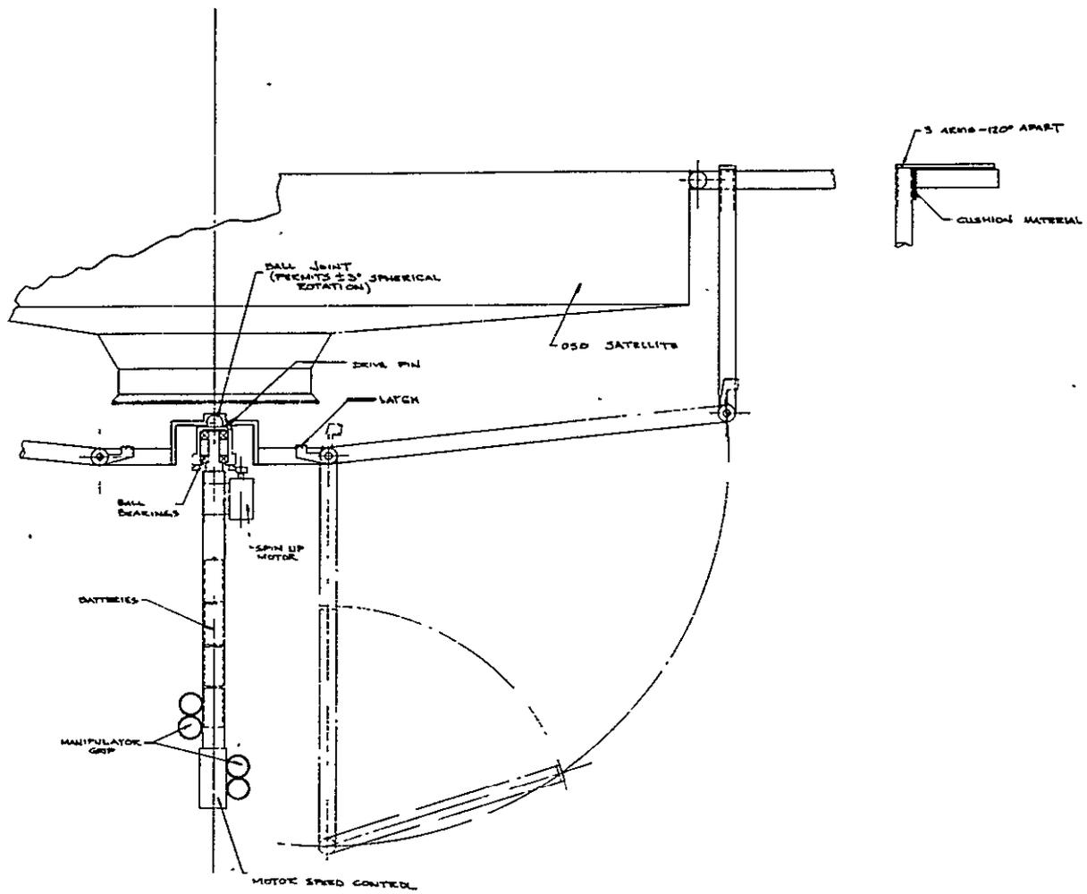
Figure 3-29. OSO-D Despin Fixture Rotating Hook Arms
