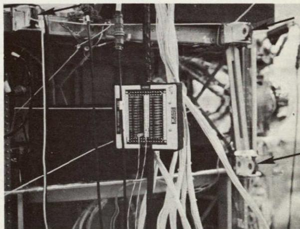
Figure 3-13. Three Mounting Clevises
