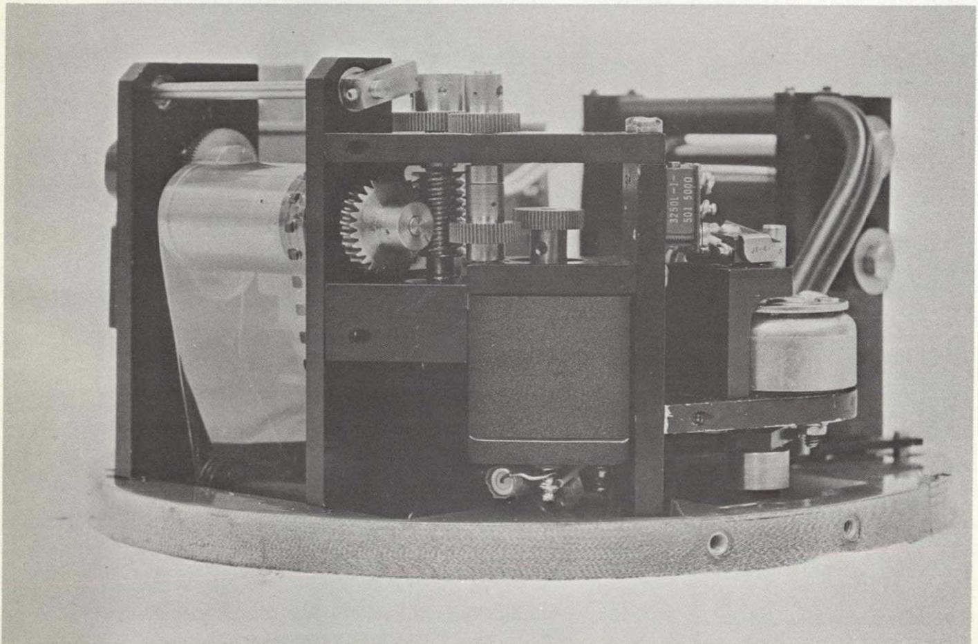
Figure 9.2-5. Automatic Light Control Shutter Assembly
