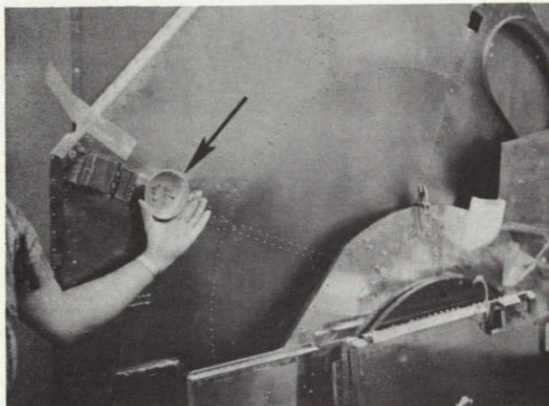
Figure 3-9B. SSC - Separation Spring Cup
