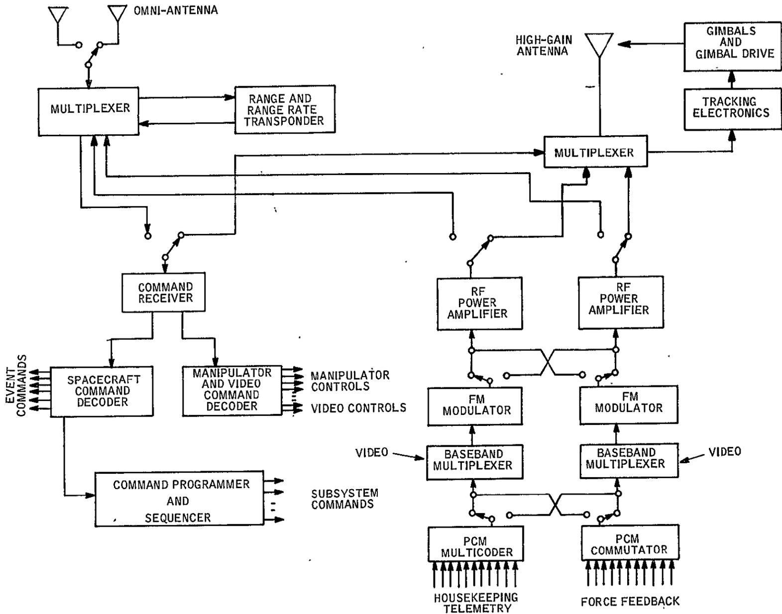
Figure 9.4-2. Radio Subsystem Block Diagram
