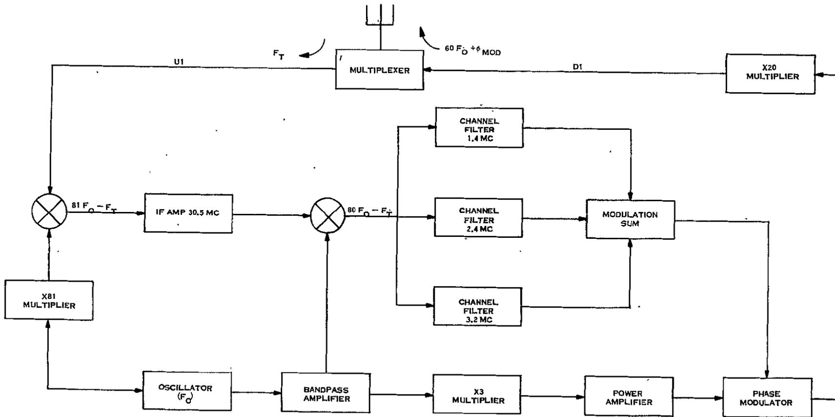
Figure 9.4-12. S-Band Transponder, Simplified Block Diagram
