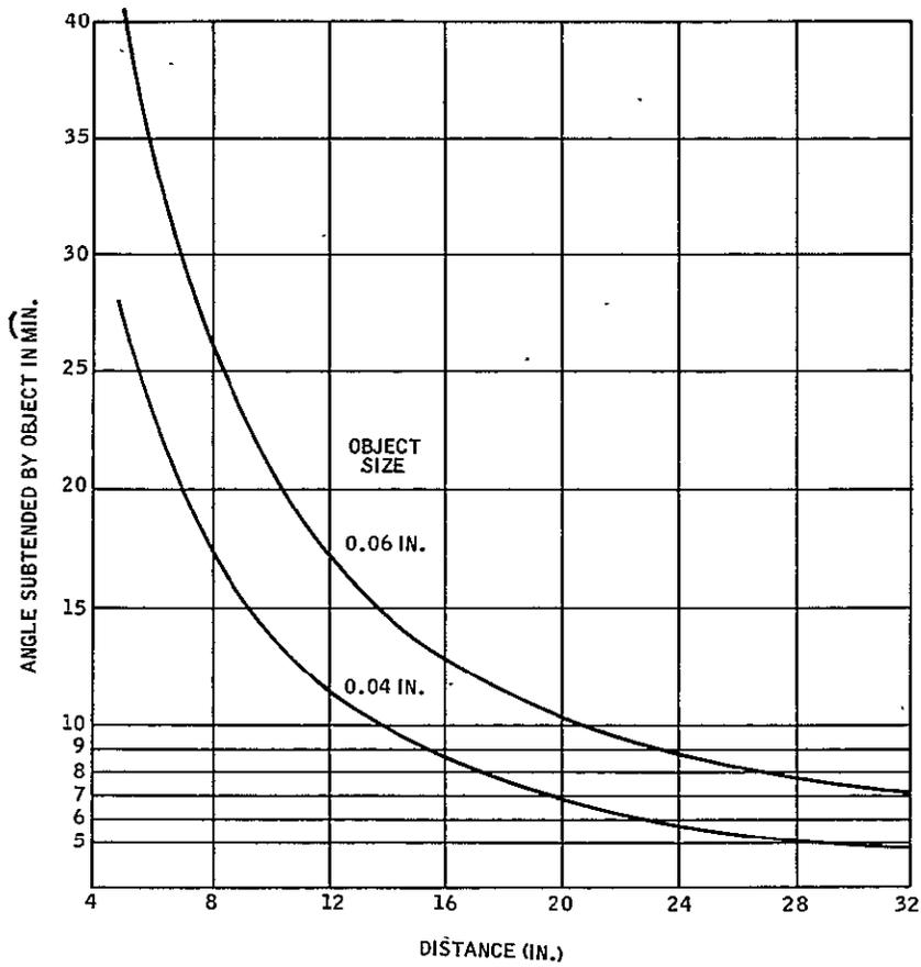
Figure 9.2-2. Subtended Object Angle Versus Distance
