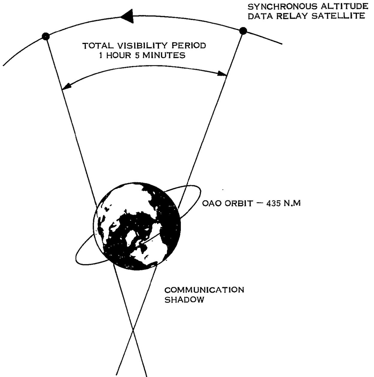
Figure 3-4. OAO, Synchronous Satellite Geometry
