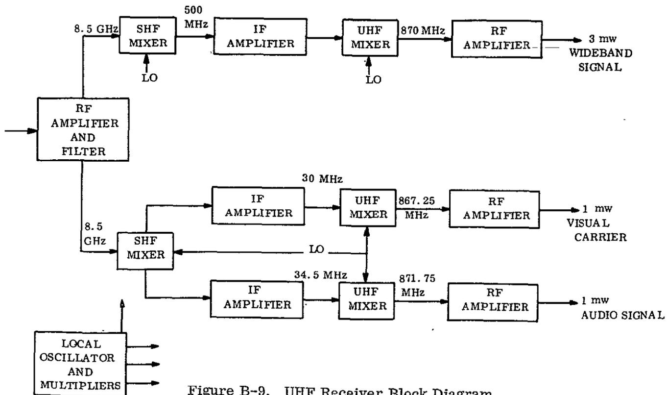
Figure B-9. UHF Receiver Block Diagram
