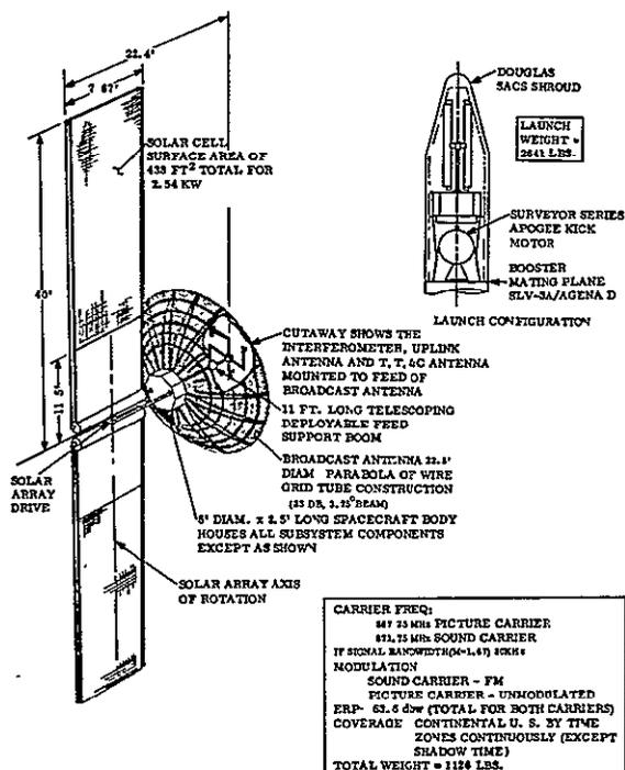
Figure 4-1. Direct Broadcast Satellite
