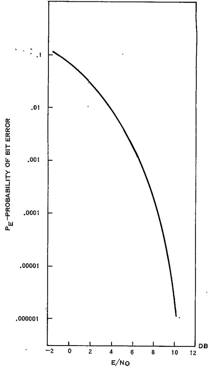
Figure 9.4-14.  $P_e$  versus  $E/N_0$  for PCM/PSK
