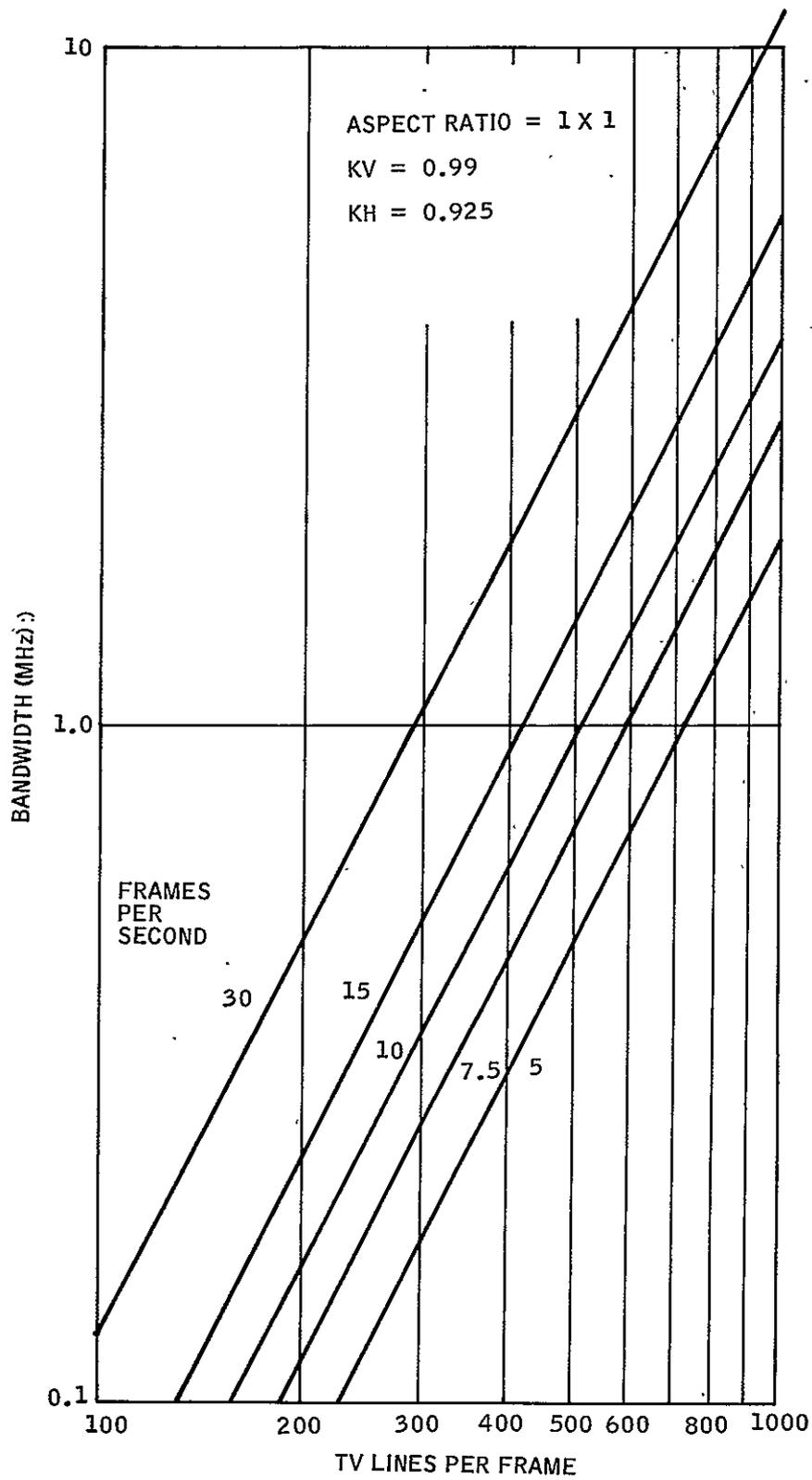
Figure 9.2-4. Bandwidth Versus TV Lines per Frame
