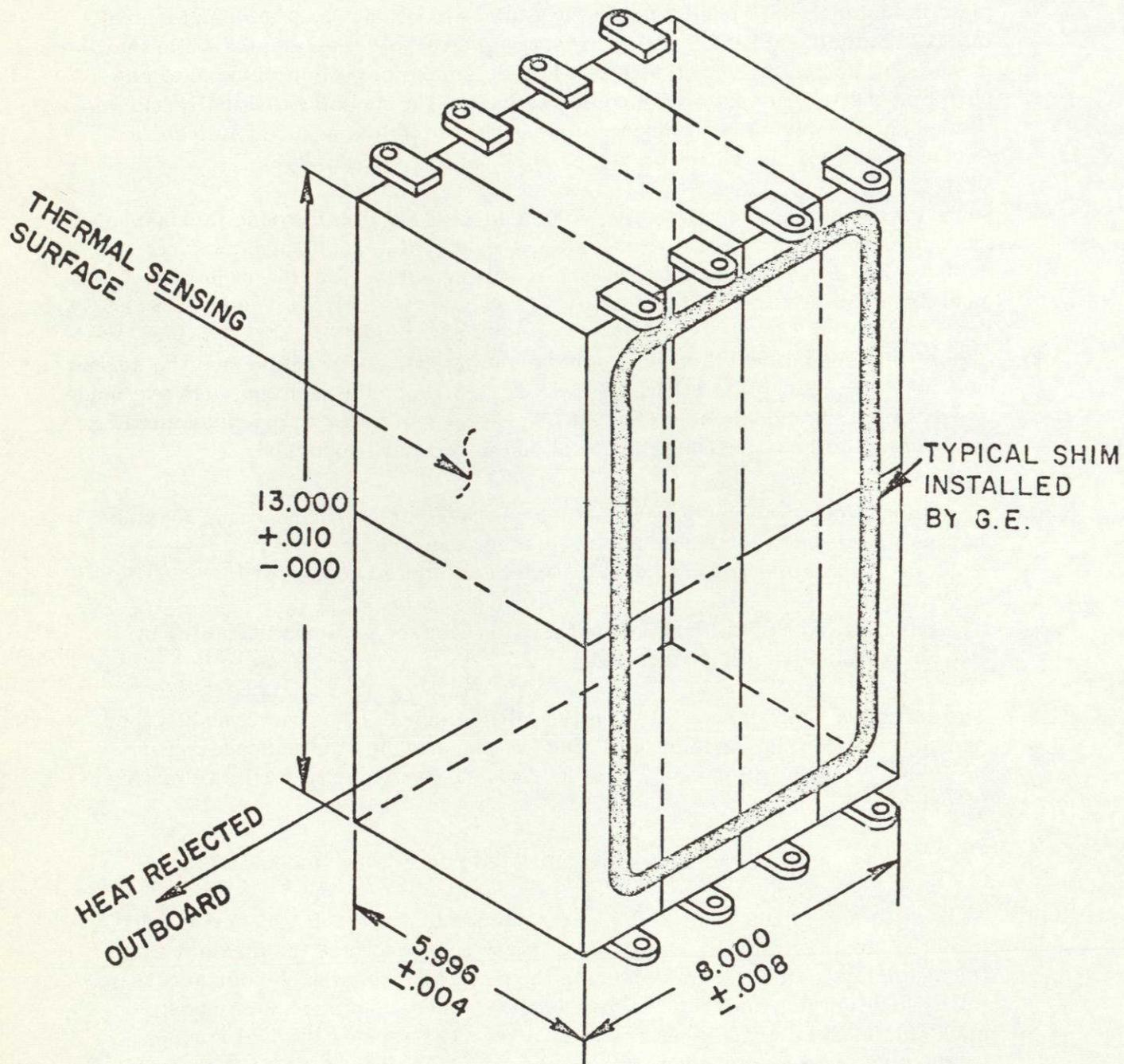
Figure 4-8. Nimbus Module Shimming
