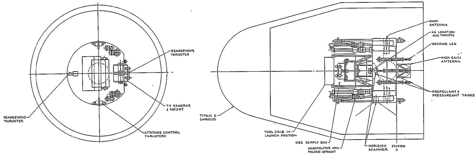
Figure 9.1-7. DBS Repair Configuration
