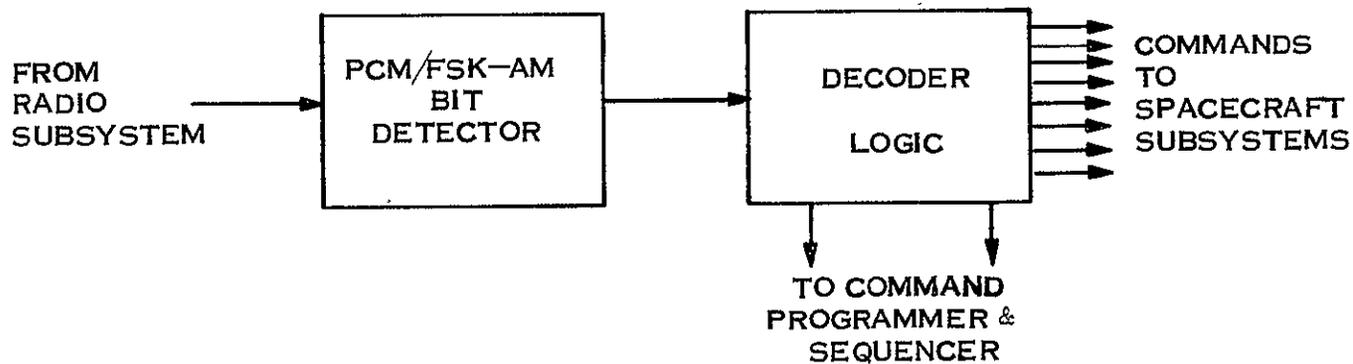
Figure 9.4-6. Satellite Command Decoder Block Diagram
