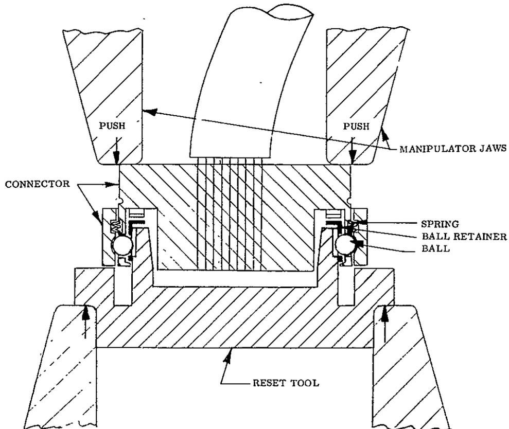
Figure 6-3. OAO A1 Deutsch Connector Reset Device
