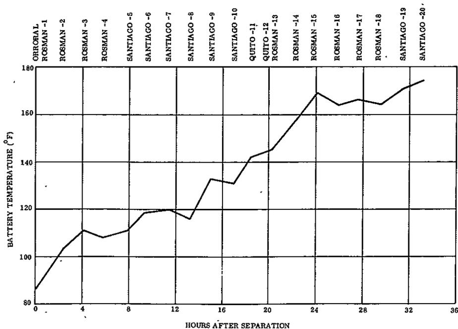
Figure 3-3. Battery Temperature Rise
