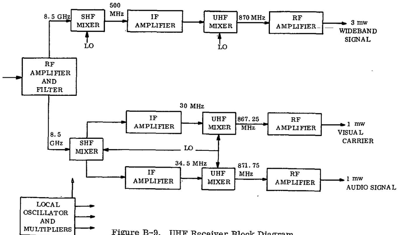
Figure B-9. UHF Receiver Block Diagram
