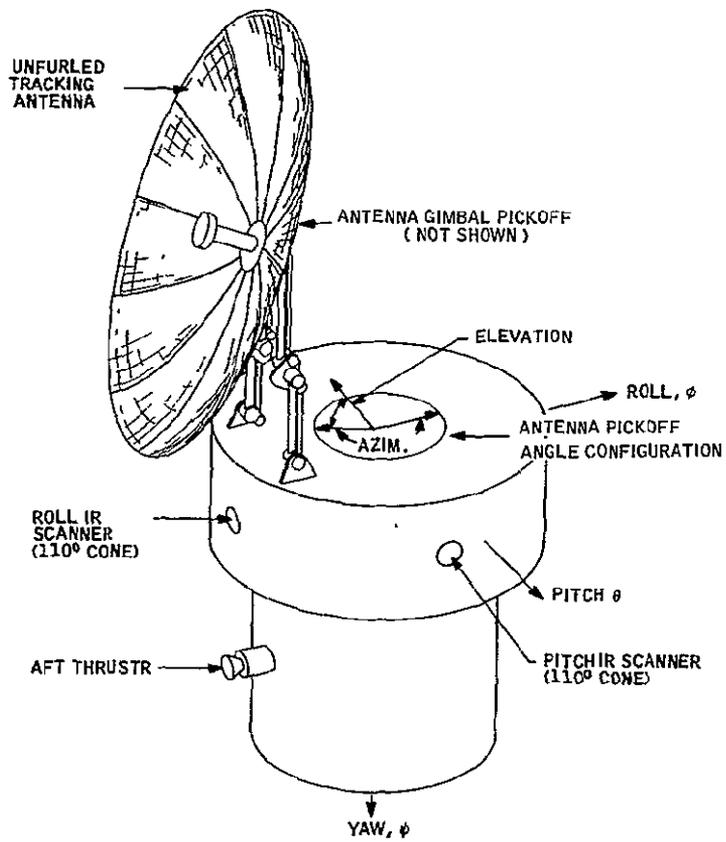
Figure 9.6-1. Location of IR Scanners and Tracking Antenna
