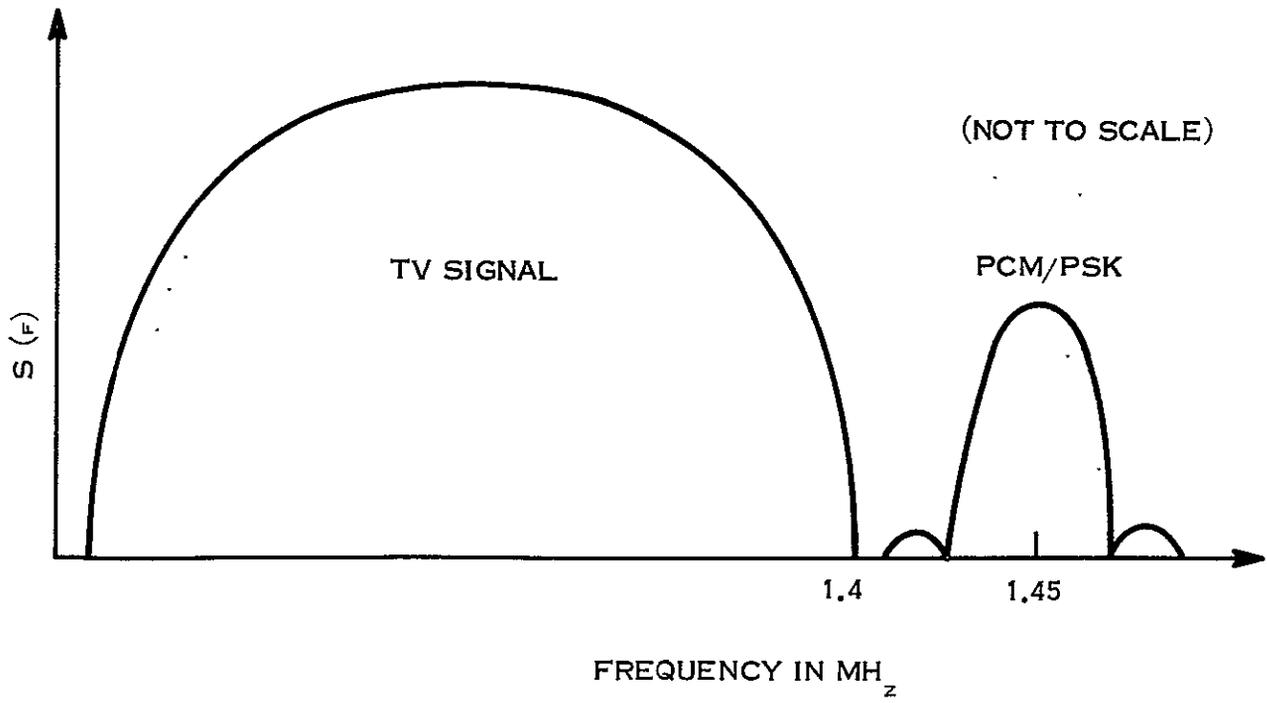
Figure 9.4-11. Composite Baseband Power Spectrum Plot
