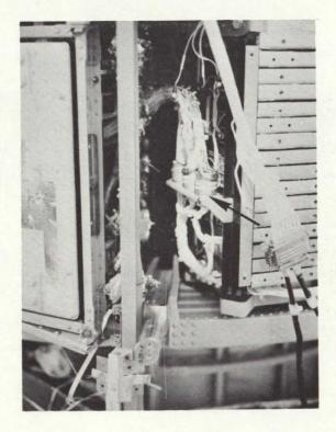
Figure 3-14. Power Output Side of Battery Pack (TA-2 has three connectors as shown, A-1 has only two)
