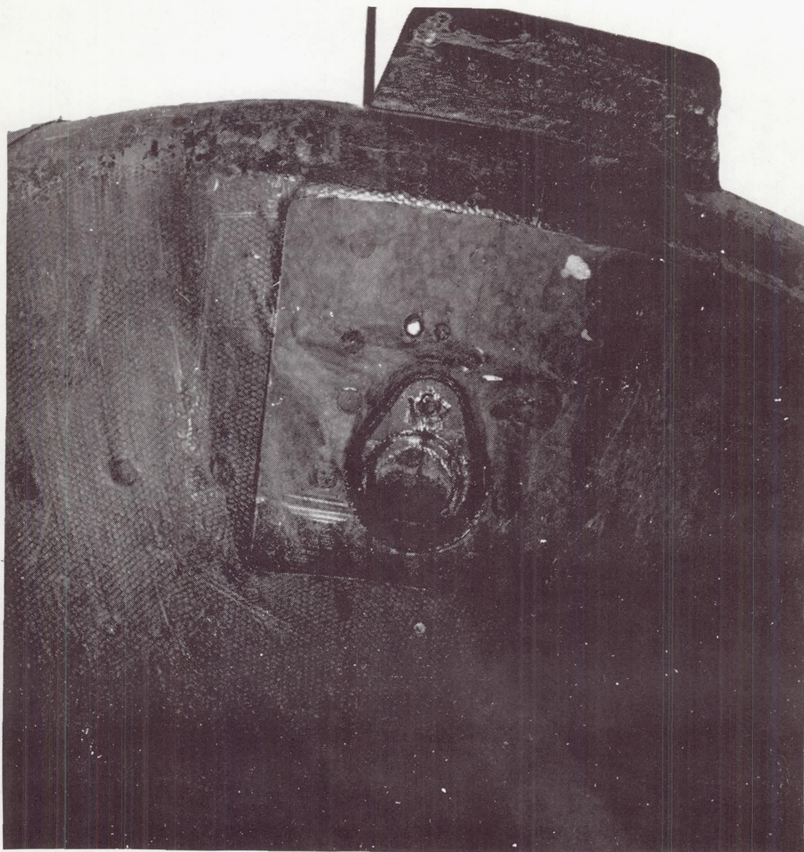
(h) Postflight photograph of CM-017 umbilical housing and ramp.
