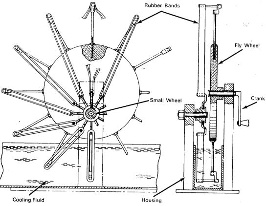
In analytical test work on the stress behavior of various types of elastomers, it is frequently observed that the internal temperature of rubber rises when it is stretched. The heat evolved by stretching rubber corresponds to the work required for such extension, and therefore, human mechanical energy is converted to heat in an efficient manner. A prototype device, shown in the figure, consisting of a rotating mechanism, a frame with multiple wide bands of rubber and a fluid
