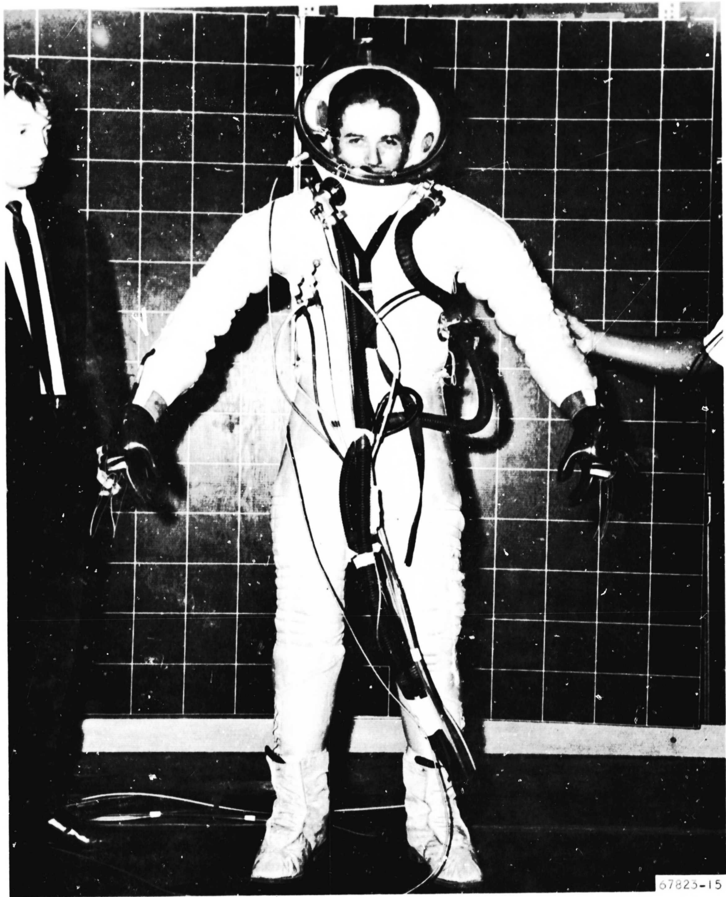
Figure 3. Phase D IVA Suit Pressurized to 3.7 Psig
