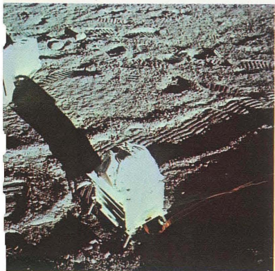
A close-up of the Solar Wind Spectrometer which is measuring the energies of the particles that make up the solar "wind." A vast flow of these particles is spun off by the Sun at very high velocities. The experiment has sent good data from the outset and its readings have been consistent with those of the magnetometer.
