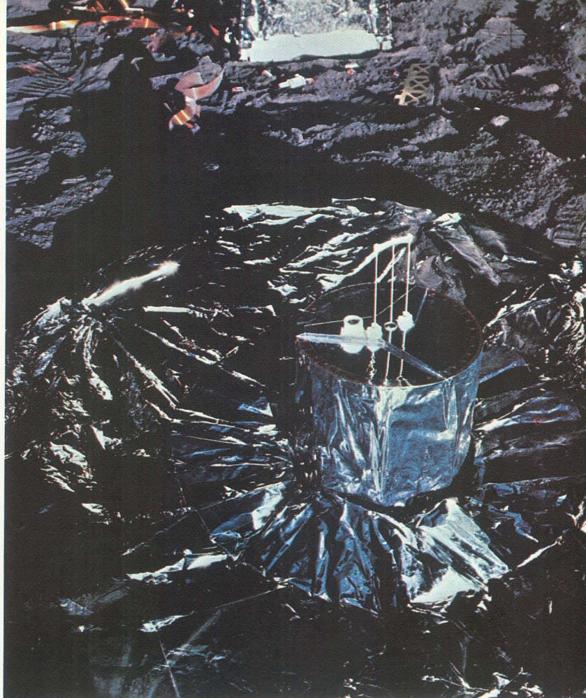
The Seismometer which recorded Intrepid's crash landing on the Moon, and other natural lunar events.
