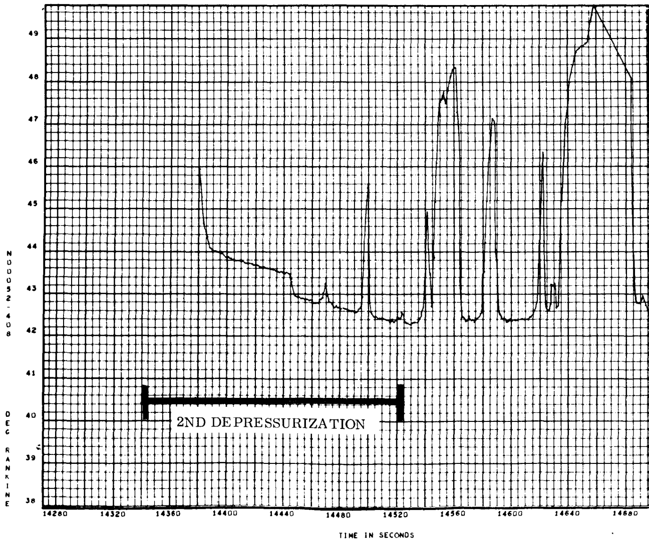
Figure 4-4. Response of Liquid-Vapor Sensor NO52 During Second Depressurization
