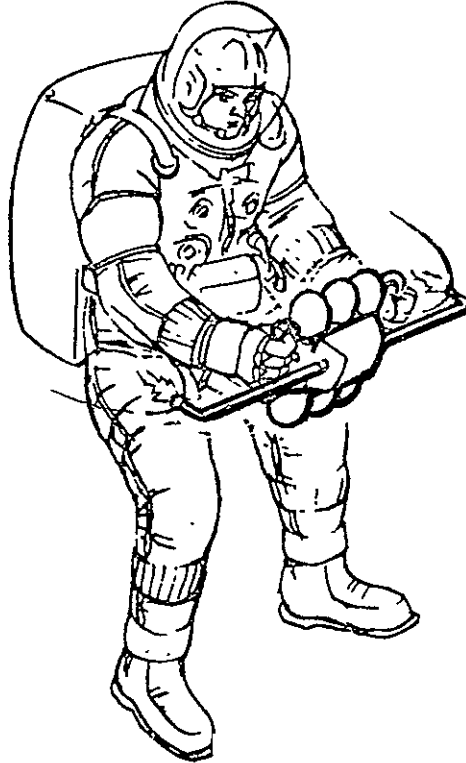
FIGURE 4-4 HAND-HELD MANEUVERING UNIT
