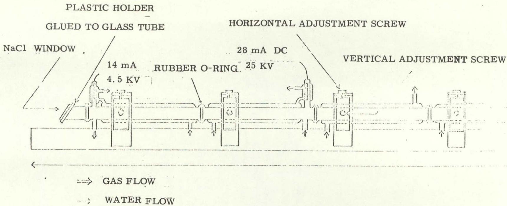
Figure 17. Laser amplifier. Section two, exit towards atmosphere
