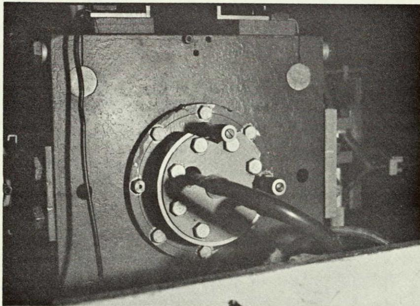
Fig. 9. - Mount for the fixed mirror.
