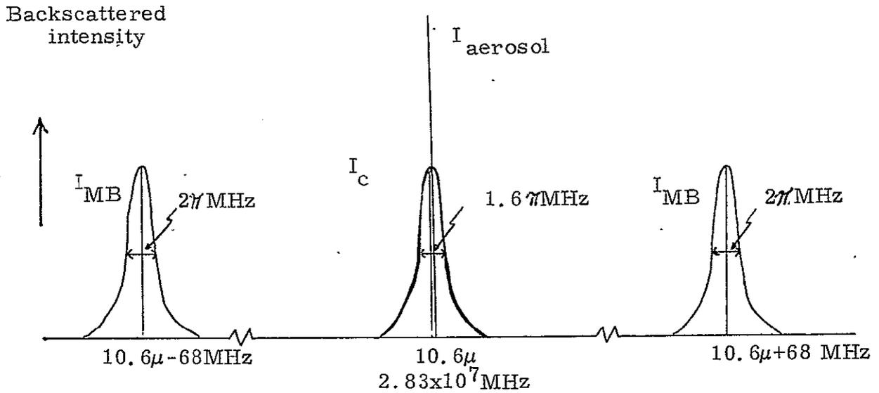
Figure 4. Expected frequency distribution of  $\text{CO}_2$  laser light scattered from the atmosphere
