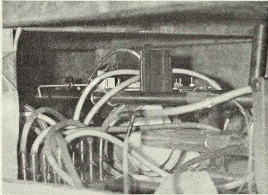
Fig. 8. - Discharge tube support for the oscillator.
