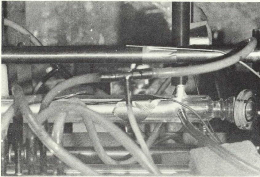
Fig. 15. - Brewster angle window for the oscillator.
