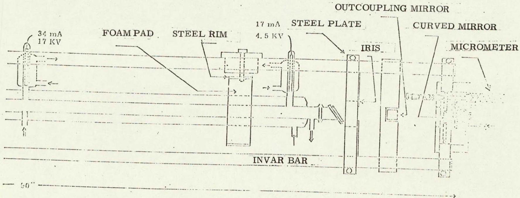
Figure 10. The Laser Oscillator
