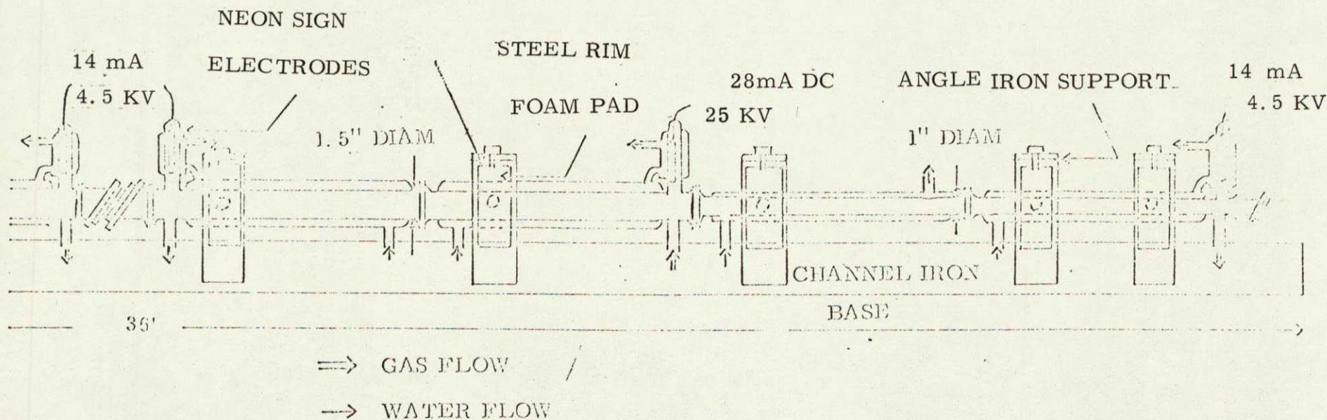
Figure 17. Laser amplifier. Section one, adjacent to oscillator.
