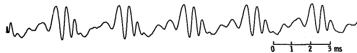
FIGURE 2. Evoked potentials recorded in inferior colliculus during a train of tone bursts, each 0.3 msec in duration including 0.1-msec linear rise followed by 0.1-msec linear decay, composed of 90-kHz sound at -15 dB referred to an arbitrary high intensity, repeated at 300/sec. Loudspeaker and porpoise's head were in the air 75 cm apart (2.2 msec sound conduction time). Sixty-four sweeps computer-averaged. Brief tone bursts every 3.3 msec evoke a potential after latency of 3.5 msec corrected for air time, consisting of a short complex of deflections less than 1 msec wide (ref. 27).
