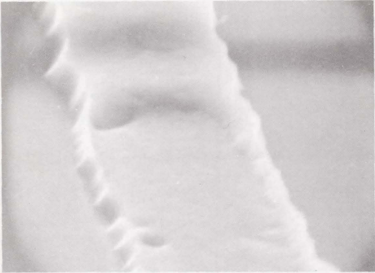
Figure 3—SEM picture of good metallization. Aluminum at oxide step is smooth and continuous. Magnification is 5500X.
