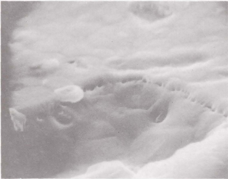
Figure 4—SEM picture of marginal metallization. A borderline case because of the number of discontinuities in aluminum at oxide step. Magnification is 5500X.
