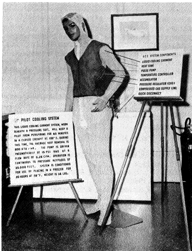
Figure 15.10 Flight-rated liquid-cooled garment.
