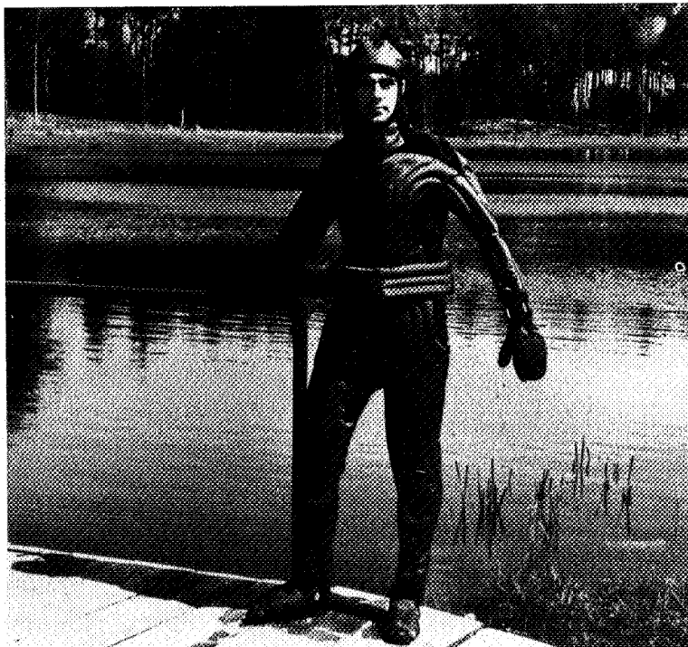
Figure 14.4 Closed circuit hot water undersuit at present under trial.
