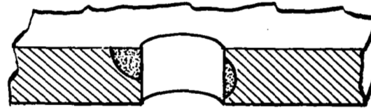
PART THROUGH CRACKS EMANATING FROM HOLES
