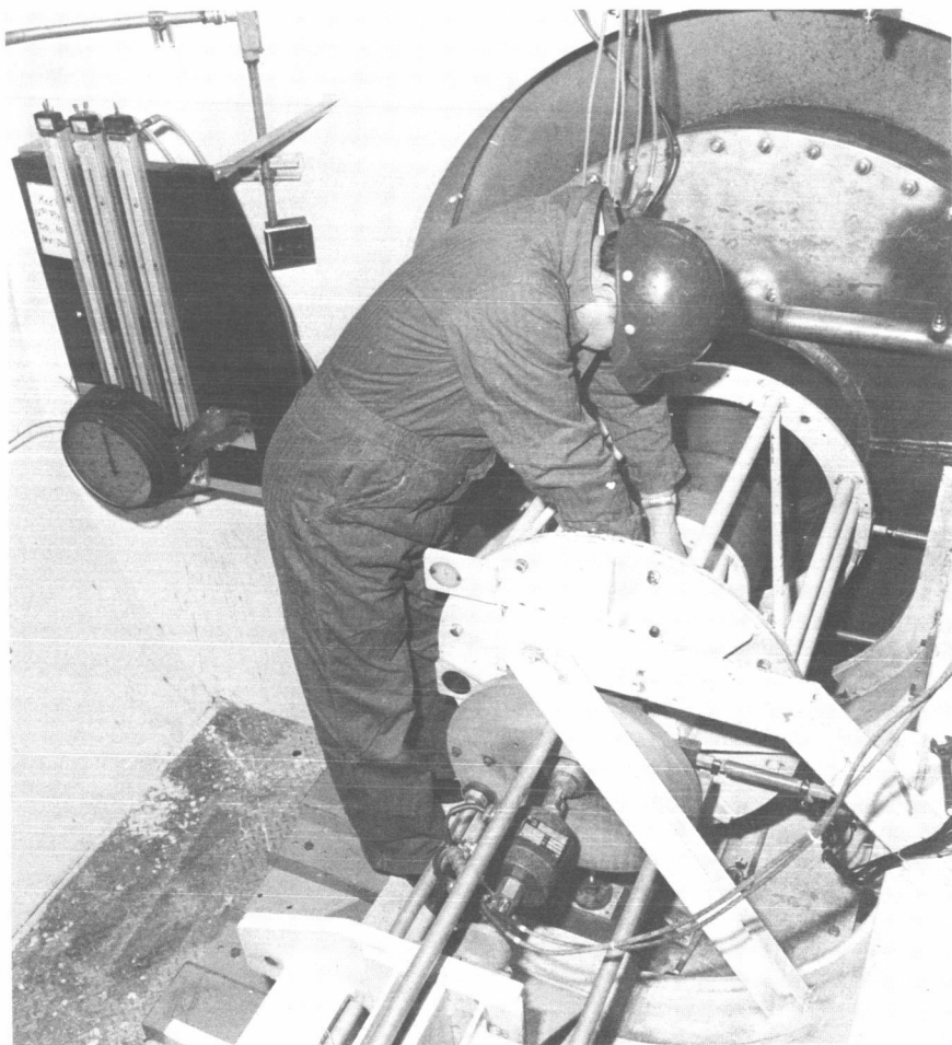
Figure 1. JPL motor P-43 at AFRPL cell 1-42A
