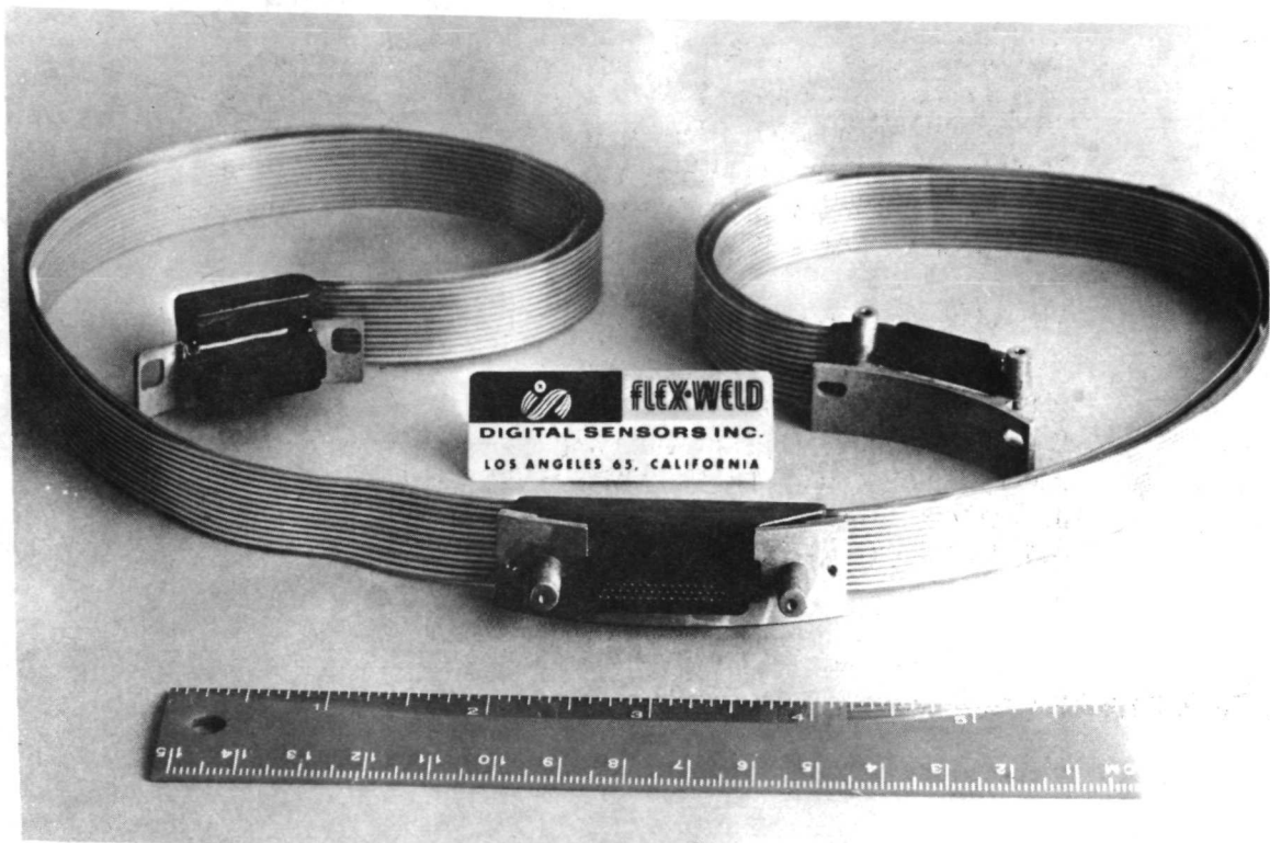
Figure 49. Gyro harness assembly (Digital Sensors, Inc., is now part of Ansley Electronics Corporation).
