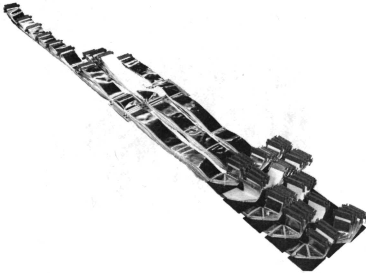
Figure 37. A completed 6-foot long 80-layer FCC harness 100 percent shielded.
