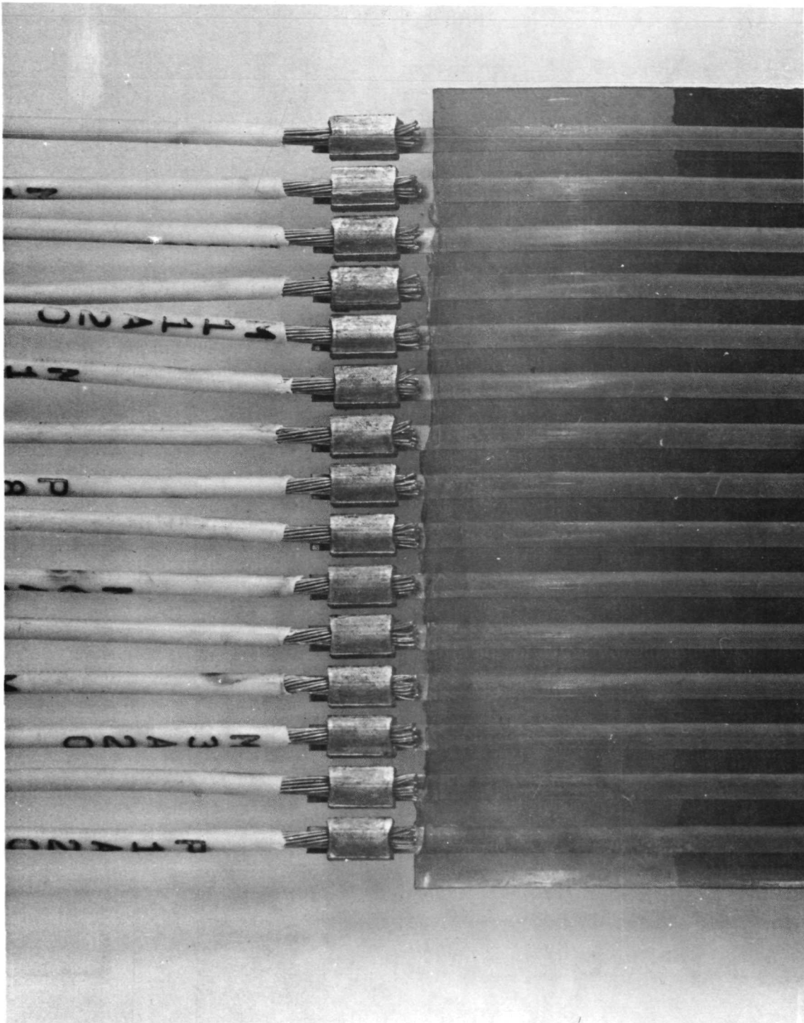
Figure 46. Crimped flat conductor to round wire transition using Thomas and Betts copper molded splices.
