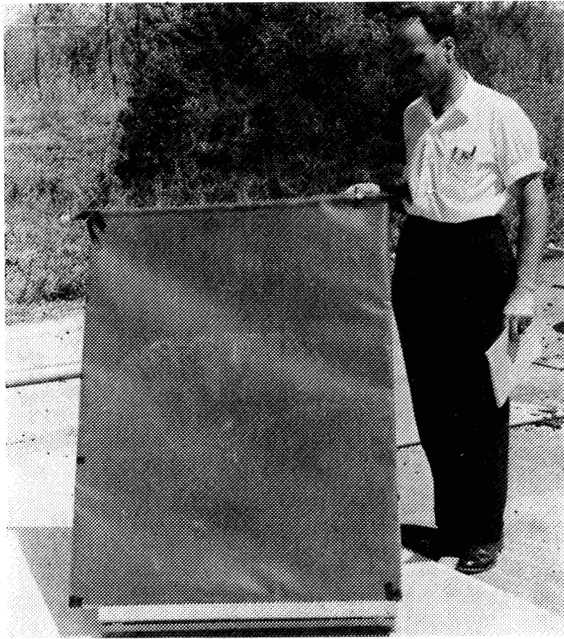
Figure 8. Swimming pool solar heater.
