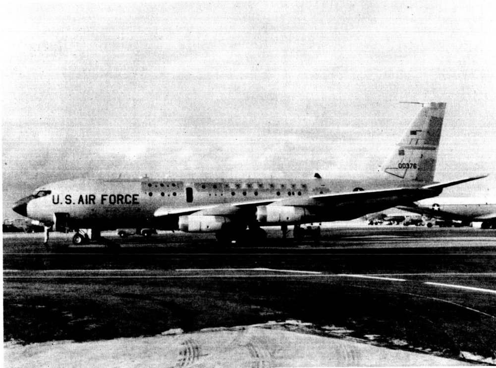
Figure 1. KC-135 with blade antenna for satellite communication.
