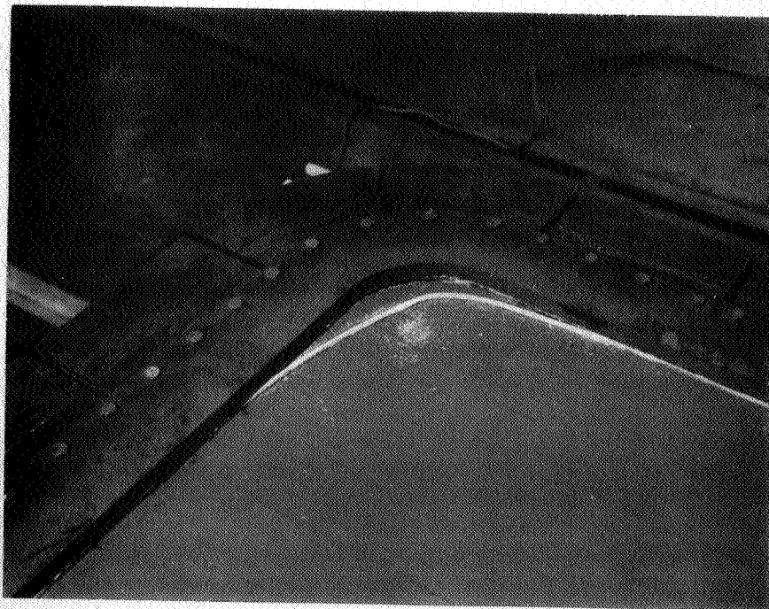
Figure 28. Closeup of Debonded Bumper Strip on Outer Windshield Test Specimen
