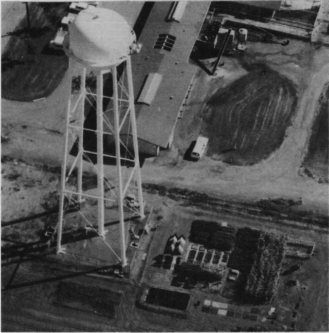
(a) Oblique aerial photo showing the water tower catwalk from which imagery was procured from a near-vertical angle of the target array below. Note that this target array contains crops, soil samples, soil moisture plots, water tanks, livestock, and color panels. Two Barnes Engineering thermal infrared sensors are mounted on the catwalk in this view.
