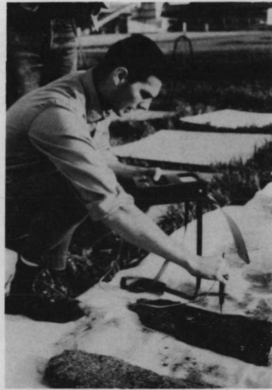
(b) Surface temperature of objects in the array can be measured using a surface temperature probe.
