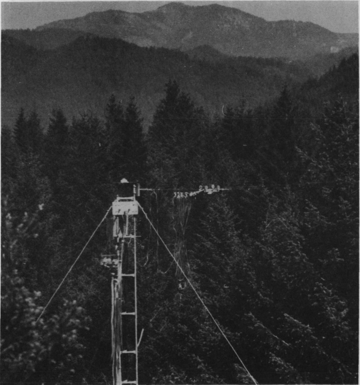
Figure 5. Net and total radiation thermometers are supported on moving tramway system above 30-meter-tall Douglas-fir ( Pseudotsuga menziesii [Mirb.] Franco) trees. These trees are being monitored for stress induced by Poria weirii root rot.
