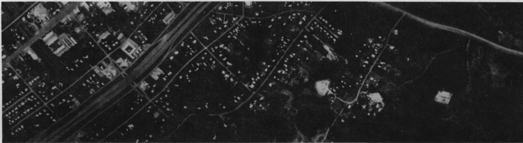
Figure 1 -- The interface between rural and urban surfaces at the edge of Houston, Texas as imaged by the RS-14 scanning thermal radiometer. Light tones represent relatively high emission of radiant energy or "radiance." Dark tones are lower levels of emission. From this image it can be clearly seen that an urban surface is a mosaic of sub-surfaces, each with its own thermal and radiant properties.
