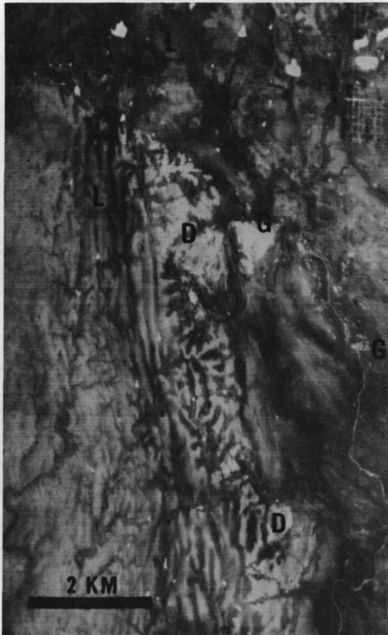
Figure 9. A predawn thermal infrared image of the Mill Creek test site (June, 1970). Contrast with the Dec. 8, 1968, results in figure 2. The most striking features are the relatively warm granite outcrops (G) in the June image. L, limestone; D, dolomite.
