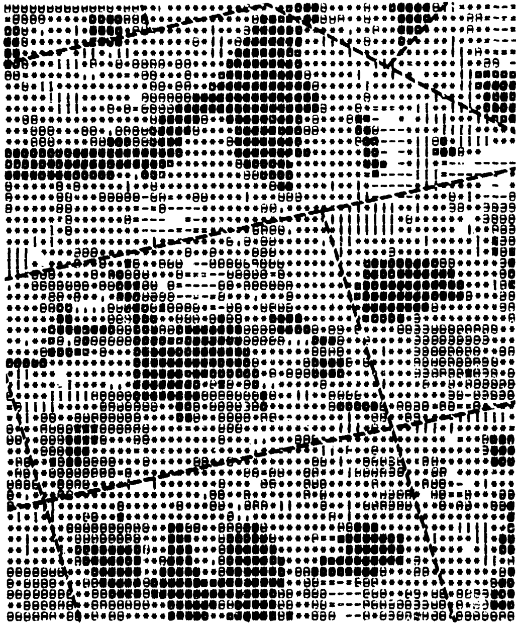
Figure 2. Computer recognition map showing correctly and incorrectly classified elements associated with forest cover; ● indicates correctly classified forest areas, ■ indicates forest areas misclassified, and ▼ indicates non-forest areas classified as forests.
