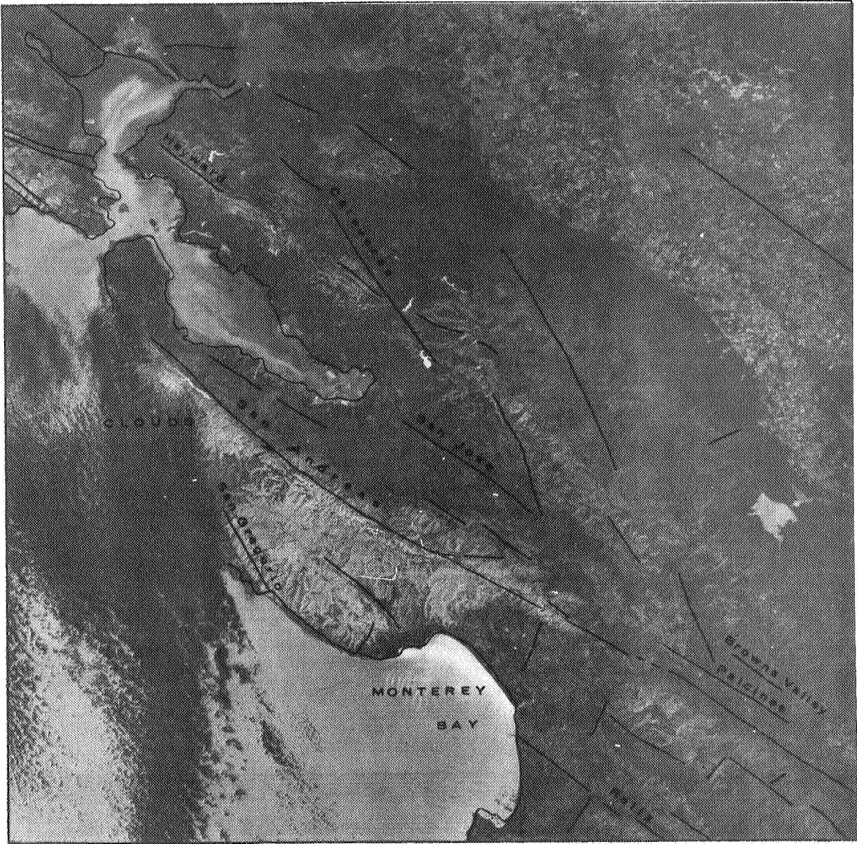
Faults and possible faults interpreted from pseudocolor transformation of ERTS-1 image
