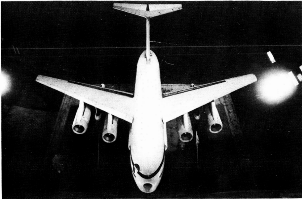
SWEPT WING MODEL INSTALLED IN THE 40-BY 80-FOOT WIND TUNNEL
