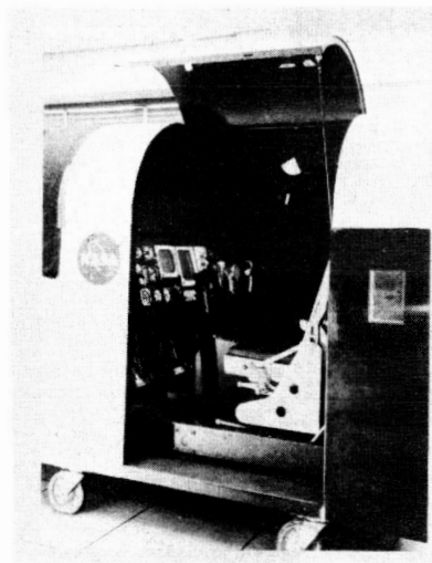
Figure 8.- STOLAND simulation cockpit.
