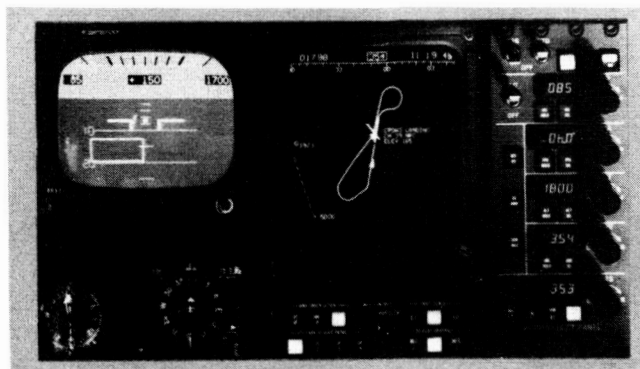
Figure 9.- STOLAND pilot display panel.
