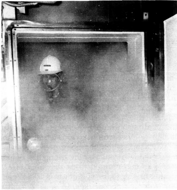
Figure 28. - Chamber fogging following a practice emergency repressurization and water deluge.
