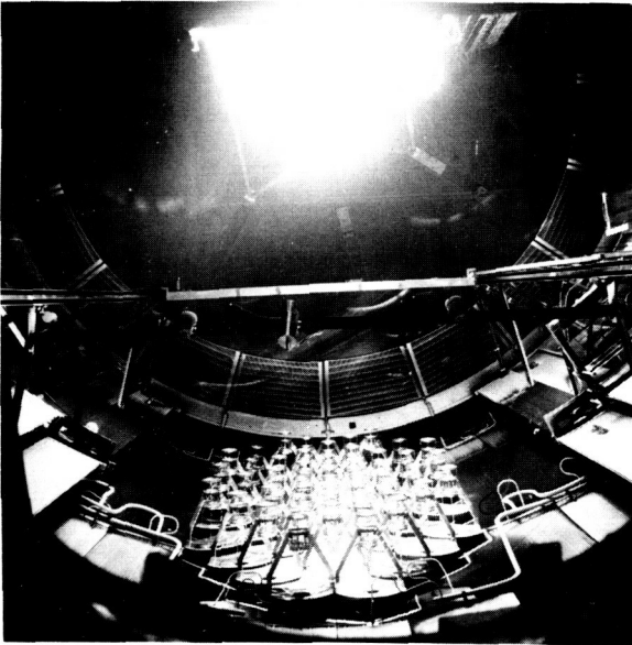
Figure 36. - Side-solar hot-soak and radiator-mode testing on spacecraft 008.
