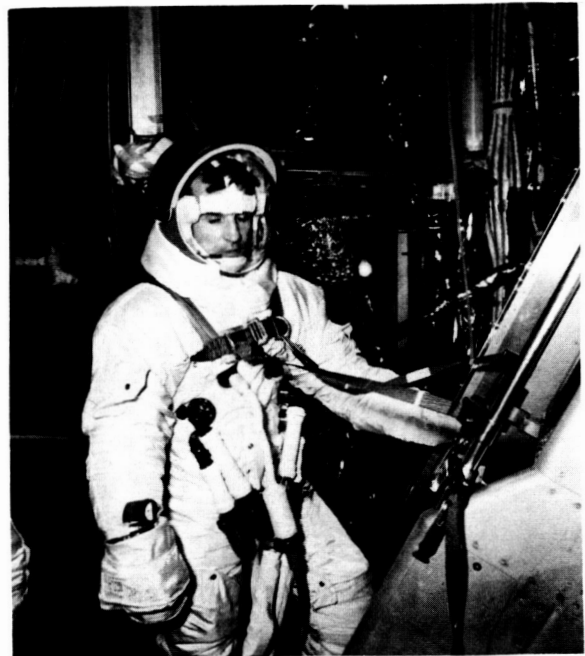
Figure 19. - Falling restraint system and umbilical connections.
