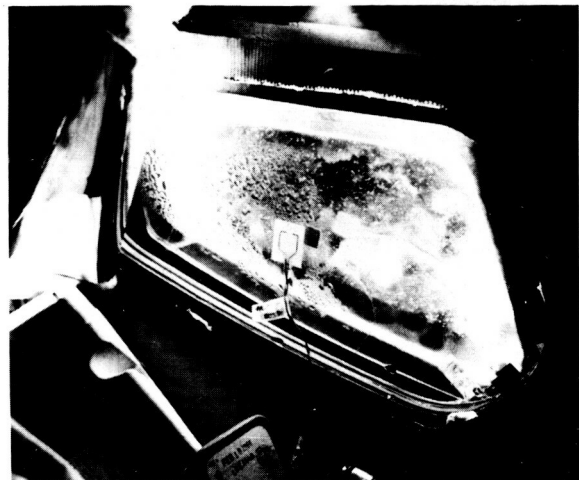
Figure 38. - Command module window fogging.
