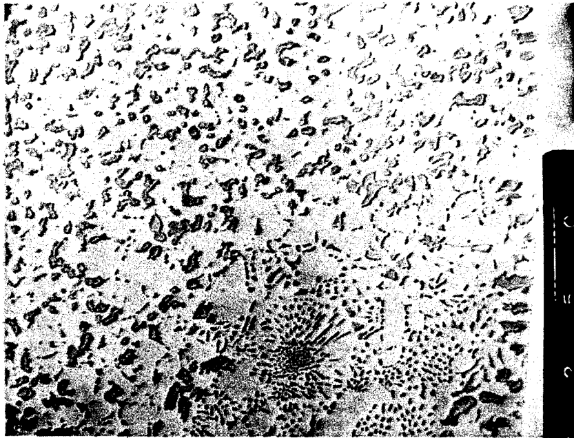
FIG. 29 SCANNING ELECTRON MICROGRAPH OF SLN 4-33mm - 220° ILLUSTRATING THE MIXTURE OF NORMAL AND ABNORMAL STRUCTURE IN THE RING-GROOVE FARTHEST FROM THE ZERO PLANE. (250X)
