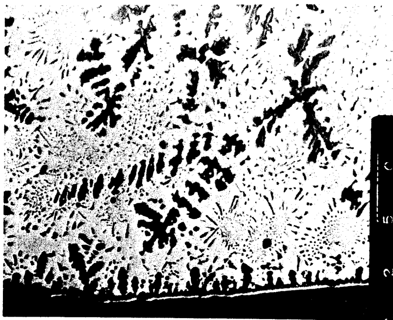
FIG. 26 SCANNING ELECTRON MICROGRAPH OF SLN 4-5mm - 290^\circ WITH A LARGE DENDRITE. (250X)
