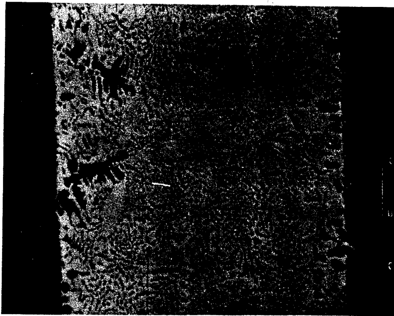
FIG. 19 SCANNING ELECTRON MICROGRAPH OF SLN-4-20mm - 120° SHOWING THE TWO KINDS OF PRIMARY PHASES. (250X)
