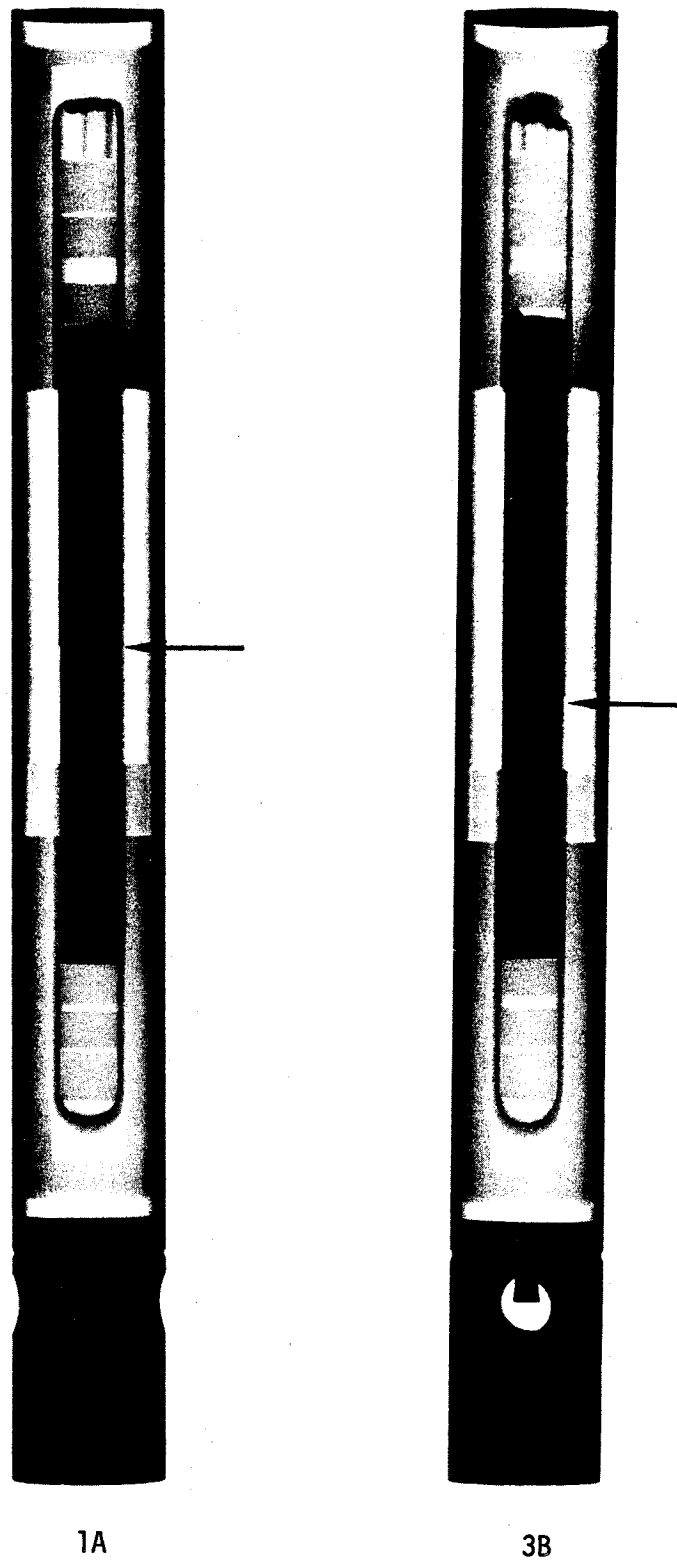
Figure 11. X-ray images of cartridges processed on the ground in a vertical position with the heater on top. Arrows indicate melt-back positions.
