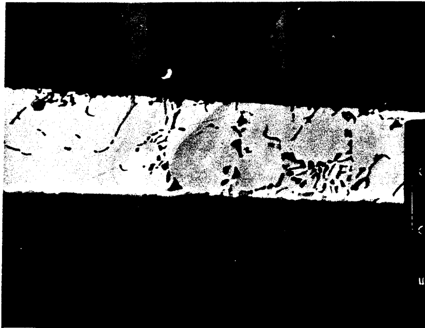
FIG. 32 SCANNING ELECTRON MICROGRAPH OF SLS 3-17mm - 5° SHOWING A MORE EXTREME CASE OF THE PRIMARY SILVER-RICH DENDRITES SEEN IN FIGURE 31. (500X).
