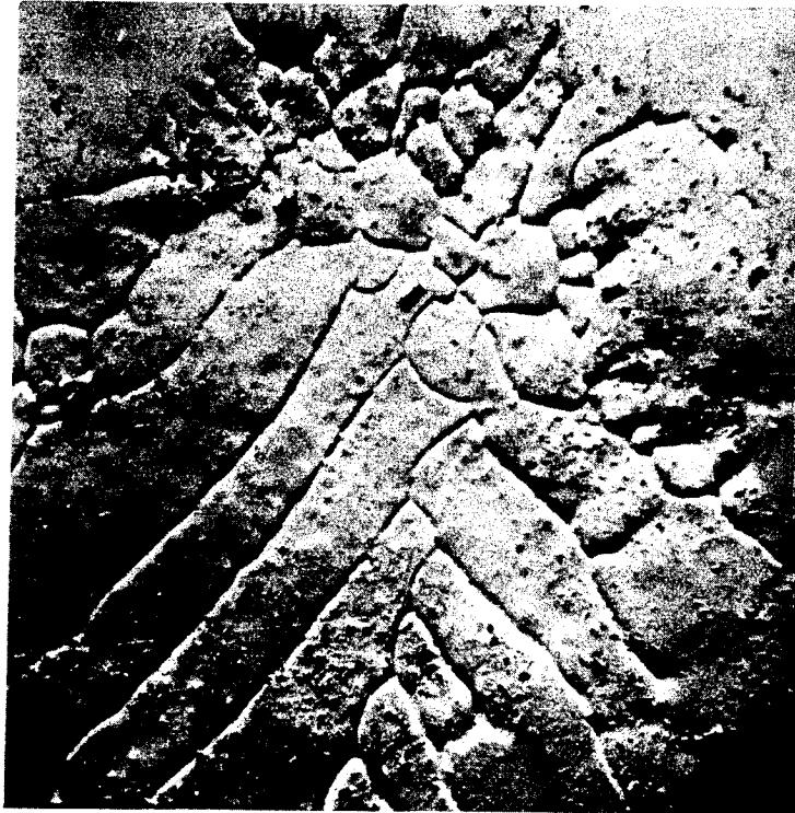
FIGURE 12. GROUND SAMPLE 3B P4 SHOWING CELLULAR SOLIDIFICATION SUBSTRUCTURE (X 45)
