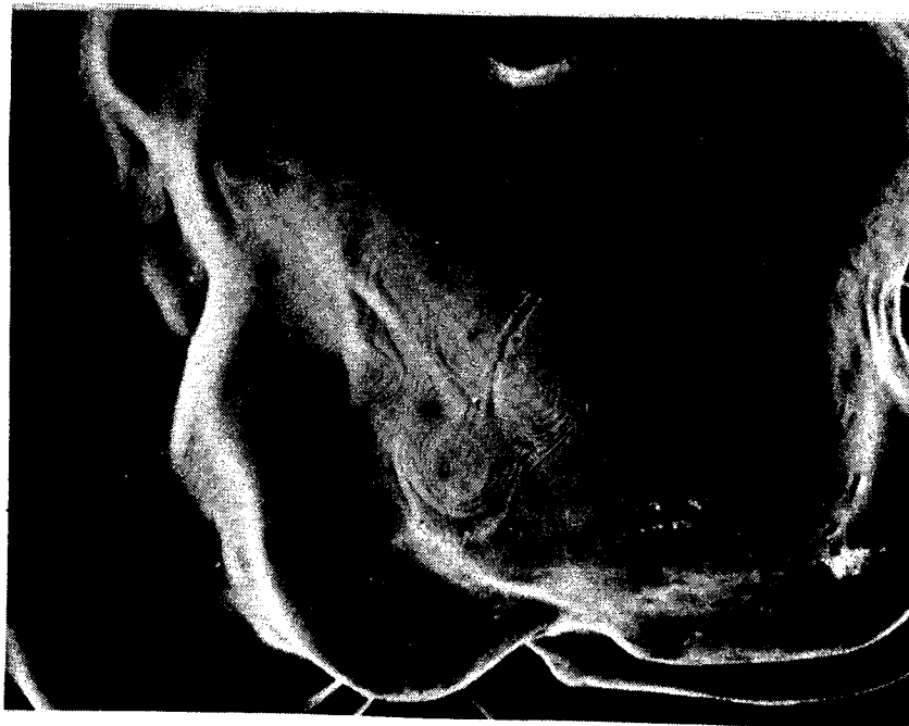
FIGURE 3B. TERRACING ON PRIMARY AND SECONDARY DENDRITE ARMS IN Ni-12 Sn SKYLAB SAMPLE 2.3 (3750X)
