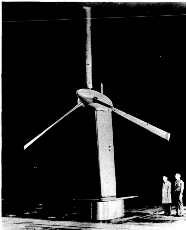
Figure 20. Bell 25-foot flight-worthy proprotor in NASA Ames full-scale tunnel for dynamic testing.
