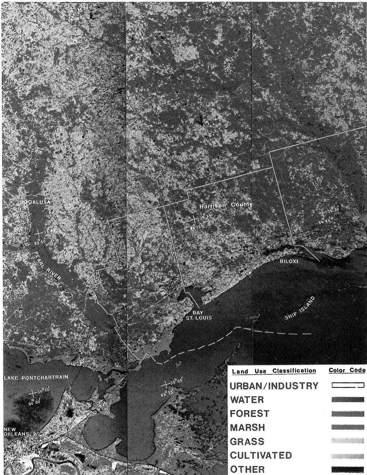
Figure 5. Computer-derived land use classification of ERTS data for the Mississippi Gulf Coast.
