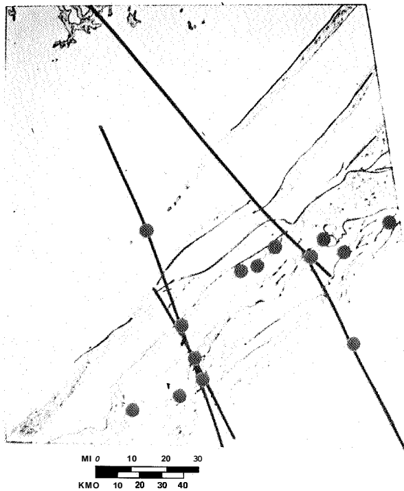
Figure 19a. Plot of two major lineaments crossing the folded Appalachians of northern Alabama (these lineaments were first detected in the ERTS imagery of that area); location of major barite mines and prospects shows a strong correlation with one lineament and some possible control by the second lineament.
