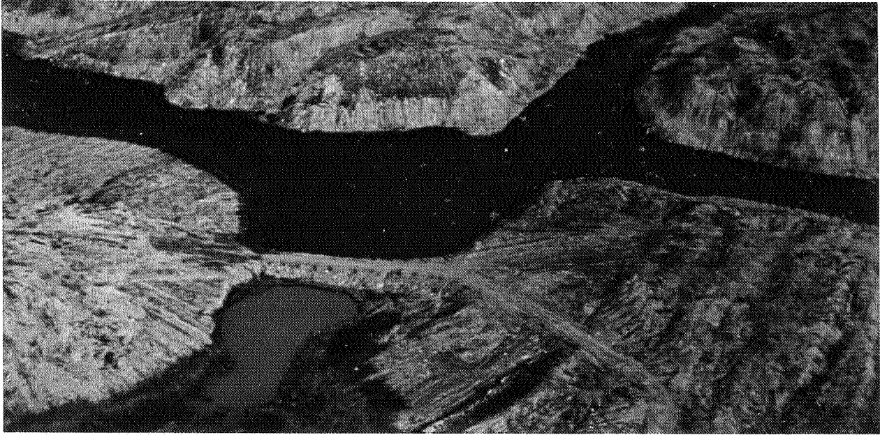
Figure 4. Strip mine reclaimed under terms of 1948 laws—some grading of spoil banks and planting.
