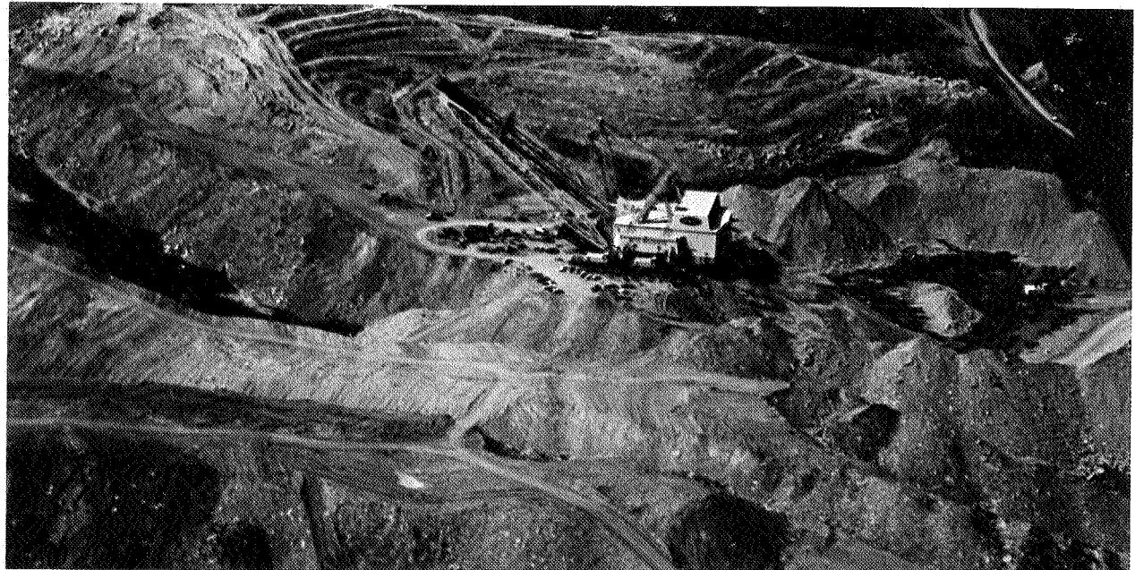
Figure 11. Air view of the Ohio Power Company mining operation with Big Muskie dwarfing nearby cars. This machine is used to strip overburden above the coal seam.
