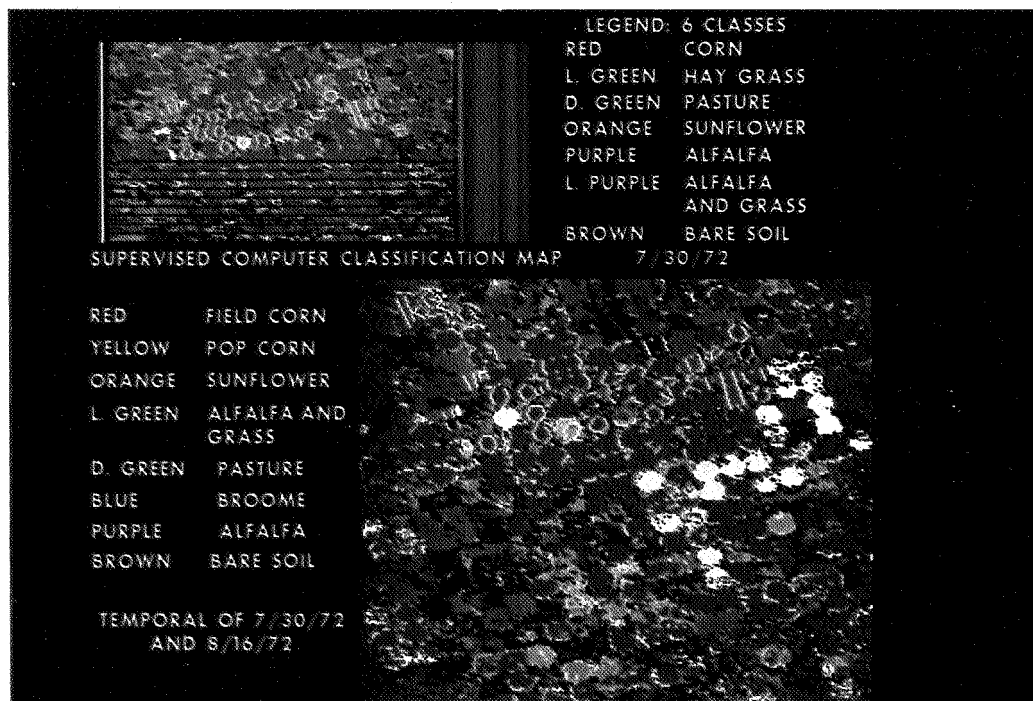
Figure 2. computer classification display of Holt County, Nebraska, test area using single-pass and two-pass data. Note that corn, popcorn, and sunflowers were separable on the two-pass data. Classification accuracies are shown at bottom of Table 2.
