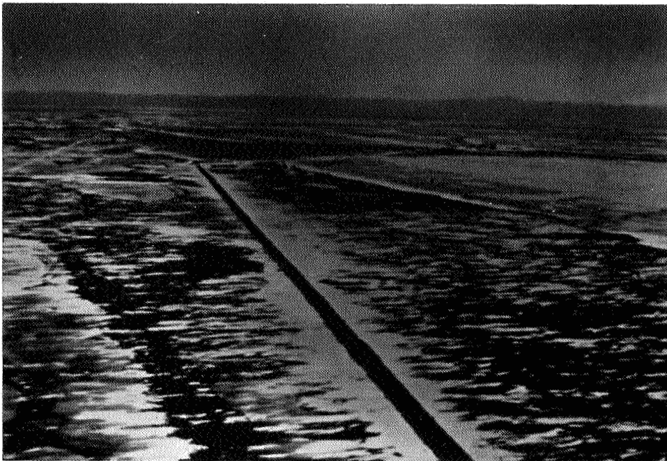
Figure 16. Aerial view of a typical North Slope gravel road showing enhanced snowmelt from dust blown downwind from the surface of the road.
