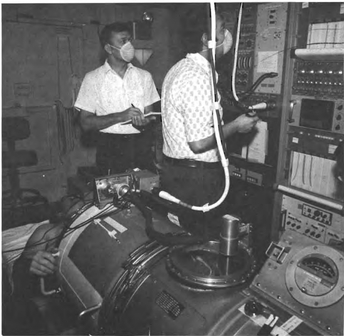
Figure 5. Skylab Mobile Laboratory. Cardiovascular facility for lower body negative pressure testing.
