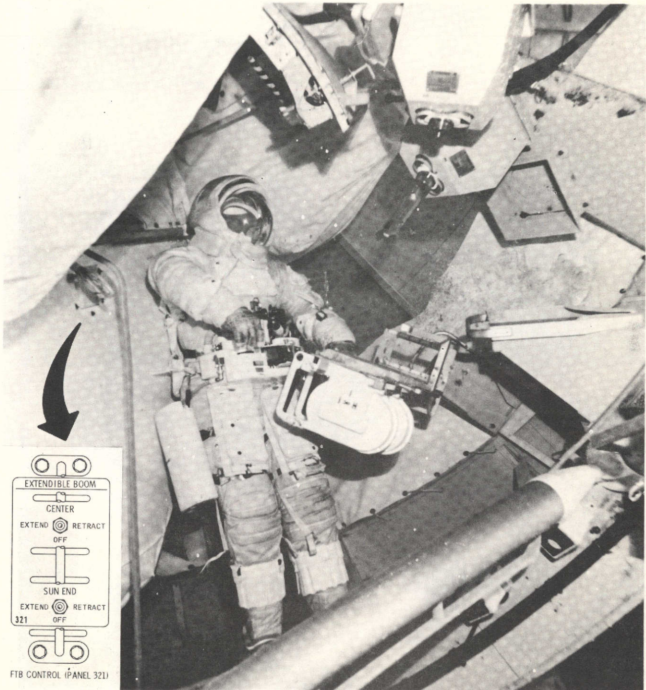
FIGURE 1.2-2: Film Transfer Boom Control Panel Location
