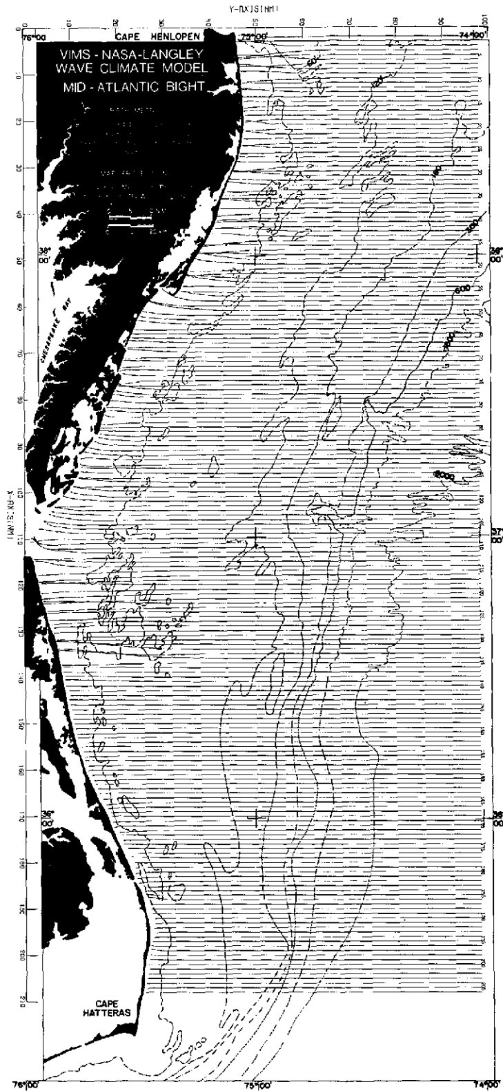
Figure B24.- Wave rays computed with following input conditions: AZ = 90°; T = 6 sec; Tide = 0.
