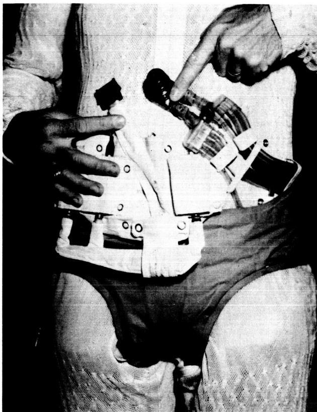
Figure 2. Urine collection and transfer assembly worn over the liquid cooling garment.
