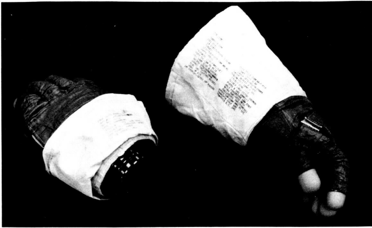
Figure 10. Extravehicular pressure gloves showing gauntlet checklist.
