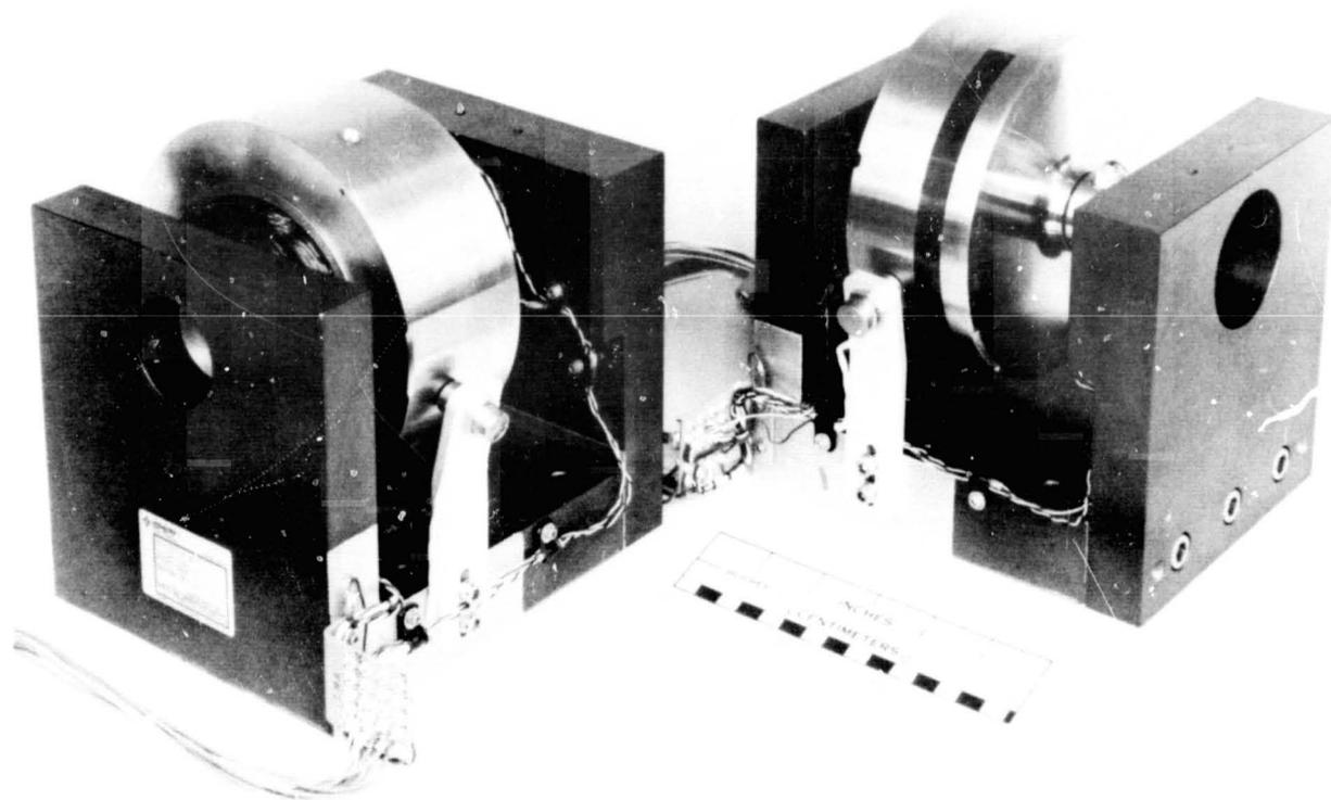
Figure 6. Momentum Wheel Fixtures in 5,000 RPM Life Test
