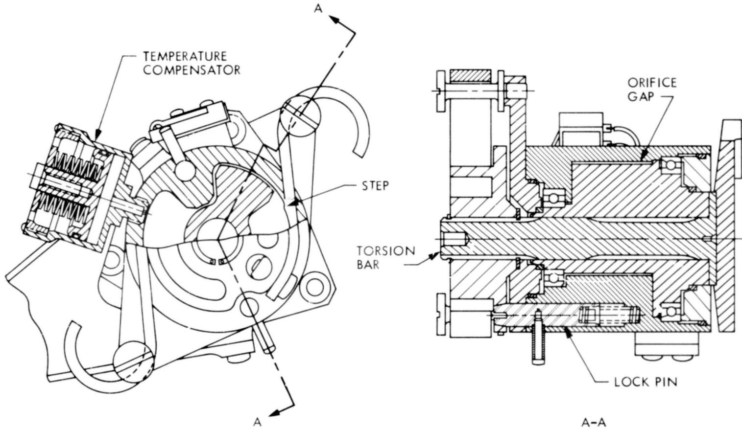
Figure 3. Rotary Vane Actuator/Damper Assembly
