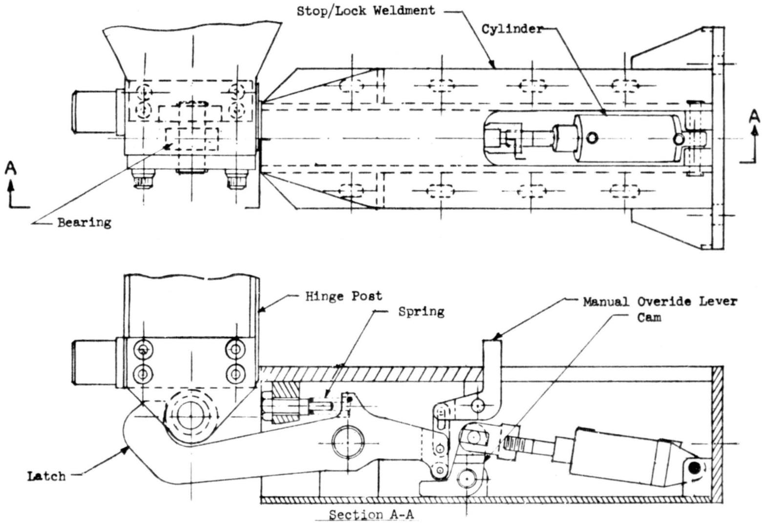
Figure 8. Stop/Lock Assembly For The Orbiter Access Arm.
