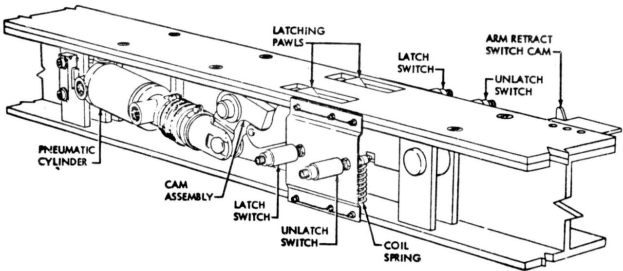
Figure 5. Arm Latch Assembly.
