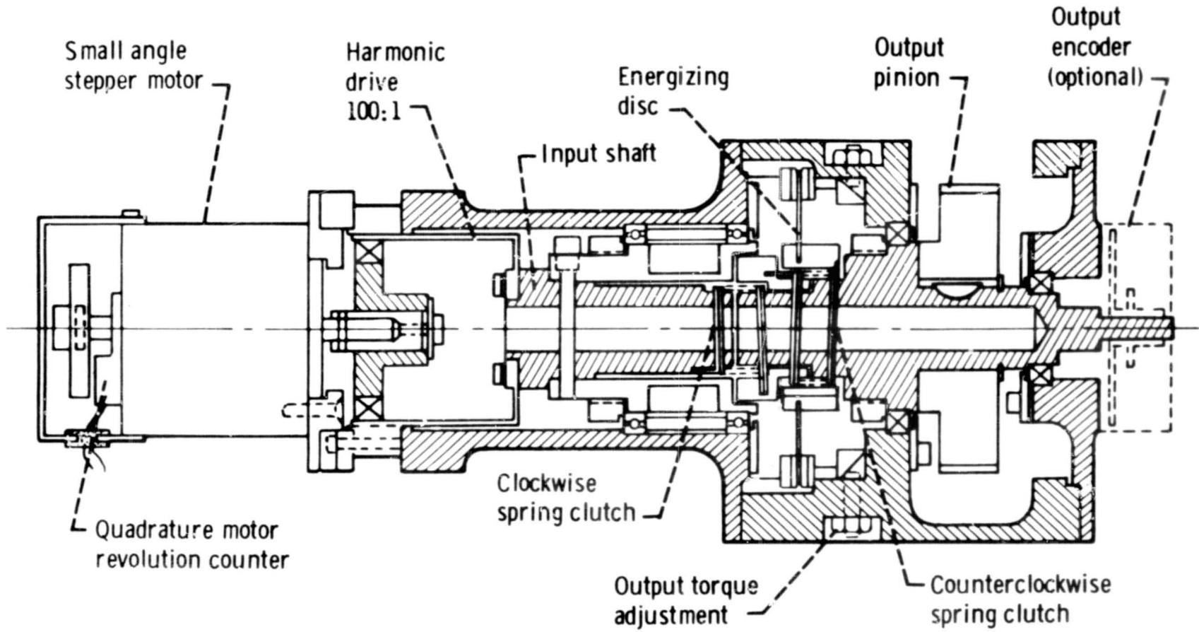
Figure 1. - Solar Array Drive Mechanism
