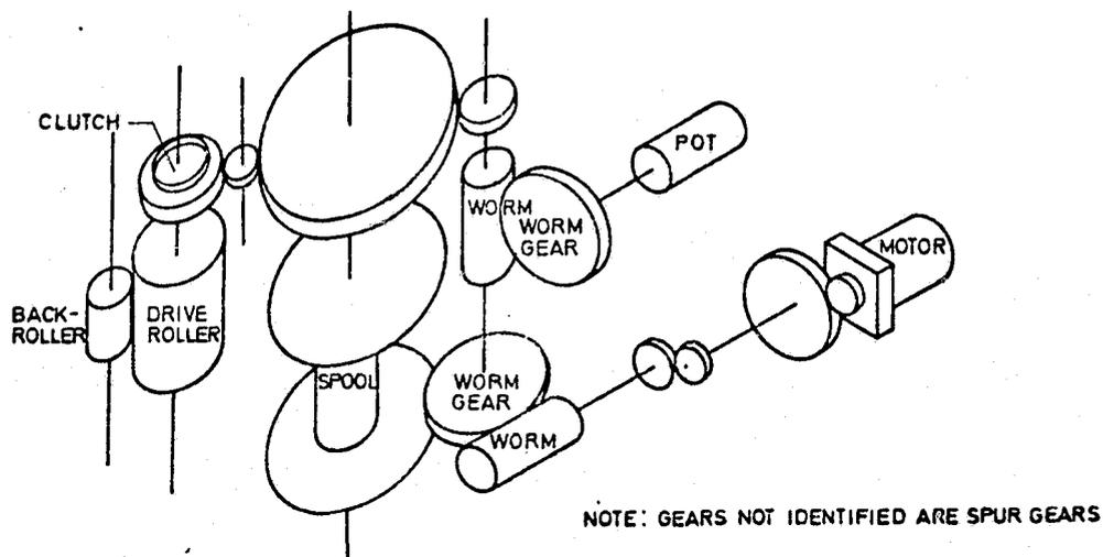
Fig. 1 Antenna drive system
