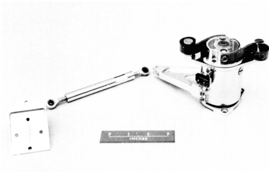
Figure 2. Actuator/Damper, Turnbuckle Linkage and Solar Panel Attach Bracket
