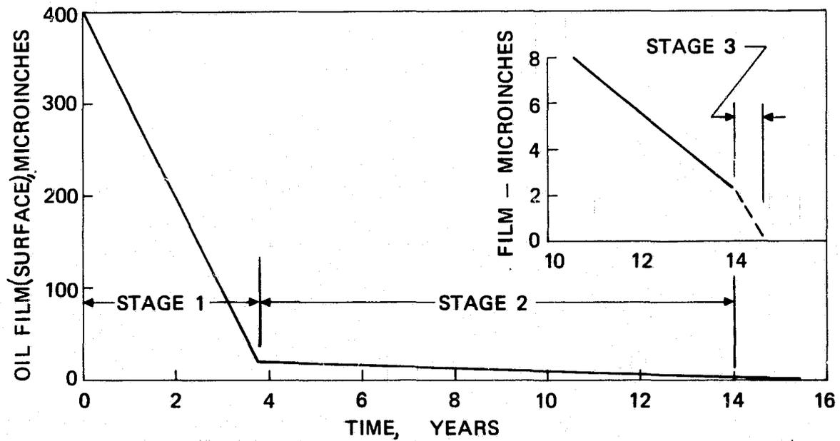
FIGURE 1. LIFE PROFILE OF OIL FILM THICKNESS IN DESPIN BEARINGS
