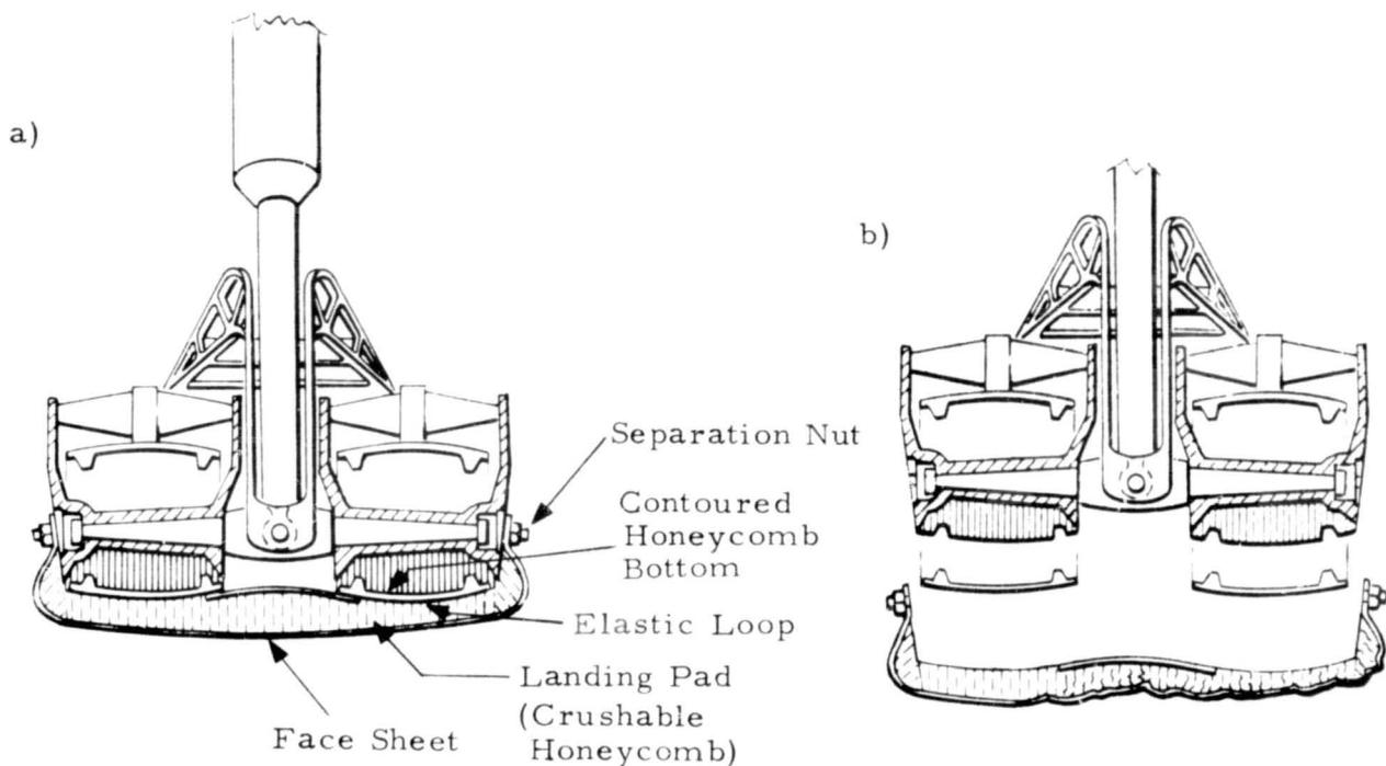
Fig. 4 - Loop protection during landing by contoured carriage bottom and crushable pad.
