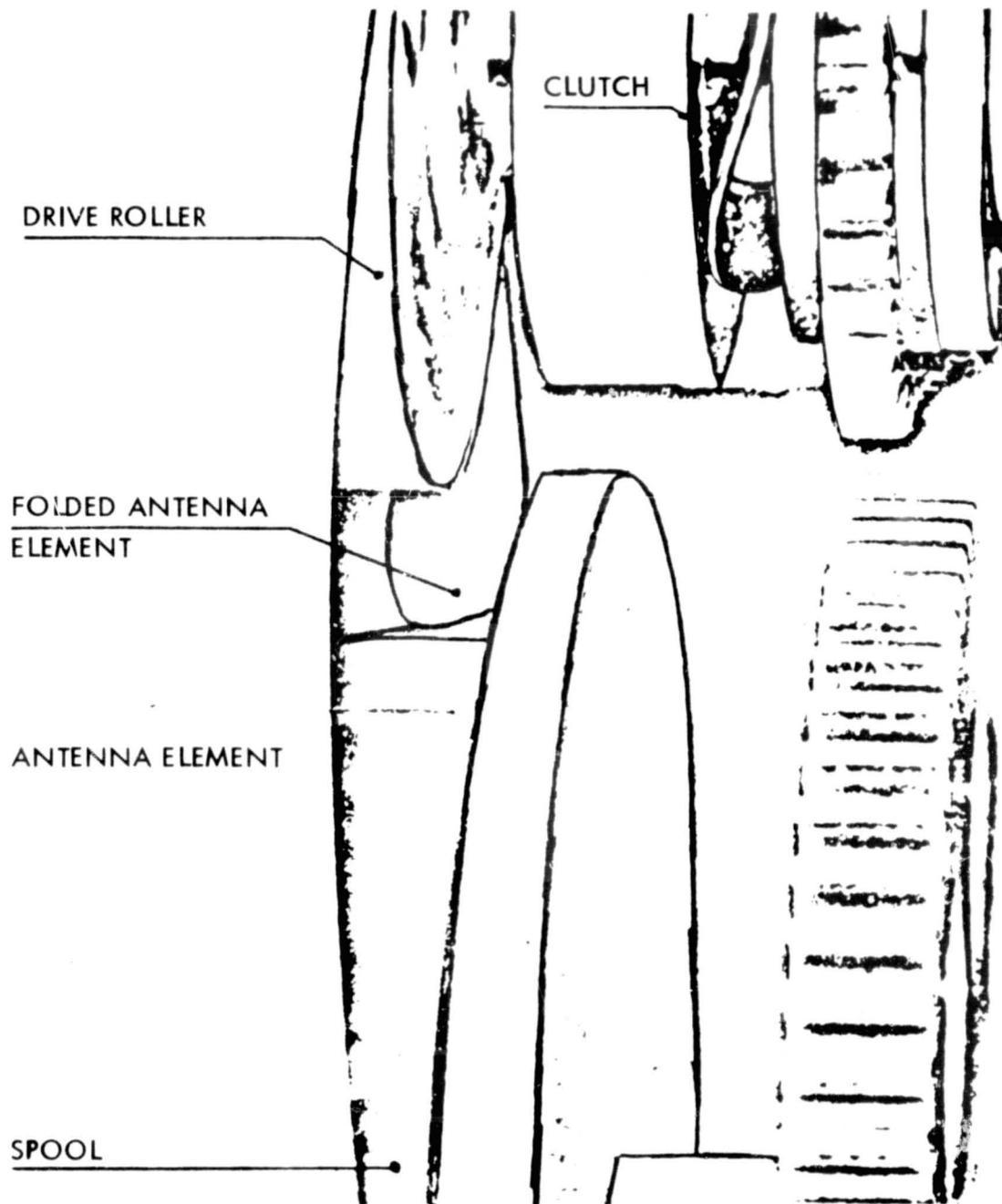
Fig. 3 Close-up view of the failed mechanism after test step 1.2
