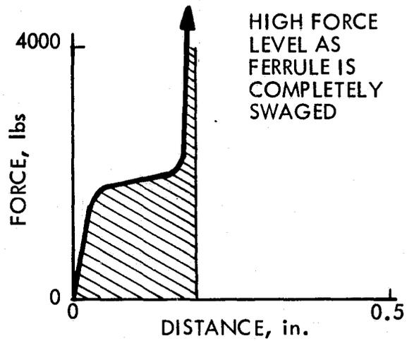
b. Characteristic of stretch tube design (high elongation material)
