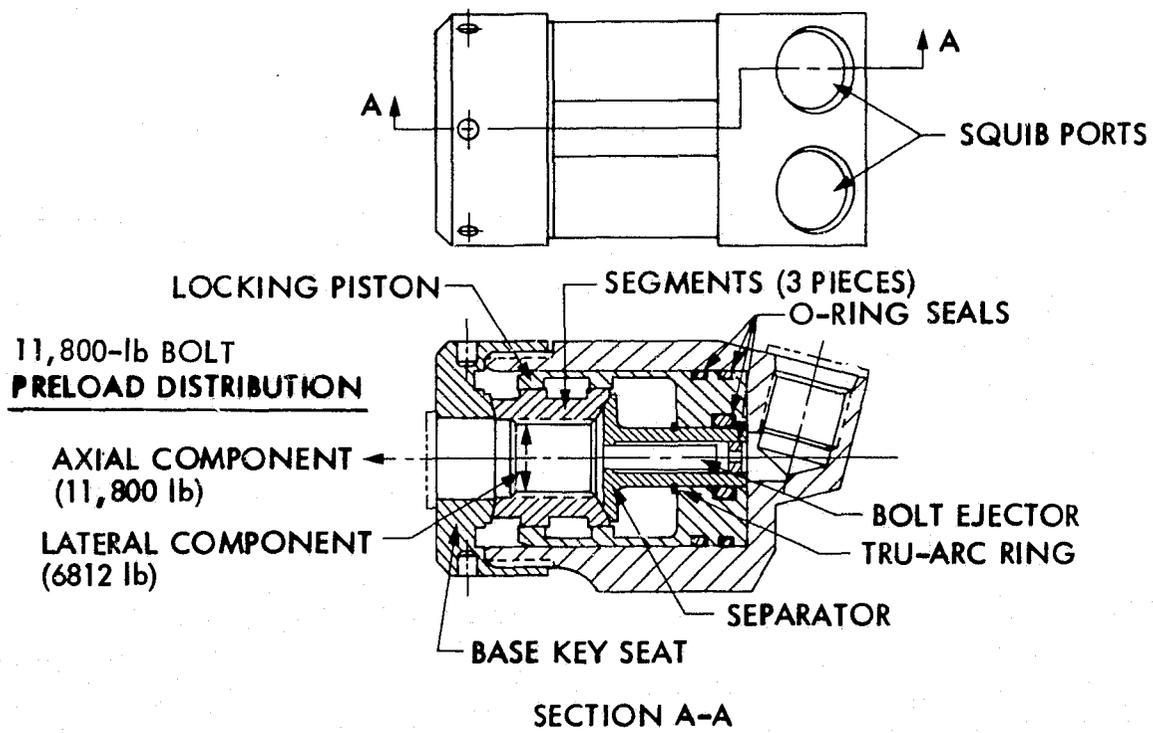
Figure 1. VO'75 release nut assembly cross section
