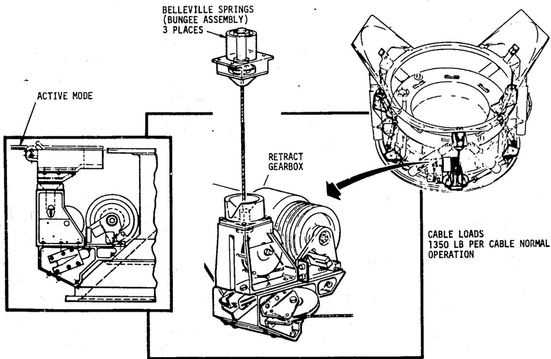
Figure 9. Docking System Guide Ring Retract System
