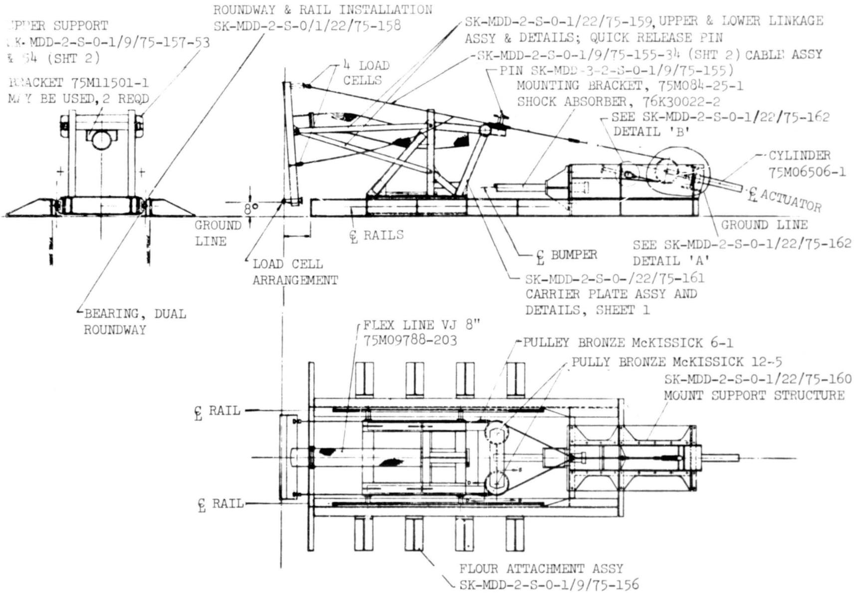
Figure 4. Assembly drawing of the TSM CVT rig
