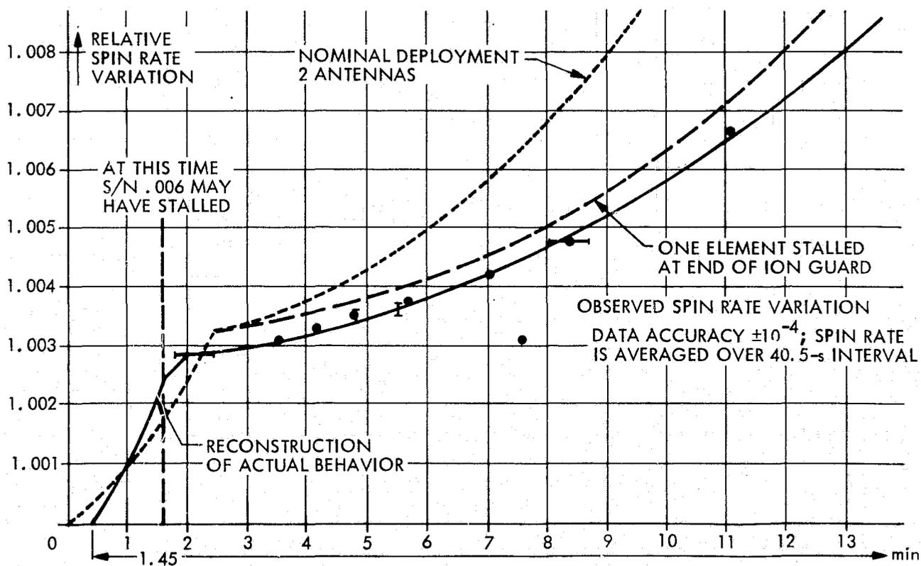
Fig. 2 Spin rate variation on board HELIOS A as function of time
