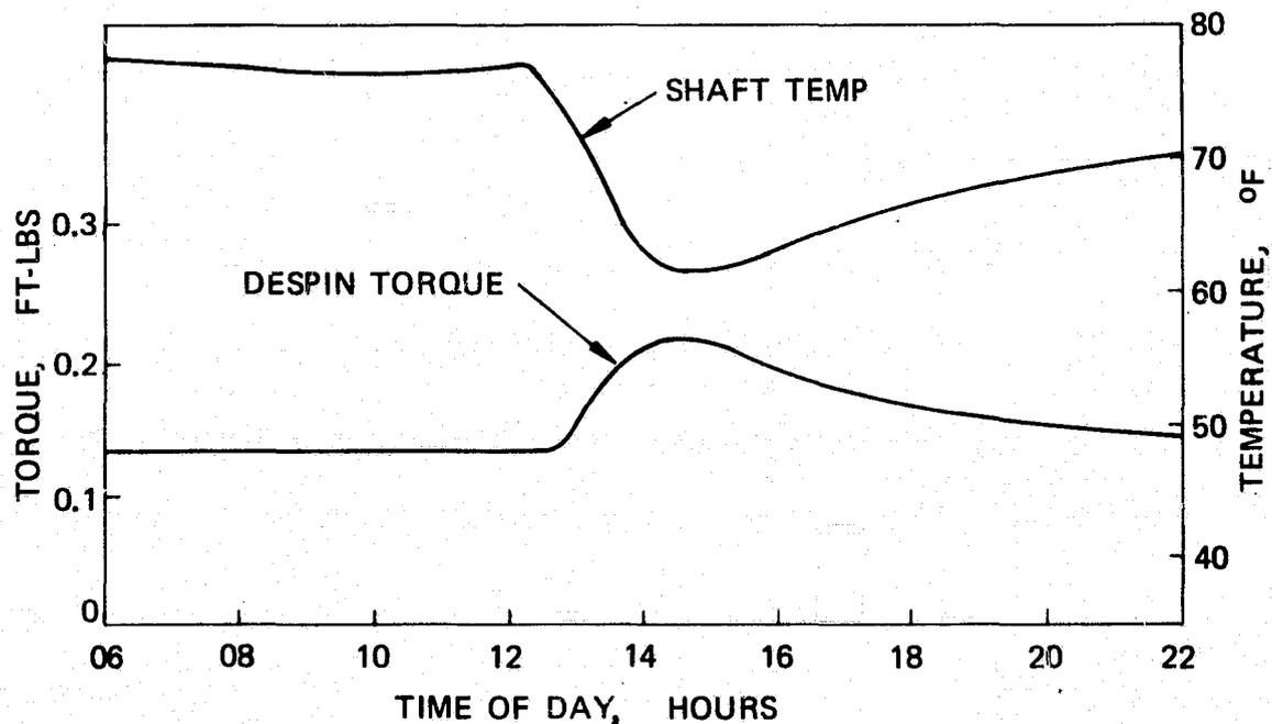
FIGURE 4. TORQUE/TEMPERATURE PROFILE OF INTELSAT IV, F-4, ON 19 MARCH 1972 DURING ECLIPSE
