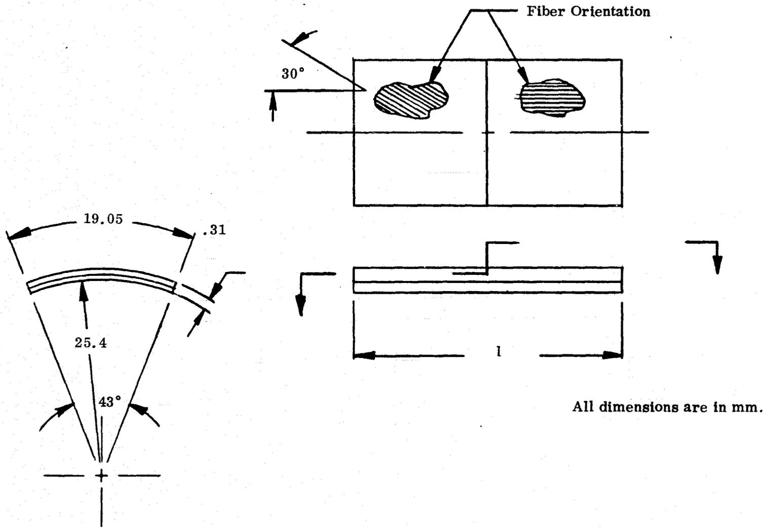
Figure 2. Flexure Hinge Configuration
