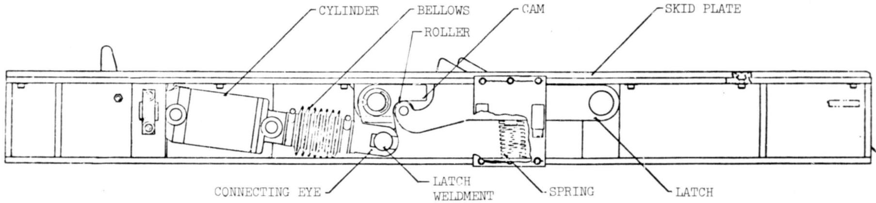
Figure 7. Arm Latch Assembly.
