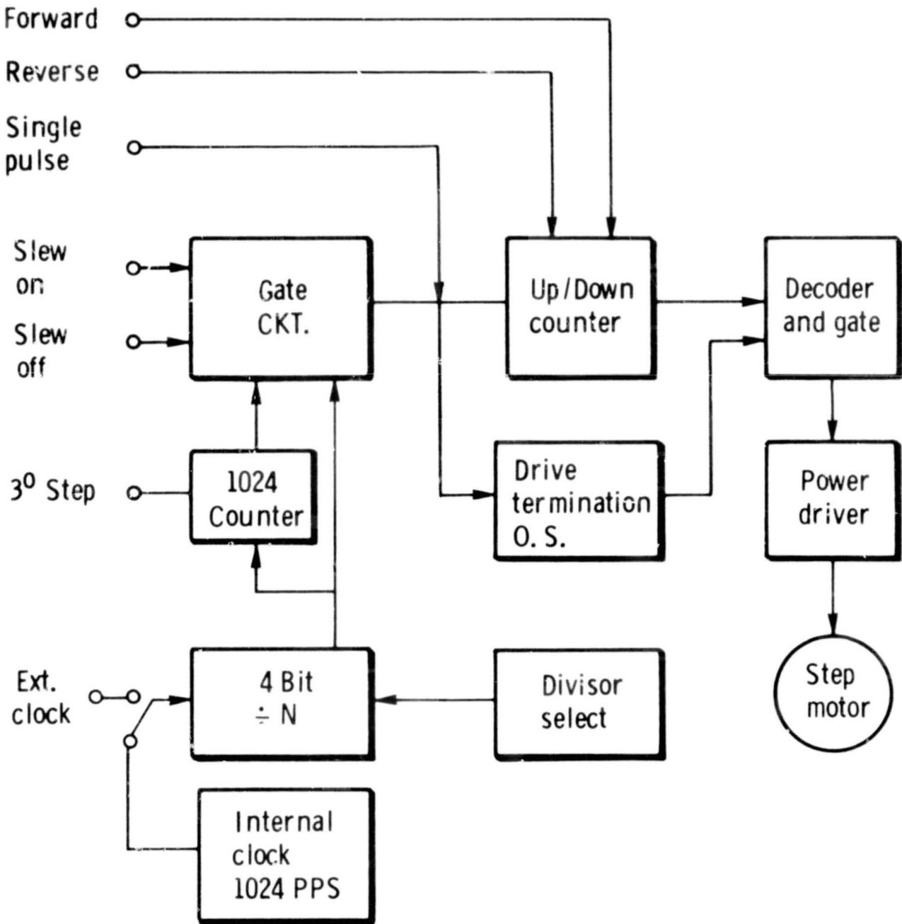
Figure 2. - Solar Array Drive Electronics
