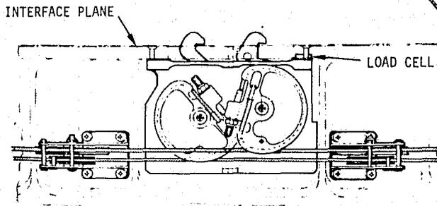
Figure 8. Docking System Structural Ring Latch
