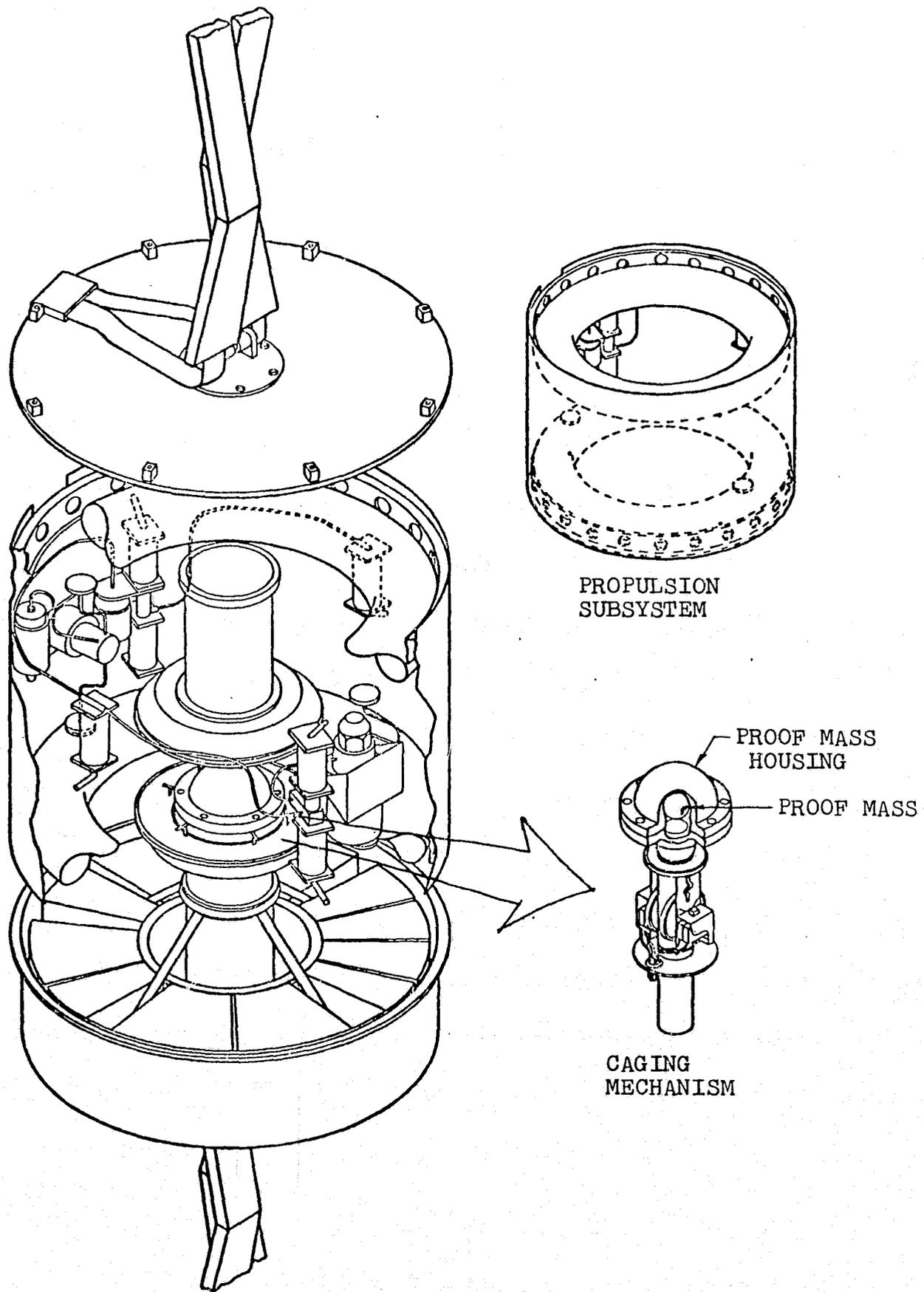
FIGURE 2 DISCOS SHOWING LOCATION OF CAGING MECHANISM.
