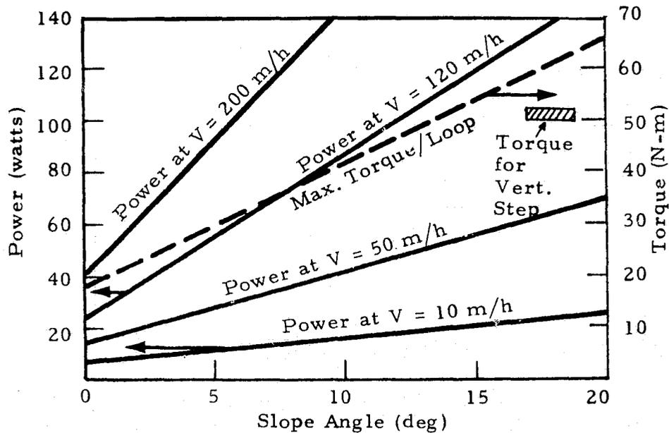
Fig. 7 - Total mobility power for mobile lander in martian loess based on loose soil tests (Ref. 8).
