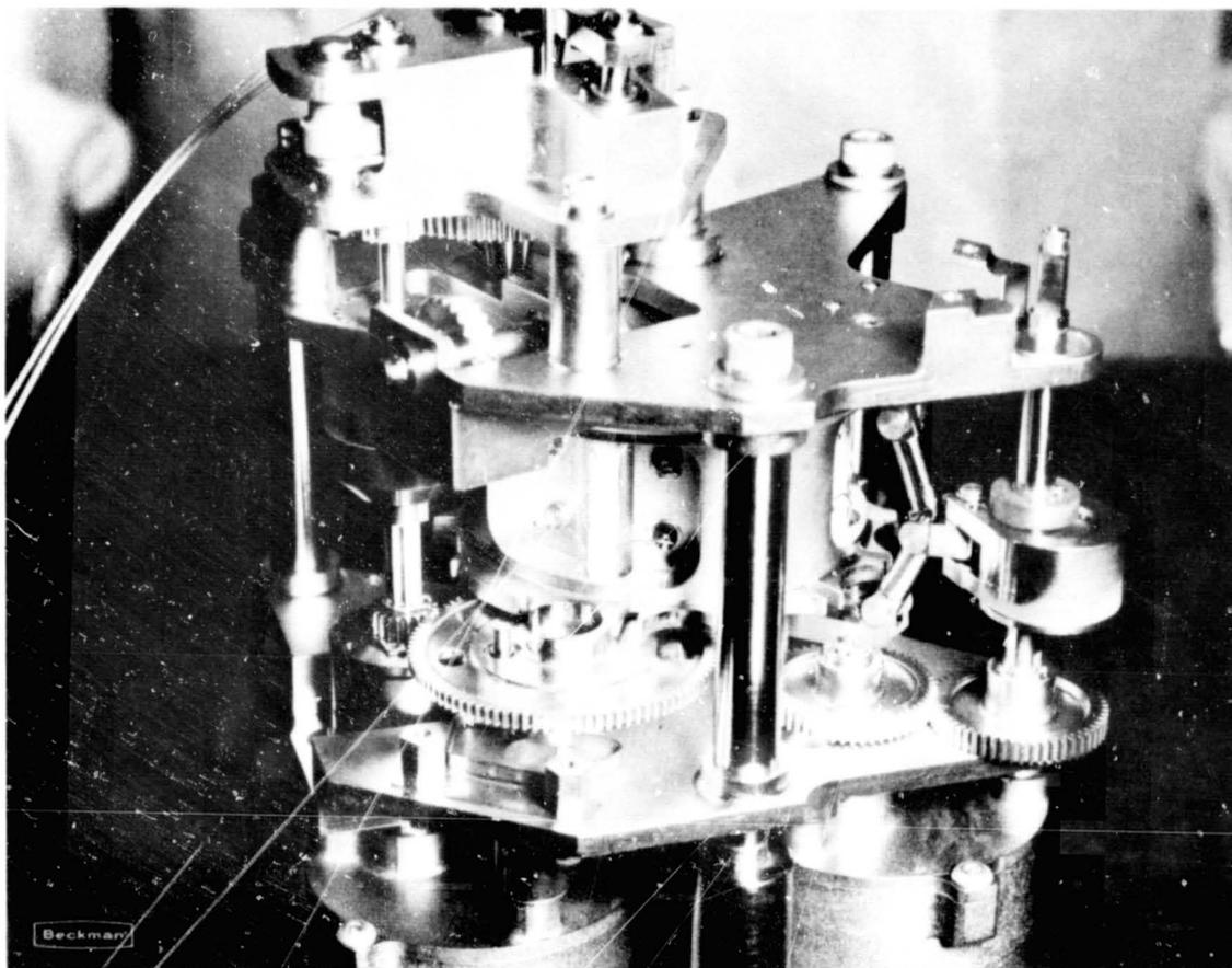
Figure 3a. Oven Carriage and Indexing Mechanism
