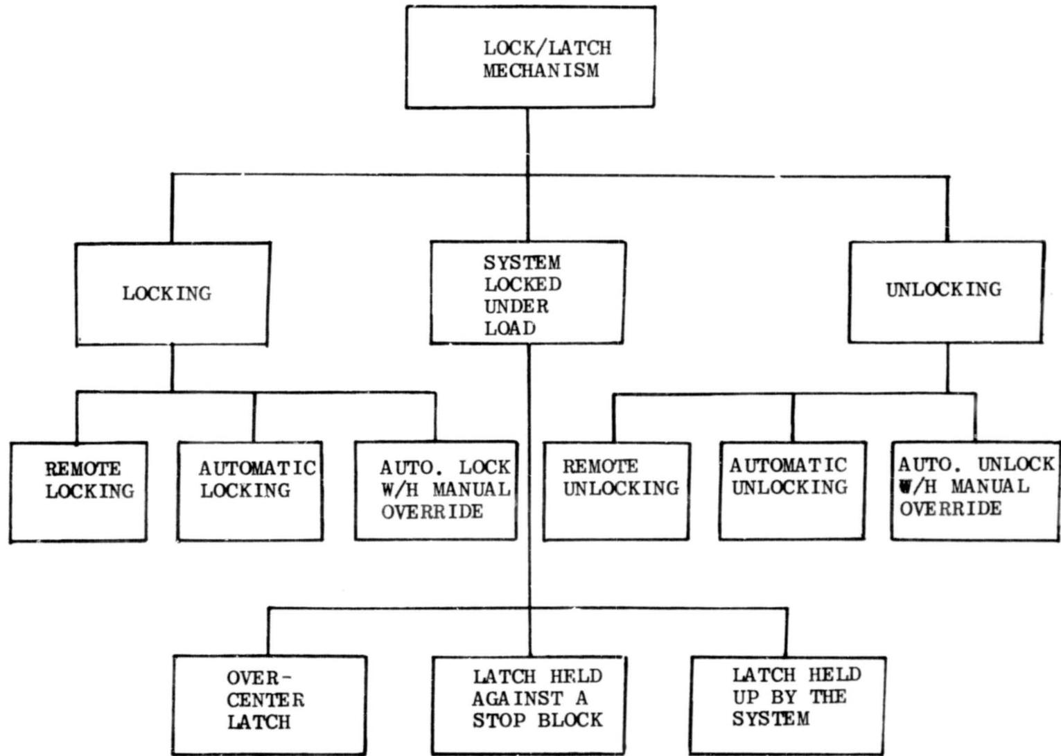
Figure 3. Locking System Tree Diagram.
