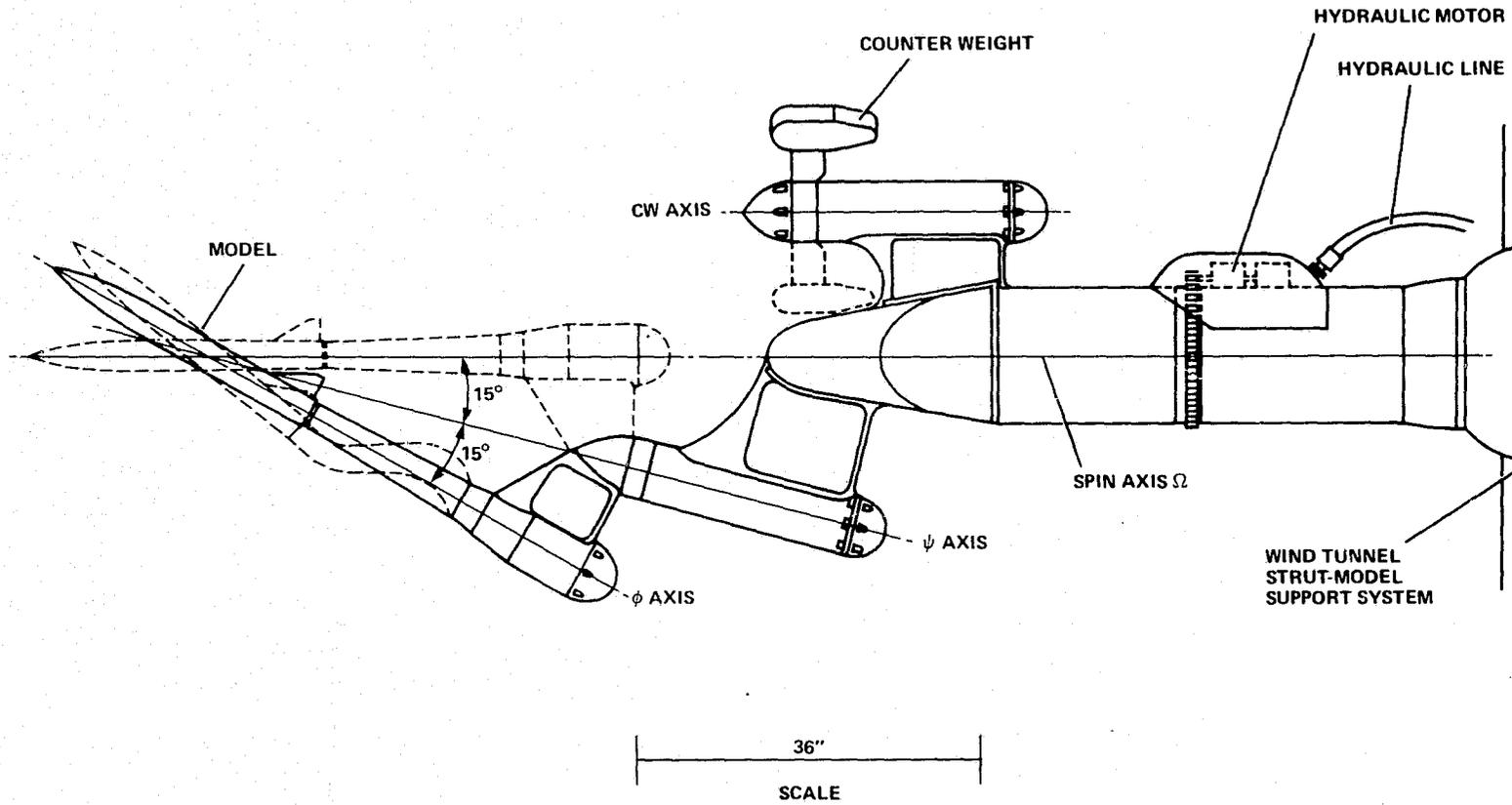
Figure 2. Axis definition and overall view of the "Dynamic Stability Rig"
