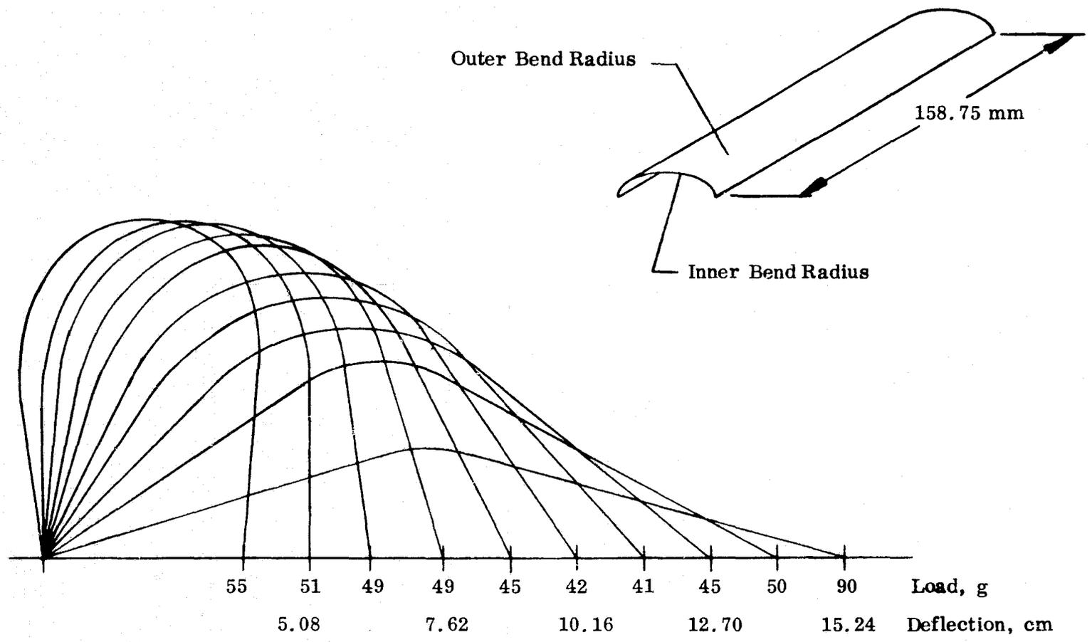
Figure 5. Flexure Hinge Force vs Deflection Characteristics
