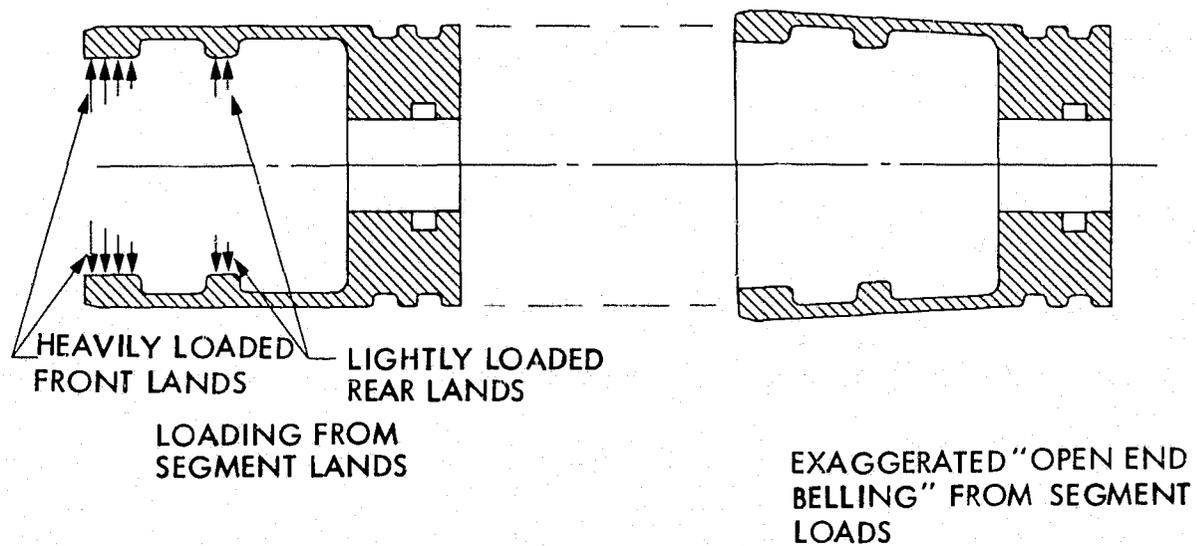
Figure 3. Piston cross sections showing loading and belling
