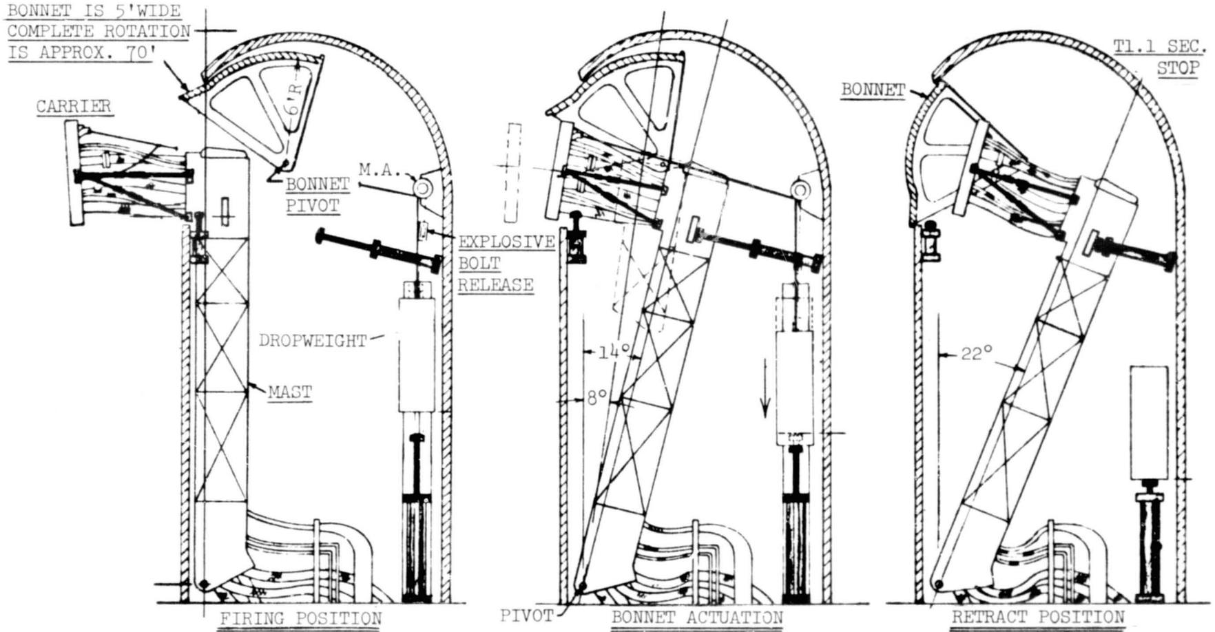
Figure 2. The basic TSM operation and components
