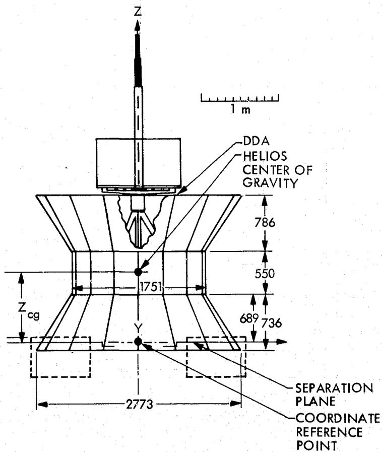
Fig. 2 HELIOS spacecraft dimensions
