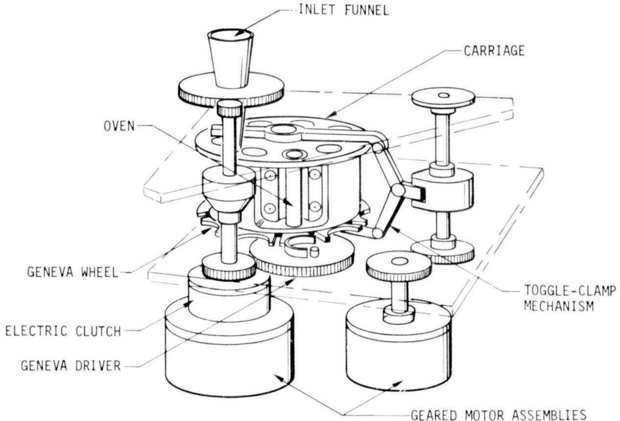
Figure 1a. Diagram of Surface-Sample Loading and Pyrolyzing Assembly (SSLPA).
