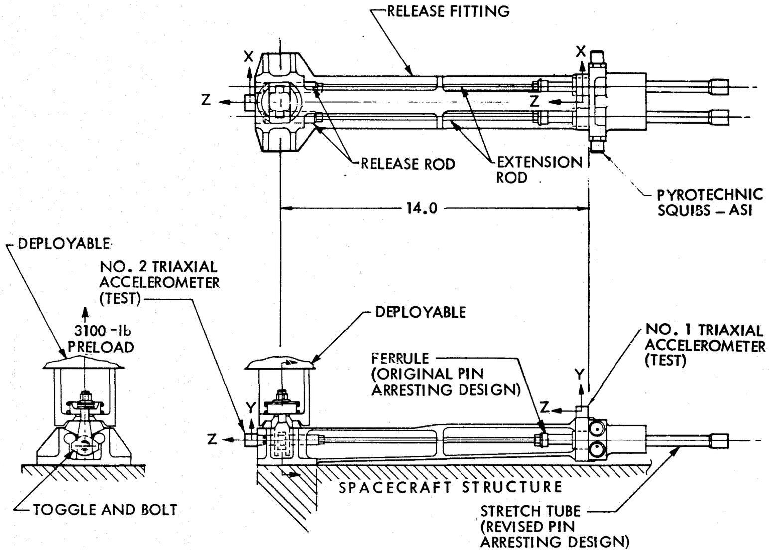
Figure 1. Release mechanism design
