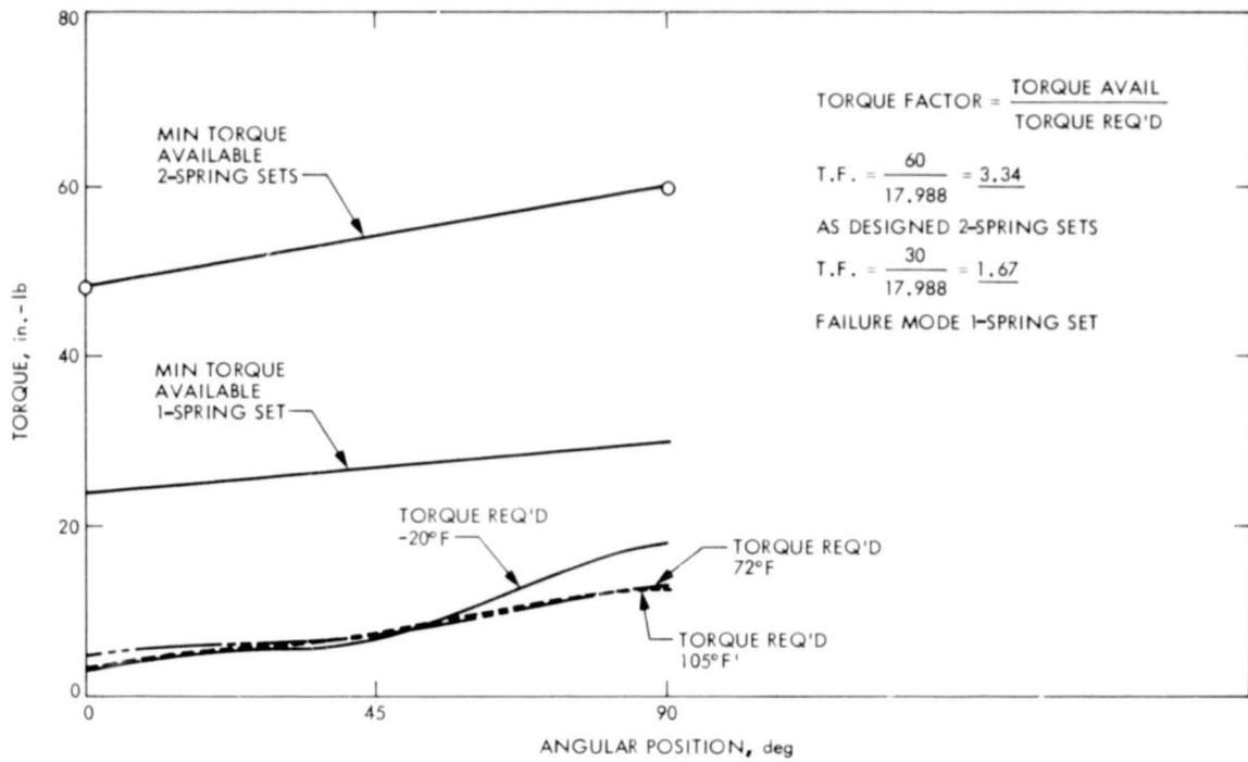
Figure 1. Input Torque Available and Resistive Torques Compared to Panel Angular Position
