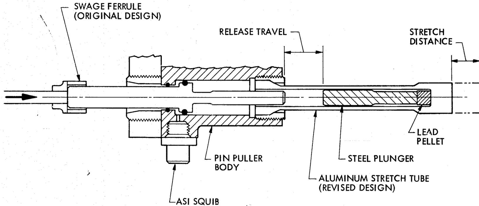
Figure 2. Details of pin arresting mechanism showing original (ferrule) and selected (stretch tube) designs
