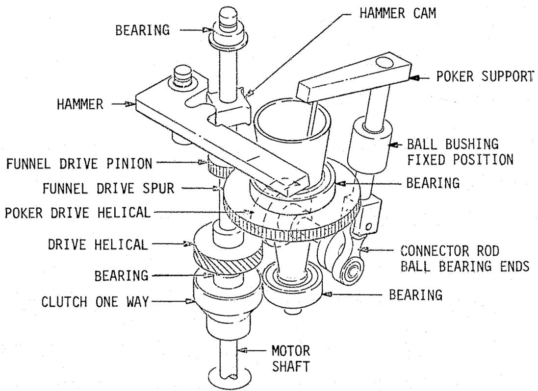
Figure 2. Soil Loader Mechanism
