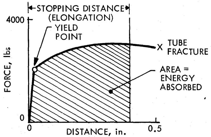
c. Characteristic of stretch tube design with addition of lead pellet (low modulus material) to reduce initial steep force rise.
