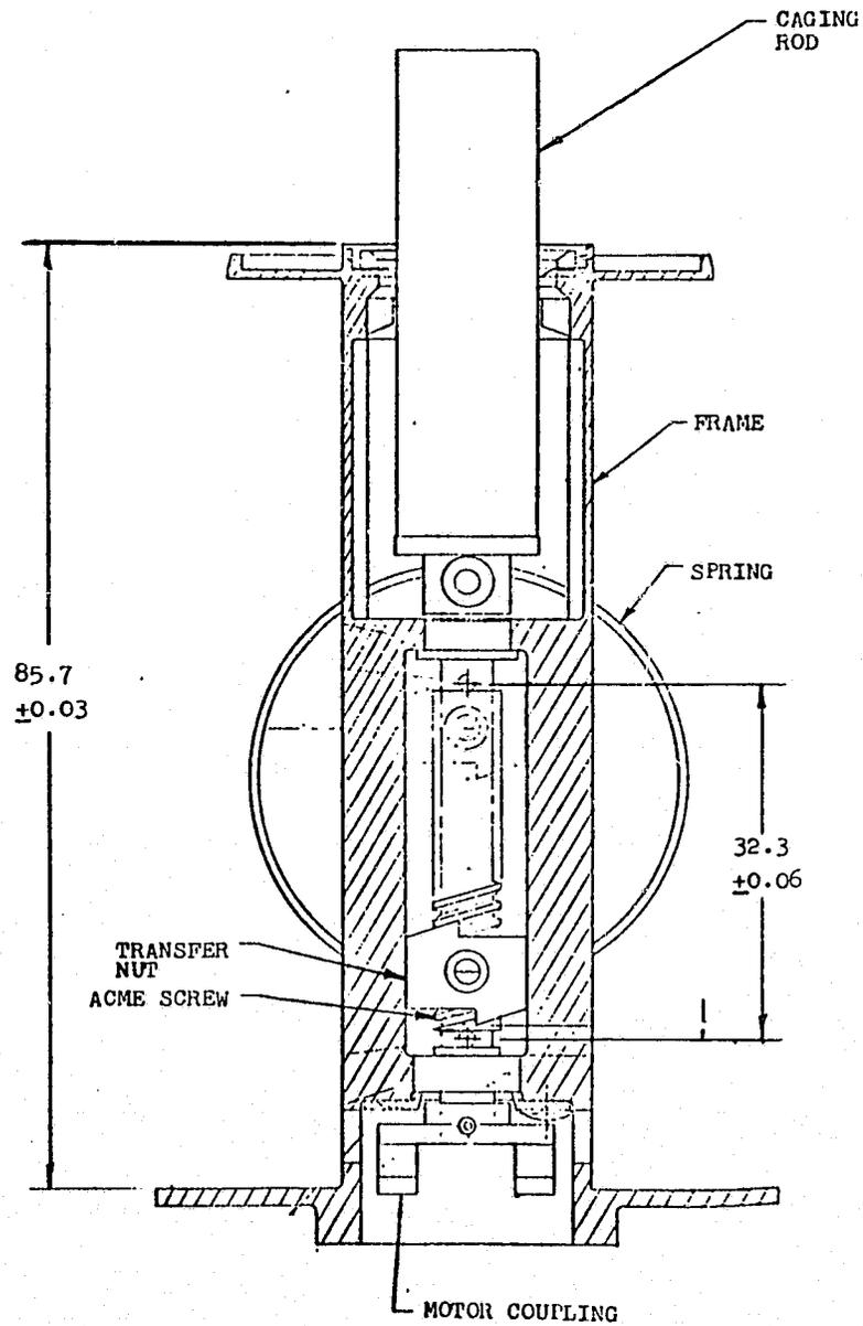
FIGURE 3 CROSS SECTION OF CAGING MECHANISM.
