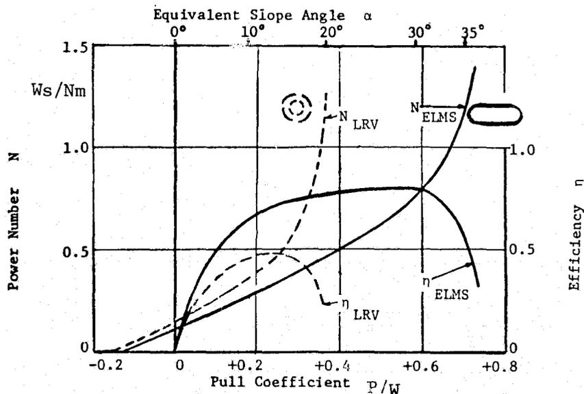
Fig. 8 - Comparison of power requirements and slope climbing capability of LRV-wheels (82 cm dia, 254 N load) and elastic loop mobility systems, "ELMS" (160 cm long, 46 cm high, 685 N load) tested in loose lunar soil simulant at WES (Refs. 8, 9); power number  $N = \text{energy required (Ws) per newton load and per meter traveled}$ ; efficiency  $\eta = \text{pull} \times \text{speed} / \text{input energy}$ .
