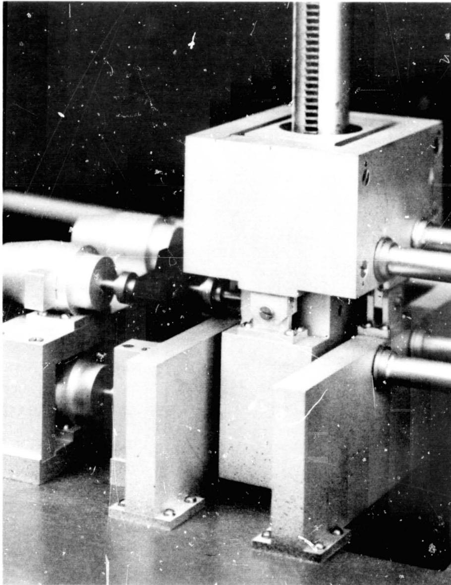
Figure 2. Vertical drive pinion carrier of Vertical Motion Simulator model
