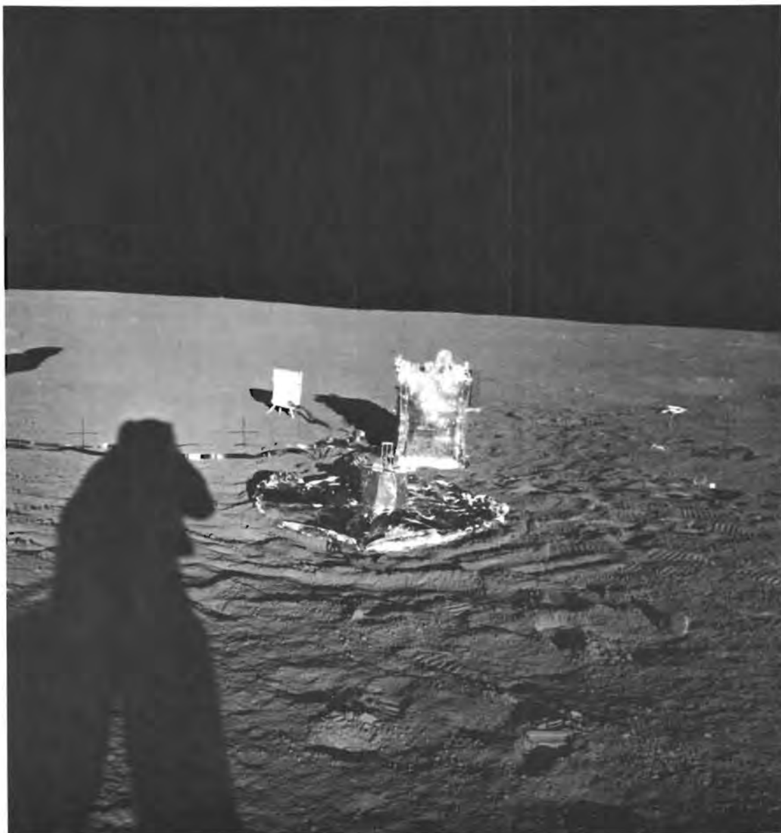
Figure 3-5.- Passive seismic experiment and the experiment central station in the foreground with the undeployed suprathreshold ion detector experiment in the background.
