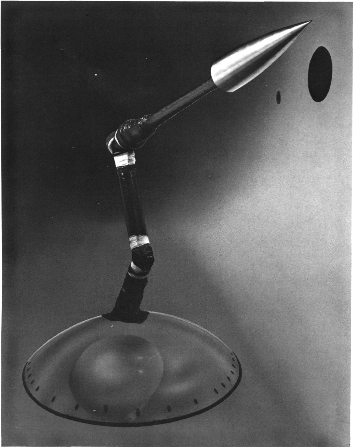
(b) Installation of \ell/d = 3.5 tangent ogive on floor-support system, \alpha = 0^\circ to 45^\circ .
