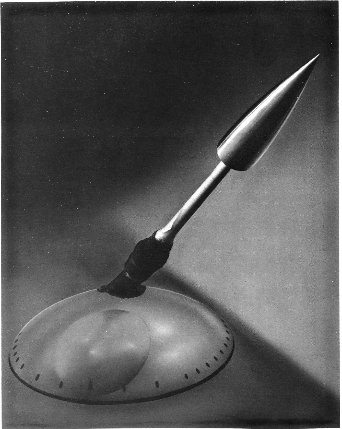
(c) Installation of \ell/d = 3.5 tangent ogive on floor-support system, \alpha = 36^\circ to 88^\circ .
