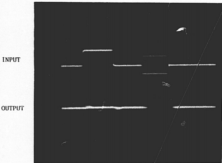
Fig. 8 Demonstration of Using Canceller Type Comb Filter for MTI Radar Applications X scale: 10 \mu sec/division
