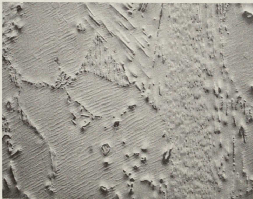
Figure VI-17. Primary bismuth dendrites and secondary MnBi/Bi eutectic within ground-based sample (325X).
