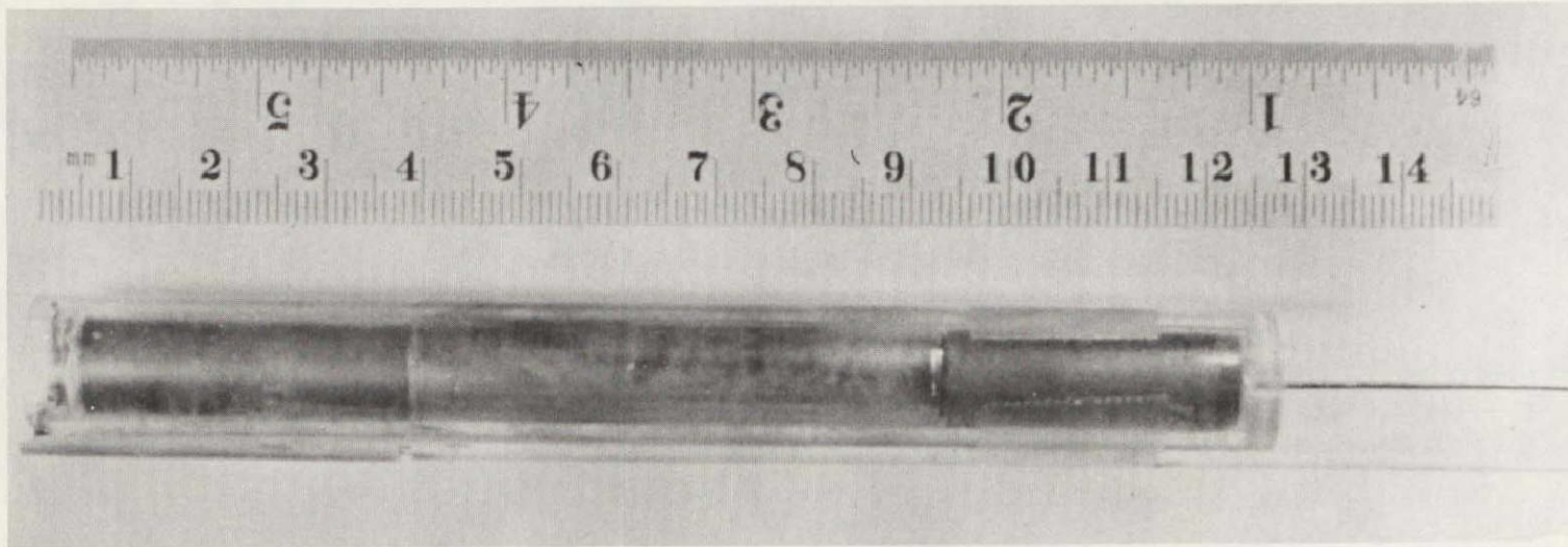
Figure V-16. Encapsulated germanium crystal used for simulation tests (the ampoule in the configuration shown was used for all ground-based and flight experiments).
