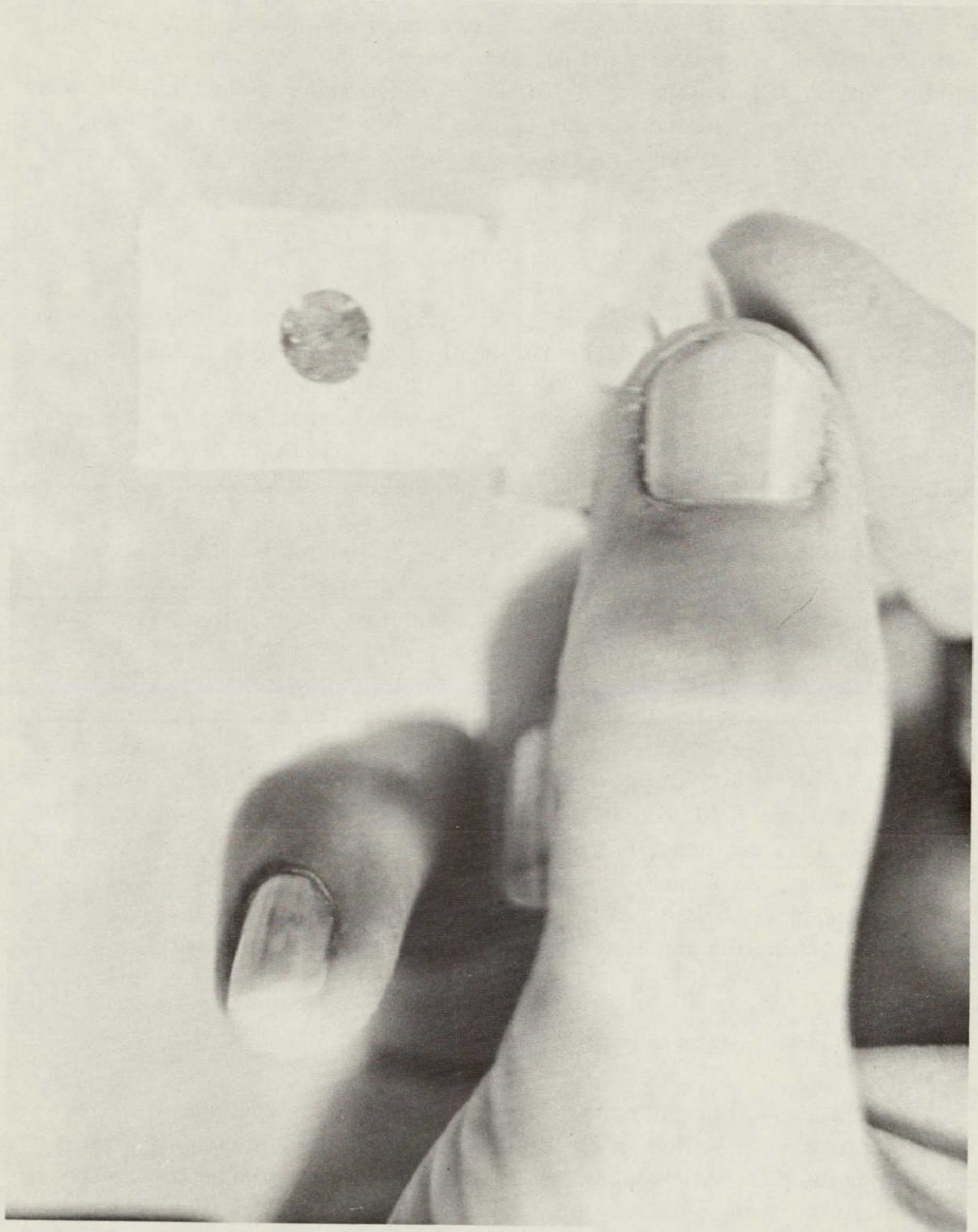
Figure I-7. Sample slide containing frozen sample (these samples were kept at liquid nitrogen temperature until processed).
