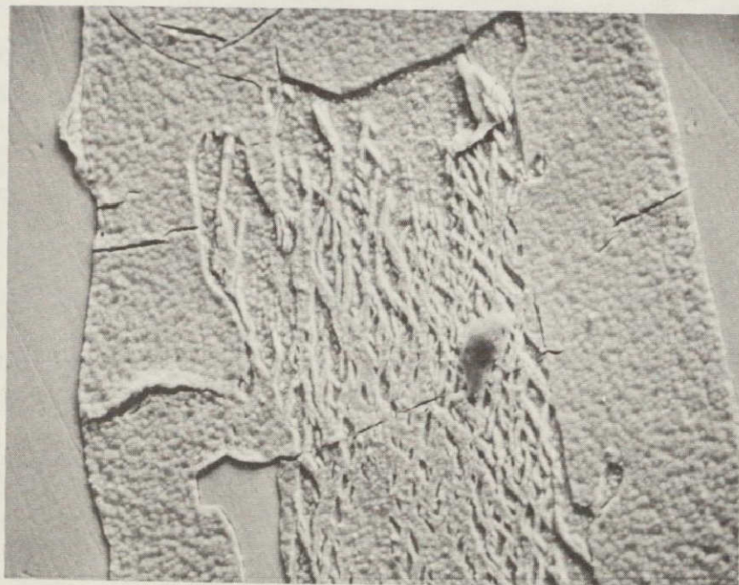
Figure VI-14. Primary MnBi crystallite showing discretely different morphological regions (900X).
