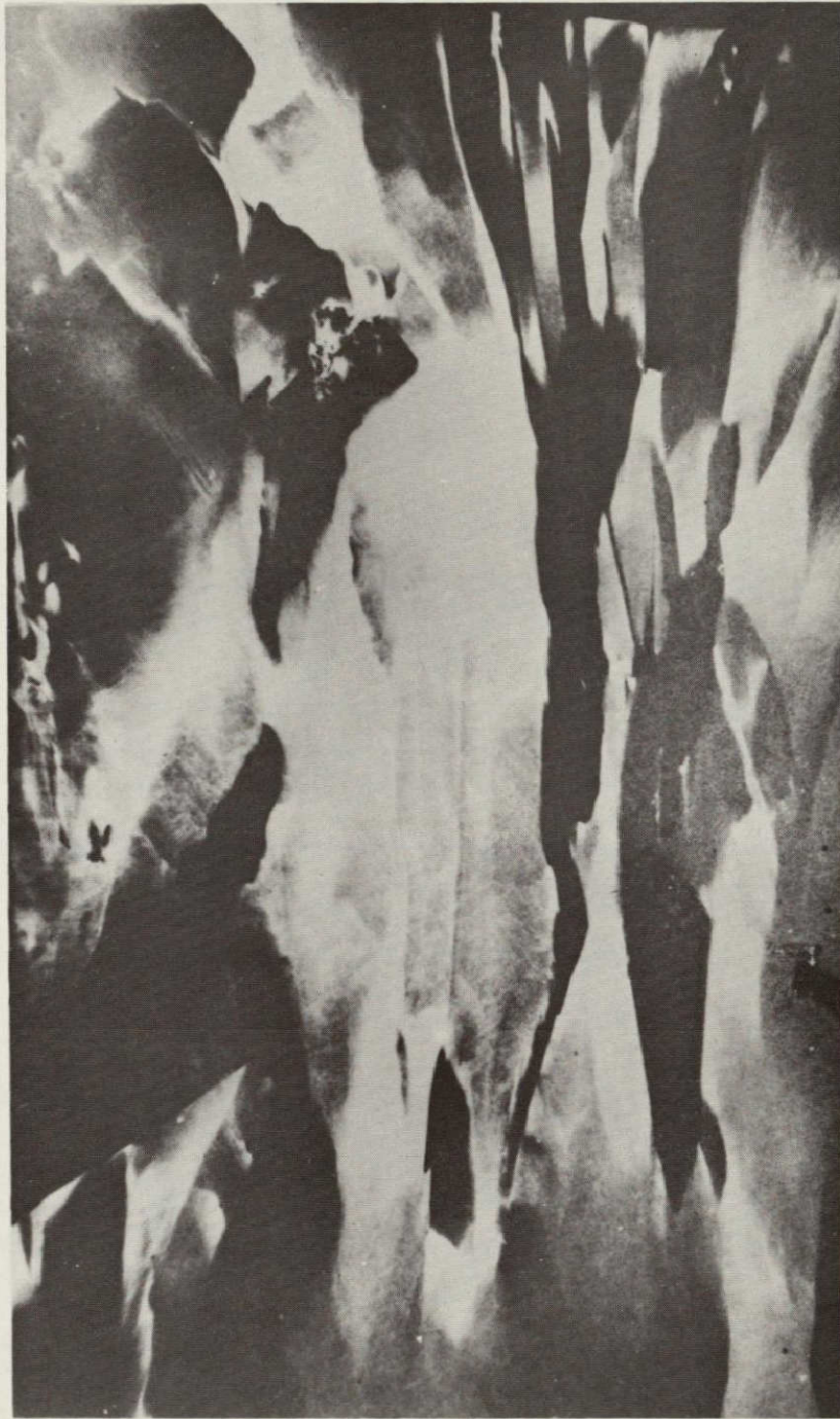
Figure IX-10(a). X-ray topograph of the longitudinal section of crystal MA-150-07 (12X).
