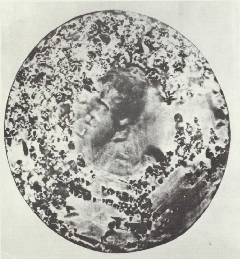
Figure IX-20(c). X-ray topograph of the seed surface adjacent to the region of crystal MA-150-17 shown in Figure IX-19 (12X).
