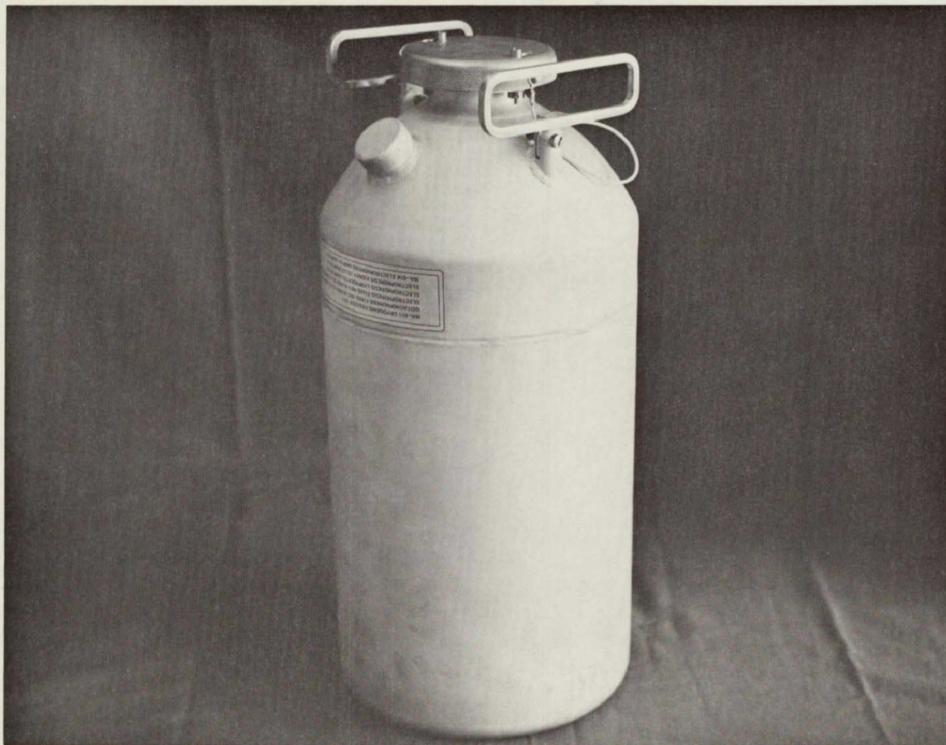
Figure I-4. CF used to transport samples to orbit and to return frozen columns to Earth (note tether cord on cap to prevent separation during orbital operations).
