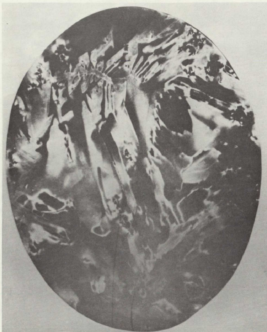
Figure IX-8(b). X-ray topograph of the cross section of the initial region of crystal MA-150-18 (12X).
