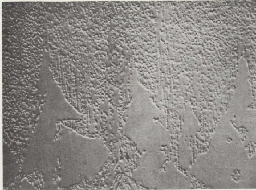
Figure VI-18. Transition from dendritic to coordinated growth within ground-based sample (75X).
