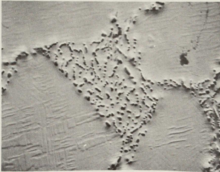
Figure VI-16. Primary bismuth dendrites and secondary MnBi/Bi eutectic within ground-based sample (650X).
