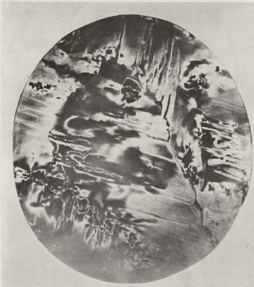
Figure IX-8(a). X-ray topograph of the cross section of the initial region of crystal MA-150-07 (12X).
