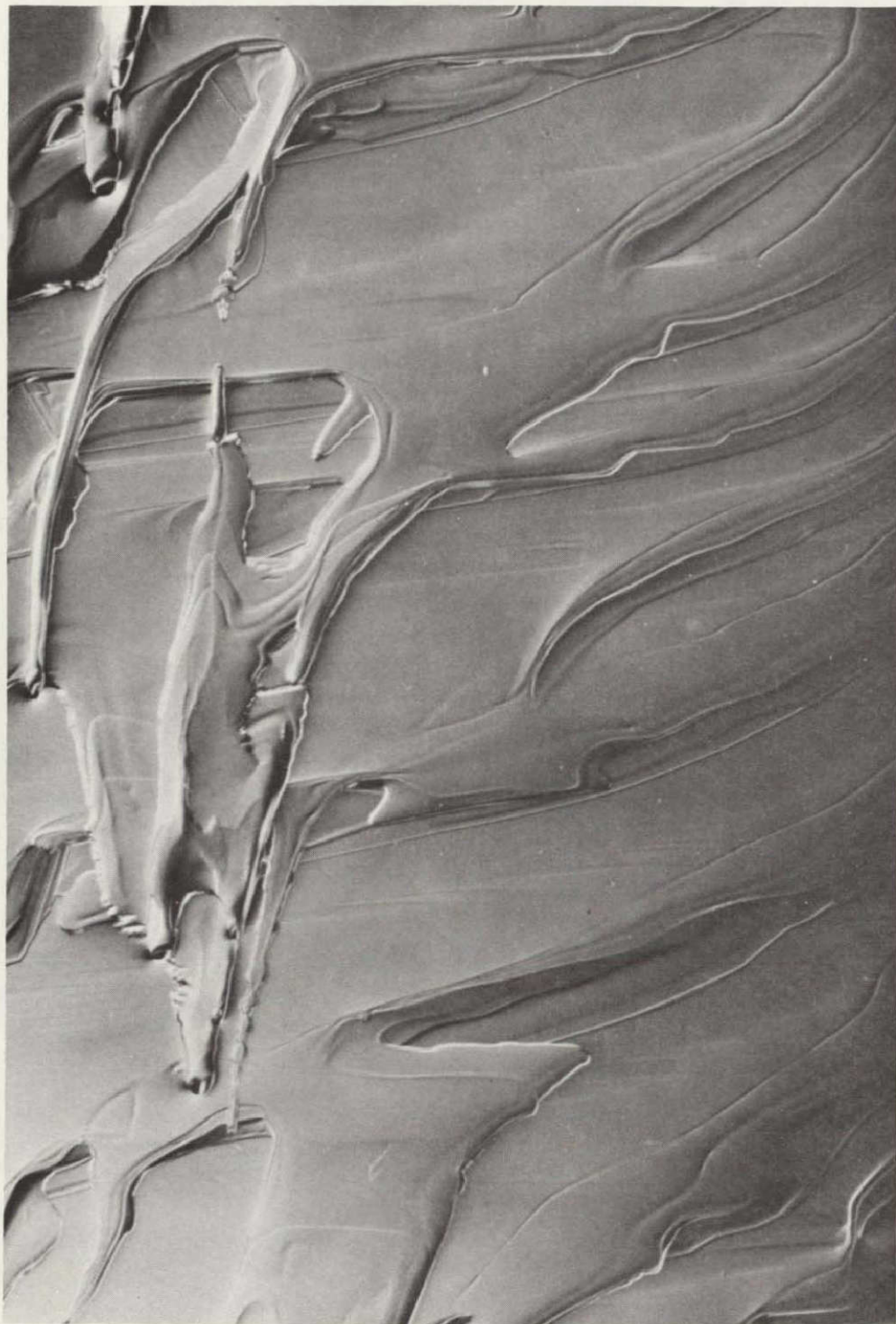
Figure V-32. Advanced stages of interface breakdown observed in the \langle 111 \rangle germanium crystal regrown during the final ground-based test (GBT 3).
