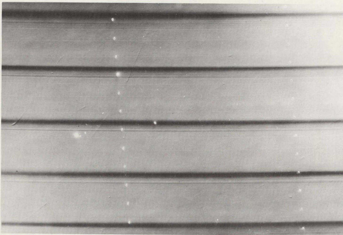
Figure V-20. Interface demarcation achieved by current pulses of 15 A and 60 ms duration at a repetition rate of 4 s (the crystal shown was pulled, by the Czochralski technique, during ground-based testing).
