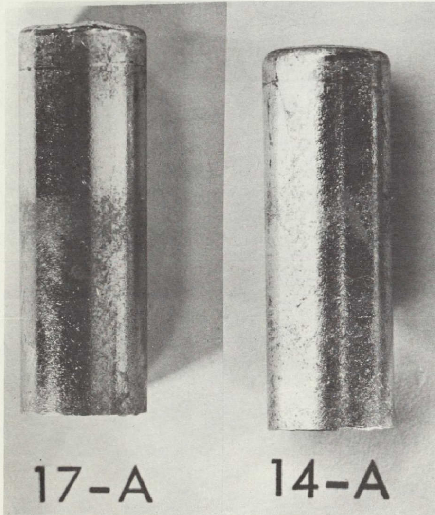
Figure 16. Photograph of ground base specimens 17 A and 14 A which were located in the 923 K and 723 K temperature zones of the multipurpose furnace, respectively. Samples solidified from the bottom to top in ampoules with nonwetting walls. Samples are approximately 1-cm diam.
