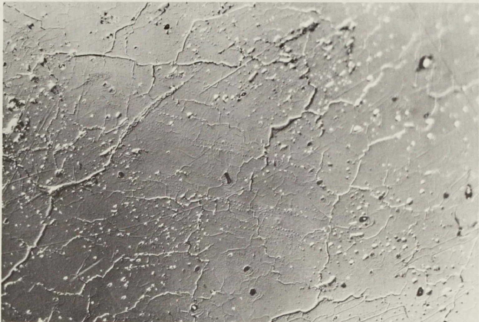
Figure V-4. Irregular ridge patterns on the surface of the \langle 100 \rangle germanium crystal regrown in space (180X).
