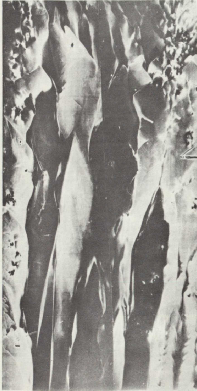
Figure IX-10(b). X-ray topograph of the longitudinal section of crystal MA-150-18 (12X).
