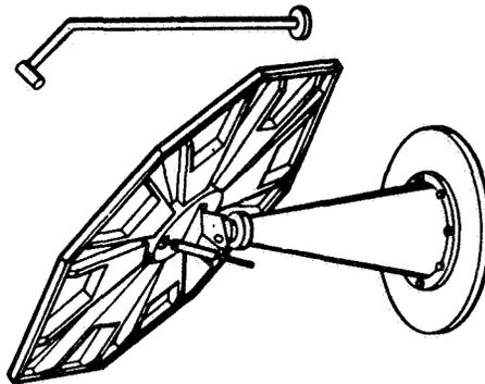
Figure 5. Pilot plant heliostat concepts.
