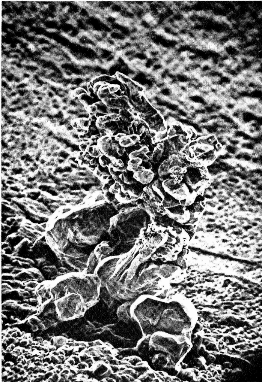
Figure 6. Silver from the electrolyte that is redeposited on the cathode can because of an excess ripple or by a strong direct voltage of the proper polarity.
