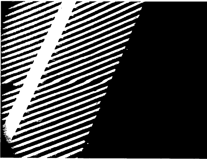
Figure 2. Scanning electron microscope picture at a magnification of 250 X of a vertical junction cell broken perpendicular to the grooves.
