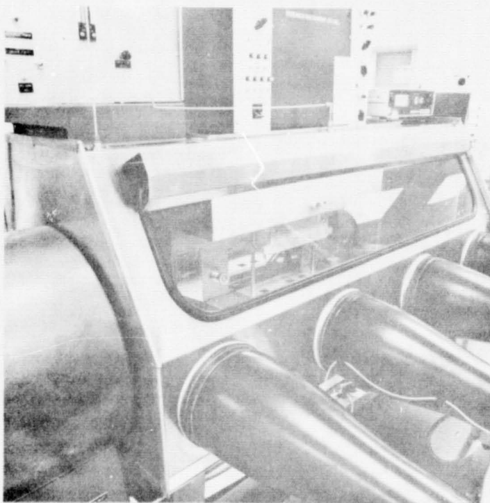
Figure 2 Gradient Sealer Enclosed with Attached Vacuum Oven
