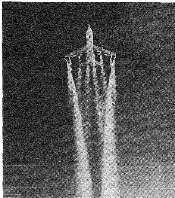
Figure 10.- L-1011 with spoilers deployed for vortex minimization.
