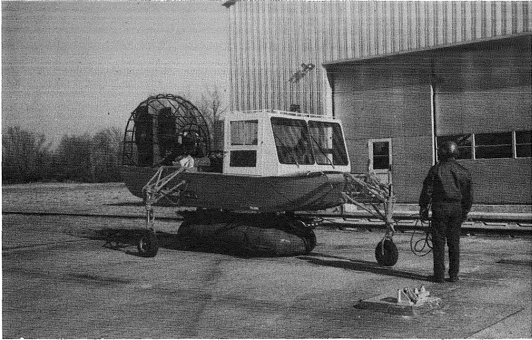
(c) Free-body ground-handling tests: RPV and general ACLS.
